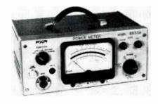
Model B833A uses a dc self-balancing r-f bridge for accuracies of 0.15% @ 10mw or 1.5% @ 1mw. The unit eliminates subtle errors associated with audio power in r-f bridges. Features include: a single zero adjustment; availability of thermistor heads at freqs. from 10Mc to 40gc. It is lightweight and portable with optional rechargeable battery. FXR, 25-15 50th St., Woodside, N. Y.
