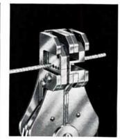
3. Keep squeezing. Simultaneously, colletblade severs insulation without contacting conductor.
