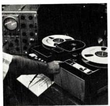
By recording hf signals, then reproducing them in its stop-motion mode, a 75-lb. TV tape recorder makes it practical to study a wide variety of transients without need for loop recorders and readout devices, or related equipment. Technician (above) stops tape on Precision Instrument Co.'s PI-3V recorder to show recorded transient signal.
