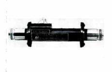
The Model DS 532 solid-state SPST switch handles 1w. It uses conventional Tri-Plate<sup>®</sup> techniques to meet military requirements and has an operating temp. range of  $-54^{\circ}$ C to  $+70^{\circ}$ C. Insertion loss is 3db max. over complete band. In operation, a 22v. potential applied to the control input turns it off; a potential of approx. +3v. @ 80ma turns it on. Sanders Associates, Inc., Microwave Products Dept., 95 Canal St., Nashua, N. H.
