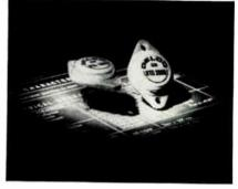
The DTG 1000 and 2000 series are high-power germanium devices. The 1000 series is rated at 15a. and are well suited for video horizontal and vertical deflection circuits. The 2000 series have a 25a. collector current and sustaining voltages from 30 to 120v. Delco Radio Div., General Motors Corp., Kokomo, Ind.
