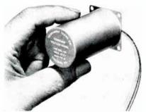
Model MCV-1 measures 2-7/16 in. long x 1-25/64 in. dia. Output voltage regulation is within  $\pm 1\%$  RMS vac, with input voltage fluctations from 95 to 130v. Developed as a substitute for the solid-state voltage reference sources used in compact instrumentation systems, the transformers remain stable over a wide temp. range. Neshaminy Transformer Corp., Furlong, Pa.
