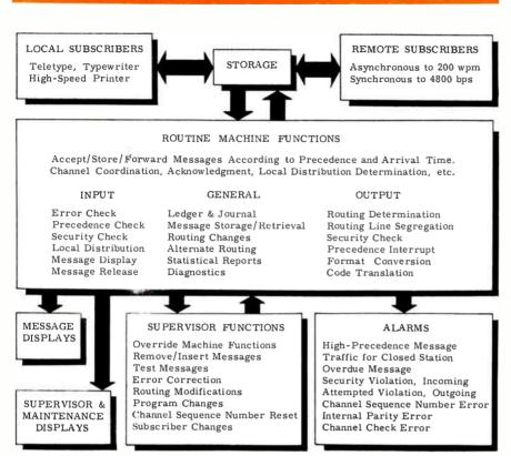
Fig. 6: Functional diagram of the Automatic Message Processing System.
