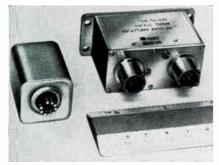
The FA1-A1 provides a ±5vdc (or 10v.) full-scale output from the low mv signals originating from strain-gage type transducers. Continuously adjustable zero balance and gain from 20 to 1000 is available. It contains a highly regulated transducer power supply, reverse polarity protection, input-output isolation and RFI filter. Fairchild Controls, Div. of Fairchild Camera and Instrument Corp., 225 Park Ave., Hicksville, N. Y.
