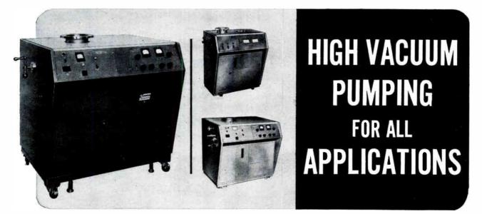
Evacuation to  $5 \ge 10^{-7}$  torr  $\bullet$  Rugged construction guarantees continuous performance under most severe applications  $\bullet$  Available in standard 2, 4 and 6 inch systems  $\bullet$  Kinney liquid nitrogen baffles for maximum conductance with minimum backstreaming  $\bullet$  Compact  $\bullet$  All in one cabinet  $\bullet$  Straight — thru pumping system  $\bullet$  Dependable Kinney Mechanical Pump  $\bullet$  High speed diffusion pump.
