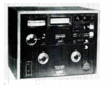
This r-f calibration system, with accessory instruments, has ranges from  $1\mu v$  to 1125v. and 0.5ma to 100a. at freqs. to 1cc. Model RFS-1 high-resolution readout system determines ac-dc differences or freq. influence. It provides readout of true RMS. Model FLH-1 ac-dc voltagetransfer standard has a range of 1.5 to 1125v. with an accuracy of  $\pm 0.01\%$  to 30kc and  $\pm 0.02\%$  to 50kc. Singer Metrics Div., The Singer Co., 915 Pembroke St., Bridgeport, Conn.
