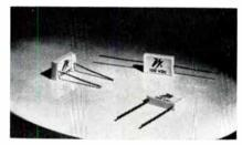
The thin-line series features: capacitance ranging from 0.5pf to 10,000pf; temp. coefficients of 0 ( $\pm 25$  ppm/°C) and 105 ( $\pm 25$  ppm/°C); axial, face radial, or edge radial lead configurations. Insulation resistance is greater than 100,000 megohms; capacitance is stabile over a freq. range from 1kc to 1kc. Vitramon, Inc., Box 544, Bridgeport, Conn.
