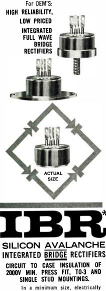
In a minimum size, electrically insulated package, the 1N4436 (250v BV  $_R$  min.) and 1N4437 (450v BV  $_R$  min.) use SAR\* (Silicon Avalanche Rectifier) characteristics to control the avalanche voltage by causing it to occur across the entire junction area.
