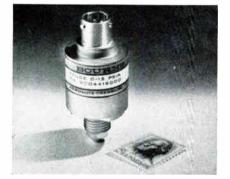
Model 441 operates over pressure ranges of 0-5 to 0-450 psia. Flex-pivot construction virtually eliminates mechanical friction and enables resolution of 0.5%. Other features include ultra-reliable potentiometric elements; hermetic seal construction; and optional LOX-clear compatibility in all pressure ranges. Bourns, Inc., 1200 Columbia Ave., Riverside, Calif. Circle 205 on Inquiry Cord
