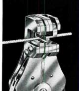
2. Squeeze. Slug gripper moves down to impinge on slug with only slight penetration.
