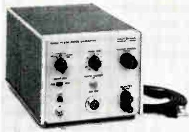
The power meter calibrator shown here is a precision constant-current generator.
