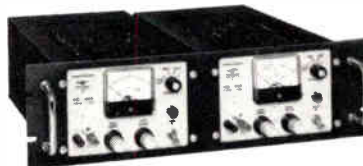
Two Trygon HR20-1.5's, rack-mounted side by side.
