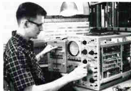
Fig. 1: Simultaneous display (1) of the same pulse train on two display-switched time bases. Brightened portion of lower sweep is displayed on expanded and delayed upper sweep. Signal source is connected to input of a single channel vertical plug-in unit. Photo below shows the 547 oscilloscope in use in the laboratory.
