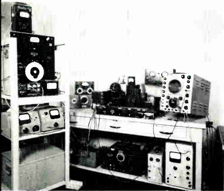
Fig. 2: This equipment comprised an IR detector measurement station in 1953. Detectors to be checked were placed in the metal box (center of picture), which slides along an optical bench to position it in front of the various IR sources.
