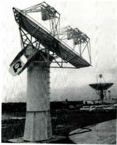
Broadband "Telscom" (Telemetry, Surveillance and Communications) automatic tracking antenna system developed by Radiation, Inc.
