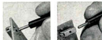
Horizontal Jack accepts tip plug in either end or from top or bottom.
