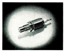
The 5367 subminiature r-f connector has a low-pass filter installed in one end of the connector body. The connector body is of hex design with 0.0001 gold plating. Captivated contacts insure proper engagement of mating parts, Sealectro Corp., 139 Hoyt St., Mamaroneck, N. Y.
