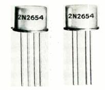
The 2N2654 is a germanium PADT transistor for use in VHF high-gain circuits. It has feedback capacitance of 0.5pf; an output conductance of  $3.5\mu$ mhos at 10.7MC eliminates variations in-stage gain and bandwidth between individual transistors, thus permitting optimum gain. Amperex Electronic Corp., Semiconductor and Receiving Tube Div., 230 Duffy Ave., Hicksville, L. I., N. Y.
