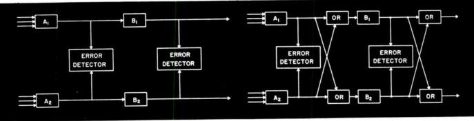
Fig. 6: Duplex logic with error detection. No provision is shown for finding which unit A1 or A2 (or B1 or B2) is faulty. No provision is shown for isolating the faulty unit.
