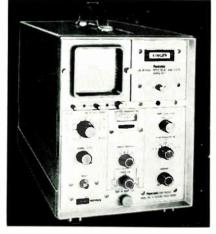
Three plug-in interchangeable modules covering the 20CPS to 25MC range are for use with the portable TA-2 Universal Panoramic spectrum analyzer. Any ac line from 95 to 1000CPS will recharge the unit's nickel cadmium batteries. Singer Metrics, 915 Pembroke St., Bridgeport, Conn. BOOTH 2415.
