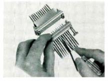
Series 25 miniature rectangular plug and socket connectors and solderless crimp-termination removable contacts conform to Mil-C-22857. The contacts feature an extra-wide, 3-tine tensionspring clutch. Connectors are available in 14, 20, 26, 34, 50, 75 and 104-contact sizes with removable contacts for #14 to 24 AWG wire sizes. Continental Connector Corp., 34-63 56th St., Woodside 77, N. Y. BOOTH 503.
