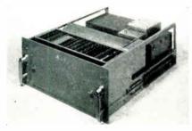
The scan converter of Model 212 Electrostore® recording storage-tube system has a single-gun recording storage tube that performs instantaneous recording and readout of video signals. The wideband deflection system makes it suitable for high-speed deflection patterns. The 30 Mc bandwidth of the input and output video circuitry permits wide-range, high-resolution storage and retrieval. Image Instruments, Inc., 2300 Washington St., Newton 62, Mass.
