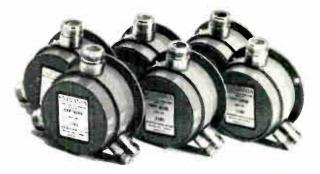
Sylvania meets the need for wideband circulators with a new miniature unit featuring a frequency range of 2 to 4 Gc—the only full-octave completely shielded circulator available today. The SYF-3248 is readily available in sample quantities. Summarized specifications appear below.
