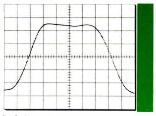
Fig. 5: Depicted here is a small time jitter that occurs during internal triggering of sampling. Pulse is 1v.-1.2nsec.
