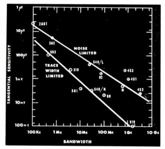
Fig. 1: Graph shows "tangential" sensitivity for some instruments, limited by two causes. The term is borrowed from radar.
