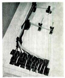
A time-saving method for preforming cable harnessing is accomplished by a few components: harness assembly clips, end clips, junction posts, and end clip brackets. All wires are held in place right through banding, lacing or tying. The harness is then peeled off the board and is ready for installation. Weckesser Co., Inc., 5701 Northwest Hwy., Chicago 46, 111. BOOTH 712.
