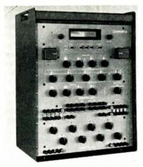
Model 121 direct-reading, double-ratio resistance comparison system is a matched assembly of a resistance bridge, special generator-detector and a lead corrector. It has a comparison accuracy of approx. 1 ppm over a range of  $\pm 6000$  ppm. Electro Scientific Industries Inc., 7524 S.W. Macadam Ave., Portland 19, Ore. BOOTH 2317.
