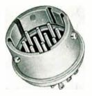
These multi-pin connectors are in the Mil-C-26482 (Class H), Mill-C-5015, and Mil-C-25955 series. They are rated at 5a, with peak voltages at 1000v. All connectors are hermetically sealed and have a leak rate of less than 10<sup>-8</sup> cc of helium as measured at a pressure of one atmosphere. Dage Electric Co., Hurricane Rd., Franklin, Ind. BOOTH 320.
