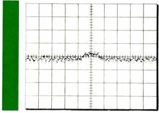
Fig. 2 (above): Sampling technique of "smoothing out" random noise without loss in bandwidth is seen in a typical display for 0.8mv/2.5nsec pulse triggering sampling and timing units.
