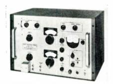
The Model 75C is a 3-terminal directcapacitance bridge. The Wien bridge oscillator, multi-stage tuned detector, and power supply are self-contained. No accessories are needed for normal use. Built-in provision is made for applying dc bias to the specimen under test. The bridge permits investigation of freq. influence on the test. The signal level across the test is continuously variable from a max. of about 3v. to a min. of less than 10mv. Boonton Electronics Corp., Morris Plains, N. J.
