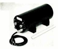
The WJ-269 is completely self-contained, requires only an ac line-voltage input, and is adjustment free. The compact L-band amplifier with its integral power supply weighs less than 17 lbs. Max. noise is 5.5 db from 2.0 to 4.0cc. Small signal gain is 25 db (min.); saturated power output is nominally -5dbm. Watkins-Johnson Co., 3333 Hillview Ave., Stanford Industrial Park, Palo Alto, Calif. BOOTH 4505.
