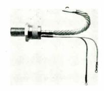
This 3-terminal, 4-layer pnpn 250a. unit has a forward blocking voltage and peak reverse voltage to 700v. The type 221 is used for fast switching high-power inverters. Other uses include motor control, plating supplies, and ignitron replacement. Features: internal construction that eliminates thermal fatigue problems; low thermal impedance; glazed ceramic headers; and hermetically weld-sealed cases. Westingtouse Semiconductor Div., Youngwood, Pa.
