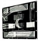
The Wasp patchboard assembly uses point-to-point patch cords for quick program changes, or pre-programmed patchplug modules for semi-permanent installation. If a more positive system is required, grid marking or positions may be imprinted by silk screening. It can be . made as a complete 24 x 24 in. unit panel. Malco Mfg. Co., 4025 W. Lake St., Chicago 24, III. BOOTH 4008.
