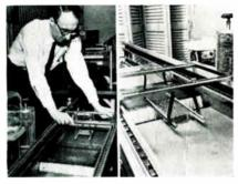
The USWA is an ultrasonically energized wave applicator which allows a straight-line ultrasonic process. The elevated standing wave is 12 in. wide x 12 in. long and is raised  $\frac{3}{4}$  in. above the tank surface. The unit may be used for pickling, bleaching, washing, burnishing and tanning processes. Electrovert Iuc., 240 Madison Ave., New York 16, N. Y. BOOTH 4009.
