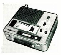
Tracemaster<sup>®</sup> single-channel portable direct-writing recorder, model 29105, has a timer-event marker to correlate time of data with related events. The marker may be used as a timer or remote timer. The unit has a response from dc to 90cPs; is essentially flat at 30mm (P to P amplitude), 3db down at 125cPs. Rise time is approx. 5msec. American Optical, Instrument Div., Buffalo 15, N. Y. BOOTH 4525.
