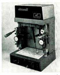
Ultramill is a laboratory tool used for development work in semiconductors and microelectronics. This micro-manipulated machine tool permits direct working from 8½ x 11 in. drawings. Movements traced by a plastic chessman on the drawing are reduced mechanically and transmitted to 2 interchangeable tool housings. The Ultramill machines its own tools. Micro Dynamics Corp., 34118 Pacific Coast Hwy., Dana Point, Calif. BOOTH 4003. Circle 287 on Inquiry Cord
