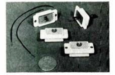
These subminiature connectors have solderless crimp-removable type 22-gauge pin and socket contacts which withstand 25 lb. axial load. The contact rating is 30a. at 280vac and 200vdc. Density is 110 psi. Hughes Aircraft Co., Florence Ave. & Teale St., Culver City, Calif. BOOTH 4240.
