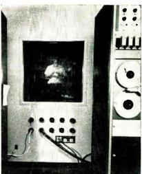
Subject is seen through 1-way glass window in sound-proof isolation chamber at Barrow Neurological Inst., Phoenix, Ariz. Room is room within room with heavy metal inner and outer walls separated by accustical filler. Built by Industrial Acoustics Co., New York, N. Y., room has noise reduction coef. of 0.95. Room is r-f and electrostatically shielded. Environment is exactly controlled.
