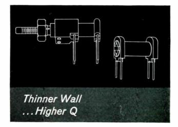
New CAMBION® tunable coil forms for printed circuit applications have a wall thickness of only .010", improving flux coupling and Q because the slug can be closer to the windings. The thin wall is made possible by a unique production technique – forms are molded of high-impact diallyl phthalate for close run-out (TIR) and concentricity control. Design highlights include live leads that double as studs for mounting on .250" x .500" PC grids and mounting lands that eliminate moisture traps.
