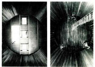
Photos show inside of 41,000 gal. tank at Sparton Electronics' new underwater acoustic laboratory, Jackson, Mich. Tank, 18 ft. in dia. by 20 ft. deep, has special foundation and vibration dampeners to reject external noise, temp. control between 20 and  $25^{\circ}$  C. Firm uses tank to study electro-acoustical devices.
