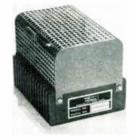
This regulated dc power supply is built with silicon transistors and has a 75°C amb. temp. range. Models are available with output voltages from 6 to 31vdc aud current capacities from 600ma to 1.5a. Input range is from 105-125vdc, 47 to 440cps. Consolidated Avionics Corp., 800 Shames Dr., Westbury, L. I., N. Y. BOOTH 4615.
