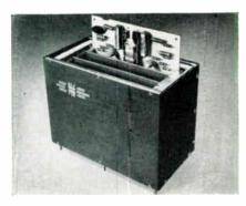
In component oven V1318 standard female printed-wiring board connectors are installed in the base of the oven to receive the boards. Stability over the amb. range is  $\pm 0.5^{\circ}$ C. The amb. range is from 15°C to 30°C, and operating temp. is 75°C ( $\pm 2^\circ$ ). Power requirements vary, depending upon the amb. temp. range, but the preferable operation is 115vac, 50w. Reeves-Hoffman Div. of Dynamics Corp. of America, Cherry & North Sts., Carlisle, Pa.
