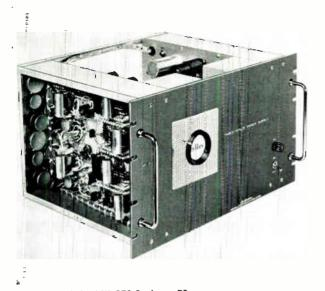
Front view of the MK-150 3 phase, 50 w. power supply. This supply consists of three 15 w. oscillators with an integral oscillator driver mounted on a  $10\frac{1}{2}$  in. rack panel. Delta and wye connections are located at rear panel of the unit.
