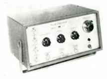
Model 126 uses transistorized circuits and a high-speed coaxially-mounted mercury switch to produce its fast rise times. The fast pulses of calibrated amplitudes make it useful in checking transient response of wide-band systems, fast solidstate switching circuits, computer devices, and nuclear applications. E-H Research Laboratories, Inc., 163 Adeline St., Oakland 20, Calif.
