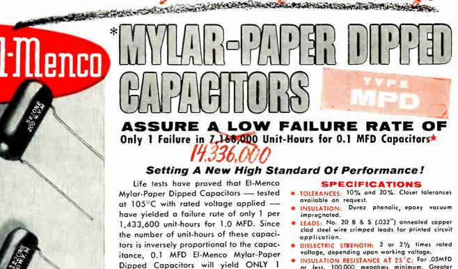
FAILURE IN 14,336,000 UNIT-HOURS.
