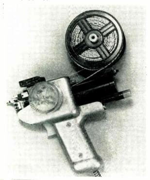
The new method, called Termi-Point<sup>®</sup>, uses striptype terminals to make multiple post-connections to posts of various sizes. These posts need not have the sharp corners, common when using the wrap-type method.
