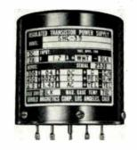
SH series feature input voltages from 12-32vdc ( $\pm 2$ ). Any 3 output voltages may be selected at any combination of amperages up to 60w. They meet the requirements of Mil-E-5272D. Units are encapsulated in thermal-conducting epoxy, permitting relatively transient-free operation from  $-54^{\circ}$ C to  $+71^{\circ}$ C. Within this range, line and load regulation are maintained to  $\pm 0.5\%$ . Arnold Magnetics Corp., 6050 W. Jefferson Blvd., Los Angles 16, Calif.
