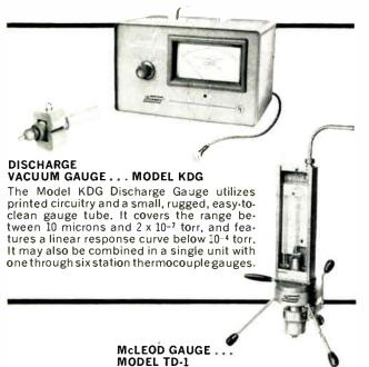
The Model TD-1 McLeod Gauge accurately indicates pressures between 150 torr and one micron, easily and without adjustment. It is light weight, sturdily constructed, and more compact than most comparable gauges and is readily disassembled for cleaning.
