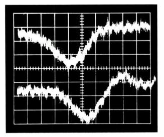
Fig. 7: Double exposure plot of reflectometer resolution. Shown are 0.02pf discontinuities in sequence at points 1 cm. apart on a  $50\Omega$  air line. Sampling is at 50 psec/cm and 1 mv/cm.
