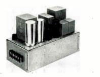
This 2 watt power oscillator has a maximum total harmonic distortion of 0.1%, a frequency stability of 0.1% and amplitude regulation of 0.2%, under all conditions of line and load.
