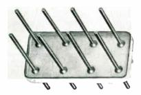
Ceramic-to-metal microminiature relay header has 0.200 in. grid spacing for fullsize or half-size crystal can relay. Highalumina body copper is brazed to terminals and outer metal mounting memher. Header is designed for heliarc welding to crystal can. Clare Ceramics Inc., 15 W. Main St., Cary, III. BOOTH 4309.
