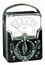
Model 630-PLK has a sensitivity of  $20 \text{K}\Omega/\text{vdc}$  and  $5 \text{K}\Omega/\text{vac}$ . It features  $\pm 3\%$  accuracy on dc and  $\pm 4\%$  on ac. Stray magnetic fields are eliminated by a self-shielding bar-ring movement. It is usable with freqs. through 500 kc. The Triplett Electrical Instrument Co., Bluffton, Ohio. BOOTH 3311.
