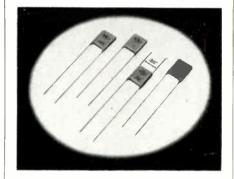
Type DA-790 measures 0.5 in, sq. with thickness ranging from 0.150 to 0.300 in. They combine metal electrodes with lamihated layers of thin-film ceramic. Capacitance values are from 0.022 to  $0.47\mu f$ . Dielectric strength is 450v. for 1 sec. min., and insulation resistance is 150 megohm- $\mu$ f minimum at +25°C. Centralab, The Electronics Div. of Globe-Union Inc., 900 E. Keefe Ave., Milwaukee 1, Wisc.
