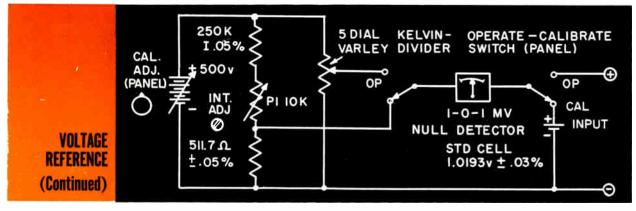
Fig. 1: Accuracy and stability of a Fluke DC differential voltmeter depends on its internal reference seen.
