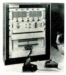
In one second the 19 x 28 x 20 in. unit can perform 36 tests on devices with up to 14 terminals. Plug-in circuit boards for bias, limits, timing, and sorting add to programming simplicity. Programming is accomplished by precision resistors on a plug-in board. Sensing leads from power supplies to the bias program
