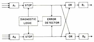
Fig. 9: Diagram at left shows duplex logic with error detection and correction details. Fig. 10: Above diagram shows duplex logic including "ands" to provide two separate computers.
