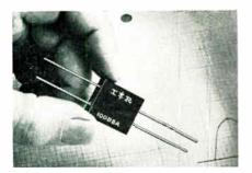
The 10DB Series single-phase fullwave bridges perform the function of 4 individual silicon rectifiers, and measure  $0.830 \times 0.530 \times 0.215$  in. Rated up to 1.8a. dc over a PRV range of 200 to 1000v., these units operate to  $140^{\circ}$ C. International Rectifier Corp., 233 Kansas St., El Segundo, Calif. BOOTH 2304.
