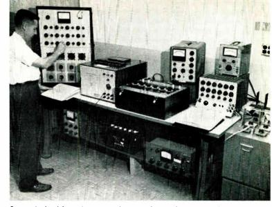
Some of the lab equipment used to accelerate the aging and increase the yield of zener diodes. Methods include power aging, hot-cold temperature cycling, and high current pulsing.
