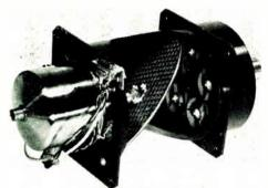
Radiometer for NIMBUS weather satellite
