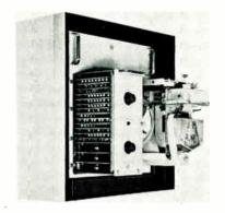
Model 265 solid-state, high-speed serial converter converts parallel digital data to serial form in data-logging applications using tape punches or magnetic-tape recorders. A built-in memory allows it to acquire new information while feeding previously gathered information to the tape punch or recorder. Non-Linear Systems, Inc., Del Mar, Calif. BOOTH 2313. Circle 290 on Inquiry Card
