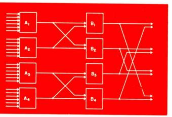
Fig. 5: Quadded logic. Quadruple logic elements are required.
