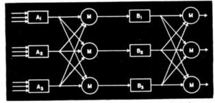
Fig. 3: Majority-vote logic with triplicated voting elements. Component count will vary from 3 1/6 to 3½ times that of a non-redundant computer. Improvement in reliability will generally be better than a factor of 3, however, depending on the number of sections the computer is divided into, reliability of the voting element, mission time and the element MTBF.
