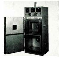
This compact environmental chamber performs the thermal shock portions of Mil-202B, Methods 102A and 107A. It performs between  $-100^{\circ}$ F to  $+300^{\circ}$ F range. The unit can also be supplied for operating in a range of  $-300^{\circ}$ F to  $\pm1000^{\circ}$ F. Operation is completely automatic with cycling timers for each test phase. Interior of the chamber is 16gauge stainless steel with 16-gauge galvanneal exterior. Conrad, Inc., Holland, Mich. BOOTH 1310.
