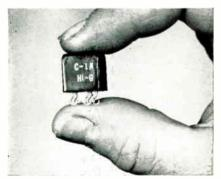
The Dice Cube microminiature relay meets Mil-R-5757 and measures 0.500 x 0.500 x 0.500 in. Dice Cube is a 1pdt, dc relay with a contact rating of 1a. resistive at 32vpc. Hi-G Inc., Bradley Field, Windsor Locks, Conn.
