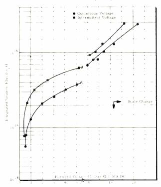
Fig. 3: Results are these plotted curves of diode(s) forward characteristics with and without energization during nuclear exposure.
