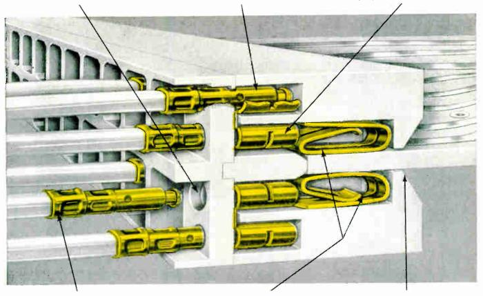
Multiple-contact, crimp-on, snap-in removable wire pins provide widest range of wiring flexibility. Bifurcated "flexing action" contacts provide twin wiping contact surfaces instead of one, assure positive contact. Closed entry card slot on 15 and 22-position sizes protects contacts from oversize probe or PC board.
