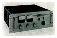
The DCR150-15 is a low-cost, smallsize 2250w, regulated dc power supply. It accepts inputs centered at 208 or 230v. Output can be varied from 0 to 150v. It can be regulated to  $\pm 0.1\%$  +15mv for 0 to 15a, load variation and  $\pm 10\%$  input line variation. Sorensen, a unit of Raythcon Co., Richards Ave., So. Norwalk, Conu. BOOTH 2410.
