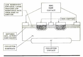
These new devices, types 2N2832, 2N2833 and 2N2834, have a specified fall time of 0.7  $\mu$ sec at 8 a. of collector current in TV flyback circuits and will operate at 83% efficiency in 15 KC power inverter circuits.
