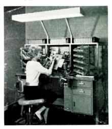
Videosonic<sup>TM</sup> systems cut training time and increase efficiency of assemblies. The systems use colored slides and tape-recorded instructions which allow individual instruction to each person. Thus, the retention of instructions is higher than by conventional training methods. Hughes Aircraft Co., P.O. Box 3310, Fullerton. Calif. BOOTH 1204.
