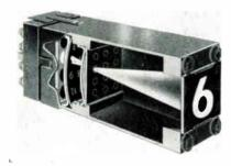
Series 120 and 220 uses a new lens to double the brightness of readouts and cue indicator switches. This lens increases the brilliance of 6v. unit, type 328, to 50 ft.-lamberts. Normal lifetime is 500 hrs. Reducing operating voltage to 5v. extends lamp life to 5000 hrs. Up to 50,-000 hrs. at 17 ft.-lamberts (using the lens) can be obtained by operating the 6v. type 349 lamp at 5v. Industrial Electronic Engineers, Inc., 5528 Vineland Ave., N. Hollywood, Calif. BOOTH 4531.
