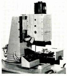
The Model U-1065 Sequential Numbering Machine also prints value and date code directly on electronic components. Offset printing with metal type allows changing any part of the print, including resetting the automatic numbering unit, in seconds. Markem Super Kemgo Ink makes serial numbering possible as all the ink on the offset pad is transferred to the components. Markem Machine Co., Keene, N. H.
