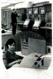
Three computers—a Honeywell 290 digital computer (inset) and 2 231R analog computers built by Electronic Assoc., Inc., will be used to simulate operation and control of complex industrial processes at Minneapolis-Honeywell's Pottstown. Pa., computer center. Honeywell will also rent center to industry and government for industrial control tests.
