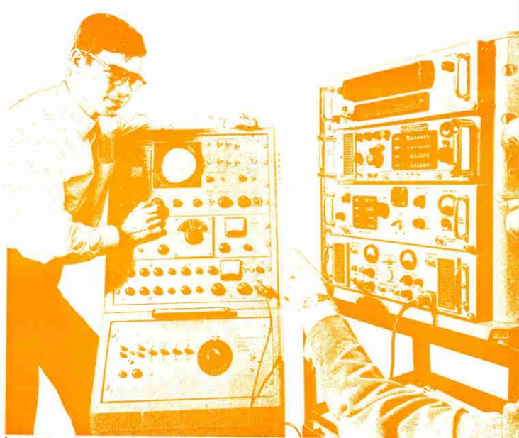
Panoramic MODEL SSB-3b SPECTRUM ANALYZER SHOWN WITH RANGE EXTENDING CONVERTER, MODEL REC-1 (LOWER PANEL).
