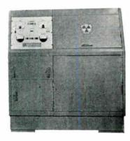
If you have to leak-check thousands of components every day, this is your answer: CEC's radiation-sensing 24-510A Radiflo Leak Detector. It's the only leak detector economically feasible for 100% checkout of mass-produced components such as transistors, diodes, and relays because it finds leaks of 1x 10<sup>-5</sup> to 1x 10<sup>-11</sup> atm cc/sec and permits checking at rates up to 2500 components per hour.
