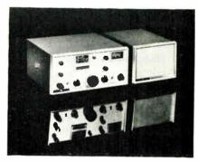
The NCX-3 has a r-f power input of 200w SSB PEP, 180w CW and 100w AM. R-F power output is 120w SSB PEP, 108w CW and 30w AM. Frequentiability is 400crs long-term after warmup. Suppression carrier —50db: unwanted sideband —40db. Receiver sensitivity is 1.0μν for 10db S/N ratio. Selectivity is 2.5kc at 6db. Receiver audio output is better than 2w; 3.2Ω. The NCX-3 measures 6 x 135% x 115% inches and shipping weight is 20 lbs. National Radio Co., Inc., 37 Washington St., Melrose 76, Mass.
