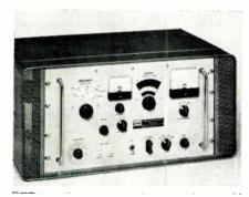
Measures bandwidth, sensitivity, and distortion of FM telemetry receivers in the 225 to 800mc range. AMI Model 303 FM, features a carrier freq. tunable from 225 to 800mc in 2 bands with freq. stability of ±0.005% and calibration accuracy of ±0.5% receivers. Three FM deviation ranges are: 0-30, 0-100, and 0-300kc, with ±5% FSD on all ranges from 225 to 400mc, and ±10% FSD from 400 to 800mc. Advanced Measurement Instruments, Inc., 109 Dover St., Somerville 44, Mass.
