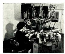
No. 116 features labor-saving devices to reduce handling costs from 66 to 75%. Such operations as taping the start lead, taping or waxing the finished coil, cutting the wire, ejecting the coil and sorting 2 different coils are all automatic on the No. 116. All the operator has to do is load the coil and attach the wire. The Automatic Bachi Bobbin Winder is manufactured with 6, 8, 10, or 12 individually operated winding heads. Leesona Corp., 333 Strawberry Field Rd., Warwick, R. 1.
