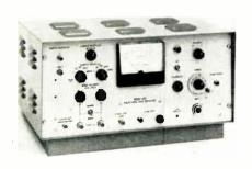
Useful in the microwave area for measuring the gain of pulsed tubes and the power levels in pulsed r-f systems. Model 405 is also useful in metering pulse droop in microwave systems or absolute pulse levels in digital systems. Instrument is furnished with a flat crystal detector which monitors the r-f power by means of its detected output. The sampling time is set by means of a variable sampling delay circuit. Wiltron Co., 717 Loma Verde Ave., Palo Alto, Calif.
