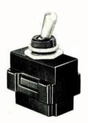
For use in electronic apparatus, test instruments, and communication. The Bulletin 7516 and 7517 feature plug-in terminals, for rapid connection by merely inserting the wire into switch body. Other standard features include: I hole insulated mounting with nylon threaded bushing; bussing connection; and semi-dusttight construction. Rated 3 and 5a at 250v, and 6 and 10a at 125v. Cutler-Hammer. 315 N. 12th St., Milwaukee I, Wisc.
