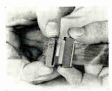
Developed for sizes of cable in accordance with the IPC standard, this connector allows 19 connections to be made in 19 sec. This connector has been designed specifically for use with flat flexible cable. The TAPECON connector has designs for use in applications for tape-to-wire, tape-to-tape, tape-to-miniature round (Mil-C-20482) connector, and tape-to-printed circuit board. Contact in the connector is accomplished through insulation "milling." Burndy Corp., Norwalk, Conn.
