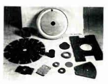
Micaceram retains its properties in applications where temperatures go as high as 1800° F. One of its outstanding features is the ease of machining this material. It is either purchased in a slab and machined by the customer, or M.D.I. will machine it. The material is then purchased in its final form and no firing is necessary after machining. It has a low loss factor and is non-out gassing. Molecular Dielectrics, Inc., 101 Clifton Blvd., Clifton, N. J.
