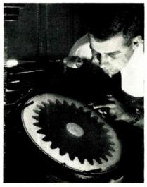
Nylon gear of planetary gear system magnified 20 times. System used in motor-driven type Volt-Pac variable transformers.
