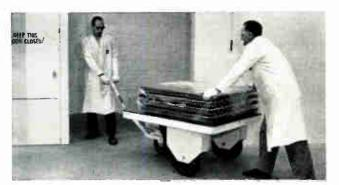
Every precaution is taken to protect the surface. Before leaving the "white rooms" for the laminating presses, copperclad loads are covered with plastic film to prevent dust or other foreign matter from contaminating the surfaces of the material.
