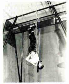
Ceiling walker shows how new Westinghouse magnet combining advantages of permanent and electromagnet works. It can be turned on and off, allowing steps to be taken. Magnet has a "memory," exerting pull in same direction until reversed. Ceramic magnet is between 2 soft steel layers. Electrical connection at one pole causes flux transfer, reversing polarity. Shoe's pull is 30-50 lbs.
