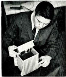
Univac Microtronic Aerospace Computer, occupying .15 cu. ft., is checked by project engineer Ted Sammis. 17-lb. computer of magnetic thin films and semiconductor integrated circuits which has expandable 74.000-bit memory.
