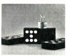
The ZJ265 is for use where the max, divice temp, can be kept below 100°C. Applications include relay replacement; motor speed controls for hand teels; and appliance controls. For automatic assembly in large volume, the silicon controlled rectifier is in the popular cup-type package which can either be pressed, soldered or clipped onto a suitable heatsink. A stud mounted version will also be available (ZJ226). General Electric Co, Rectifier Components Div., W. Genesee St., Auburn, N. Y.
