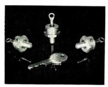
The family is the 1N3208 to 1N3211 series and has a basic current rating averaging 15a over a temp, range of -65° to +150°C. The rectifiers maintain full rated reverse voltage to +175°C which extends through the forward current derating range of +150° to +175°C. Max. peak reverse voltage ratings available from 50v to 300v. Dimensions are 1.6 in. max. overall height, stud length is 0.44 in. and hex size is 0.6875 in. across flats. Delco Radio Div., General Motors Corp., Kokomo, Ind.
