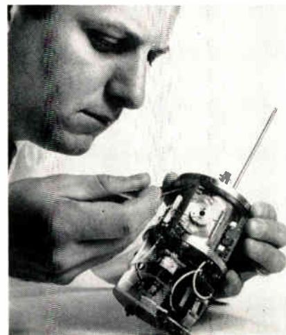
Three-axis, cryogenic accelerometer developed by Minneapolis-Honeywell has been successfully operated at a temperature of about 5°K. Company says it could be used with any high accuracy inertial navigation system. Transformers in the instrument help generate current which create a magnetic field to support a superconducting spherical mass in a frictionless bearing. Mass is found in the upper portion of the unit.
