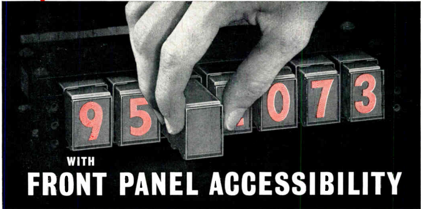
Series 220000 miniature readout can be installed individually or in a 230000 assembly.
