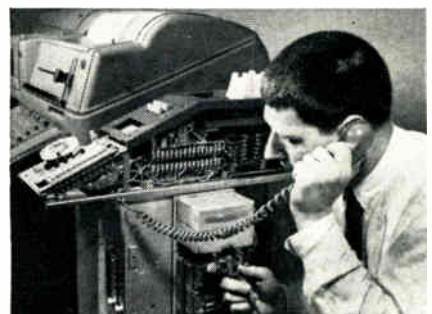
New York Laboratory, N. Y. We were studying the performance of a new data set which converts teletypewriter pulses into tones for transmission over regular voice circuits. Transmitting teletypewriter messages over voice circuits was introduced on August 31, 1962.
