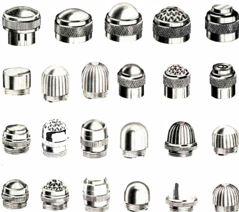
Typical selection of lens caps for indicator lights. Glass types recommended for use with the larger miniature and large lamps because of the heat they generate. Plastic caps used with most miniature, and all neon glow, lamped indicators. Reading l-r, top row: friction mounting, convex glass; screw-on, convex glass; screw-on, plastic dome; screw-on, faceted glass; and screw-on, flat plastic. 2nd row: screw-in, cylindrical plastic; screw-in, long stovepipe, 'halo' effect plastic; screw-in, long stovepipe, fluted plastic; friction, convex glass; friction, faceted glass; friction, flat plastic. 3rd row: screw-in, flat plastic; screw-in, faceted glass; screw-in, convex glass; screw-in, long stovepipe, plain plastic; screw-in, stovepipe, fluted glass; screw-in, short stovepipe, 'halo' effect plastic. Row 4: screw-in, convex glass; screw-in, faceted glass; screw-in, flat plastic; screw-in, short stovepipe, plain plastic; screw-in, stovepipe, plain glass; and screw-in, short stovepipe, fluted plastic.
