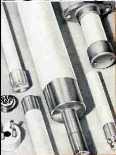
High temperature metallized miniature ceramics with O.D. .0815 \pm .003 with two holes .017 \pm .0015 , thickness .016 \pm .002 are supplied with gold or other finishes.
