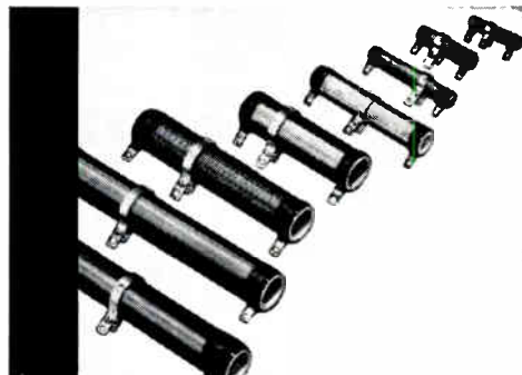
MIL-R-19365C (ADJUSTABLE): Vitreous enameled, wire-wound; all 8 MIL sizes from 11 to 210 watts, 1 to 15,000 ohms.
