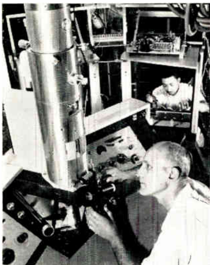
Machinist at RCA's Camden, N. J., plant puts finishing touches on the company's 1,000th Electron Microscope. The microscope enables researchers to see and photograph objects 1 million times thinner than a human hair.
