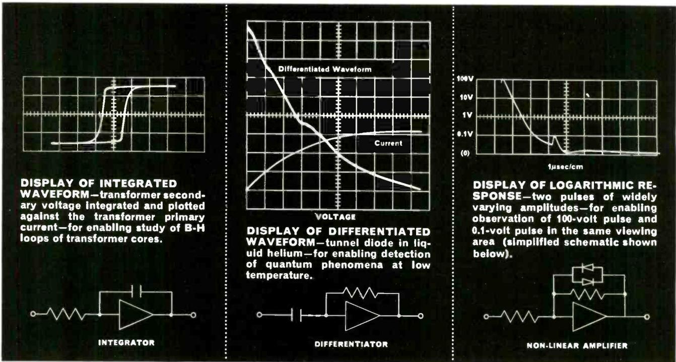
**DISPLAY OF INTEGRATED WAVEFORM**—transformer secondary voltage integrated and plotted against the transformer primary current—for enabling study of B-H loops of transformer cores.
