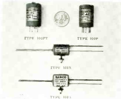
Type 100 line has a noise level of 3 to 10 $\mu$ v at 1K impedance and a noise level of 20 to 150 $\mu$ v at 10K impedance. The drift as well as dc offset is in the low  $\mu$ v range from -65° to +125°C. For shielding, these units are potted in a steel casement containing a transformer and (when required) a phase shift network to provide up to a 50° phase lag. These 400CPS units need only a 6v sine or square wave drive. RAWCO Instruments, Inc., P.O. Box 7393, Ft. Worth 11, Tex.
