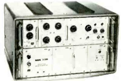
It offers twin-pulse capability as a standard feature. Can be switched in wherever desirable to generate 2 pulses on a common time basis, each pulse having the same width, polarity, and amplitude. Basic instrument specs.: 0 to 10,000 $\mu$ sec. delays; 0.05 to 10,000 $\mu$ sec. widths;  $\pm 50$ v into 50 $\Omega$ ; and better than 15nsec. rise time. Standard modules plug into both front and rear of the rack frames. Servo Corp. of America, 111 New South Rd., Hicksville, N. Y.
