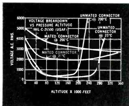
High altitude air has low dielectric strength. By maintaining an air-tight seal 48 Series Connectors enjoy extremely high voltage safety factors.
