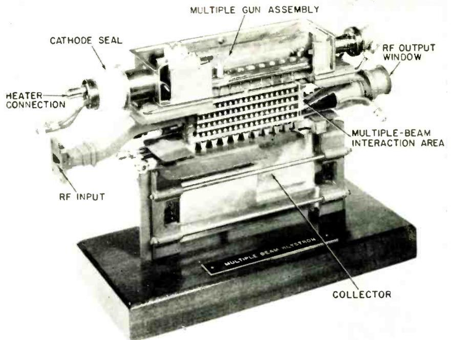
Fig. 7: Modular concept is apparent in this cut-away view of a typical ten-beam multiple-beam klystron which operates at 8.35 GC.
