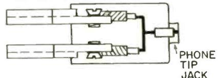
Modification of video plug permits observing waveforms of the video signal.
