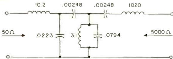
2. Construct a filter with the same characteristics as in problem 1, except that  $R_{in} = R_{out} = 50$  ohms. Using the constant-K values which were calculated for problem 1, it is seen that  $L_{2k}$  and  $C_{2k}$  are very unsatisfactory if one is to get high  $Q$  and small size. A convenient solution is to transform the section by substituting  $\theta = 10$  into Fig. 7. Fig. 21 is thus obtained.
