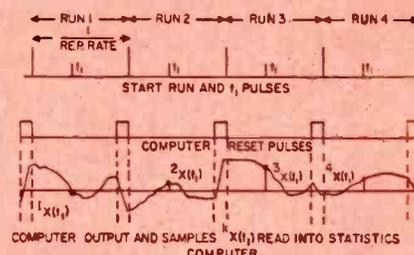
Fig. 1: ASTRAC system operation for random-process studies. Right is block diagram and left illustrates the pulses.
