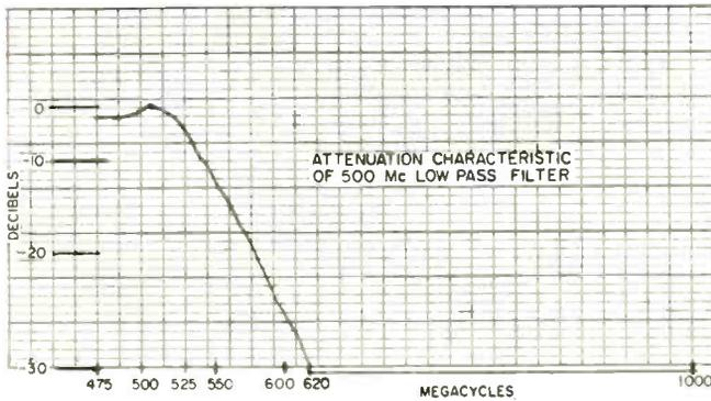
Fig. 3: Typical attenuation characteristic reading obtained with automatic plot system.
