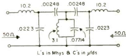
Here, all the coils and capacitors are of reasonably small size, and of values to give good  $Q$ s at 10 kc.
