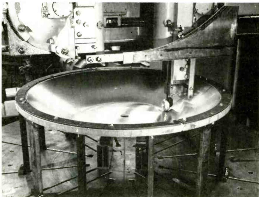
Template serves as a contour guide on a large vertical boring mill to form 6061 Series sheet aluminum to the desired parabolic contour.
