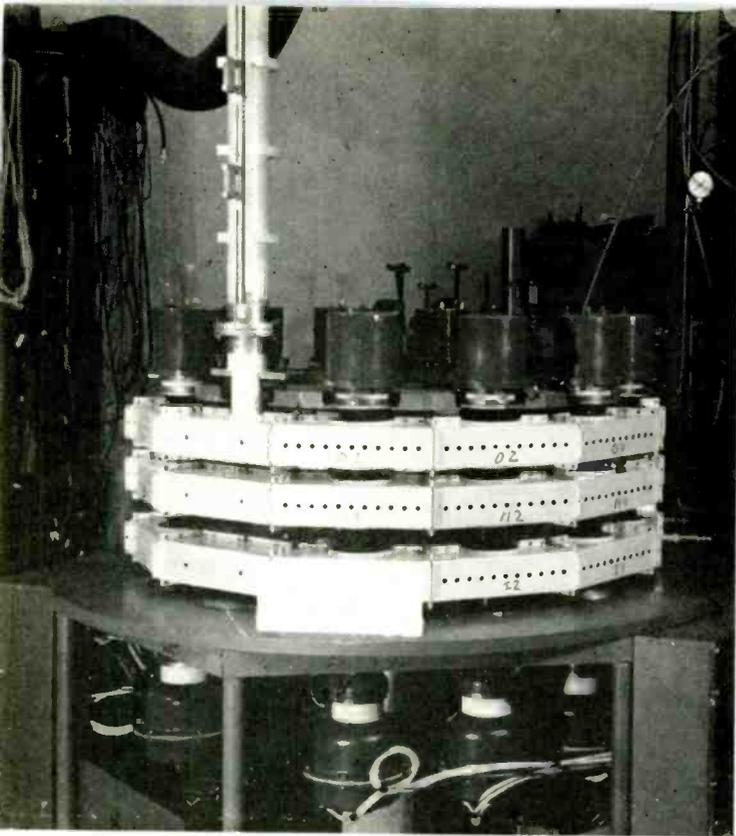
Fig. 4: The ten-beam model was arranged and tuned in the same manner as the four-beam tube, except the circuit was horseshoe-shaped. The ten-beam amplifier is shown here without the magnetic field.
