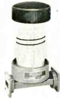
These Direct Reading Frequency Meters give broadband measurement over the full waveguide freq. range to a high degree of accuracy, without the need for interpolation or charts. The direct reading feature makes these freq. meters ideal for use in both laboratory and production testing. The long effective scale length gives max. readability, resolution and accuracy. Overall accuracy ranges from 0.07% for the 398-DR to 0.12% for the 1098-DR. Waveline Inc., Caldwell, N. J.
