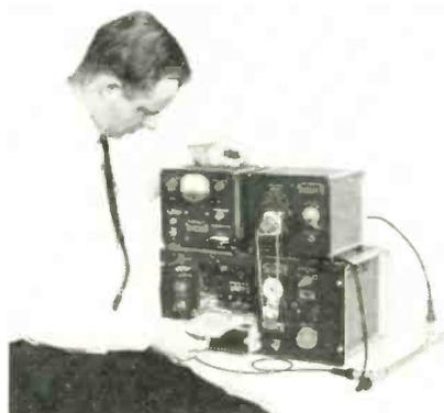
Fig. 2: Amplitude regulating power supply, uhf oscillator and graphic level recorder used to plot frequency response characteristics of filters and other networks at high frequencies.
