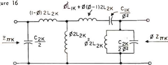
Again note that  $\theta$  has to be less than 1 (a true step-down) for  $(1-\theta)2L_{2K}$  to be a positive inductance.
