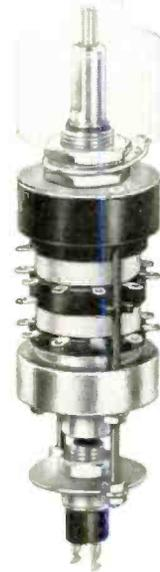
One unit incorporates a 2 deck, 4 pole, #36 Series Concentric Shaft Switch, #24 Series Spring Return feature, and Push-Pull Switch operated by 1/8" shaft.
