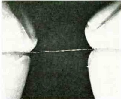
This microdiameter wire is drawn from high permeability Co-Netic AA alloy. Diameter is  $5.0 \times 10^{-4}$  inches (0.25 circular mills). The wire displays magnetic properties and is offered for experimental investigation as to applications. It is available from stock. Magnetic Shield Div., Perfection Mica Co., 1322 No. Elston Ave., Chicago 22, Ill.
