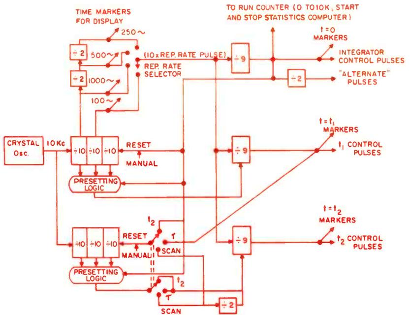
Fig. 4: Simplified functional block diagram of the digital control unit.
