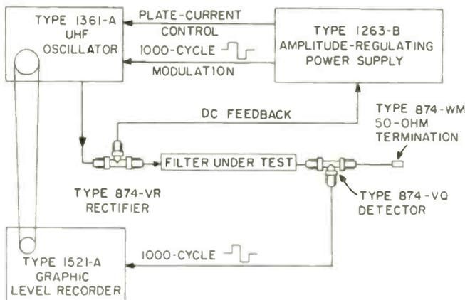
Fig. 1: Block diagram of automatic plotting set up.
