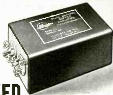
These high-performance units are designed to drive Kearfott's Size 11 R980 winding-compensated synchro resolvers. The amplifier-resolver combination has stable gain characteristics and negligible phase shift through an ambient temperature range of  $-50^{\circ}\text{C}$  to  $+85^{\circ}\text{C}$ . Extremely high resistance to shock and vibration. Meet environmental requirement of MIL-E-5272.
