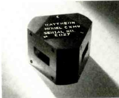
The CMX9 handles up to 2kw peak and 20w average power, and can be supplied for operation at more than 100kw peak power. It has 20db min. isolation with a 0.3db max. insertion loss; VSWR 1.30 max. A three-port wye circulator made of aluminum, it is approximately 2½ in. in dia. and 1½ in. high. It mates with UG135/U flange and 1½ waveguide. The CMX9 can be used in parametric amplifier applications. Microwave & Power Tube Div., Raytheon Co., Foundry Ave., Waltham 54, Mass.
