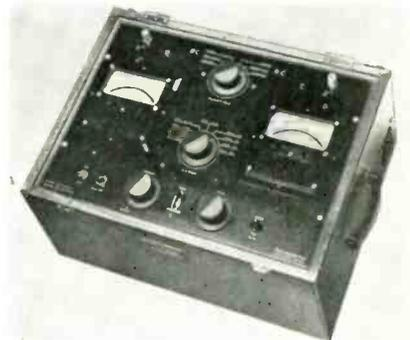
This portable Meter Calibrator supplies accurately metered ac and dc voltage and current for calibration of all kinds of panel and laboratory meters without loading errors. The 54 full-scale ranges cover 20 $\mu$ a to 10adc, 2v to 1000vdc, 20ma to 10a ac and 2mv to 1000vac. AC ranges are compensated and calibrated for 60 and 400 cps; dc supplies are filtered to 0.5% or better. The controls of this instrument are fully interlocked for safety. Twinco Inc., 10 Cheney St., Boston 21, Mass.
