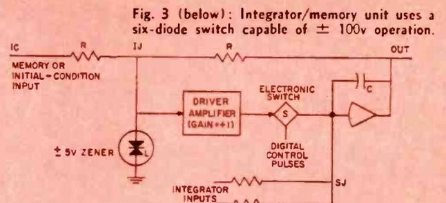
Fig. 3 (below): Integrator/memory unit uses a six-diode switch capable of  $\pm 100$ v operation.
