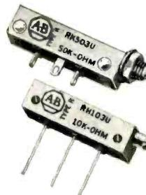
Type R adjustable fixed resistors allow stepless adjustment. Moving element is self-locking for absolutely stable settings. Watertight case permits encapsulation. For continuous use from  $-55^{\circ}\text{C}$  to  $+125^{\circ}\text{C}$ , rated 0.25 watt at  $+70^{\circ}\text{C}$ .
