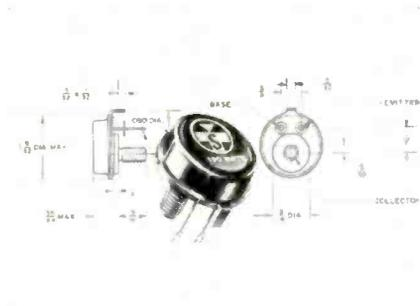
These silicon transistors, Types 2N1015C, 2N1015D, 2N1016C and 2N1016D are diffused junction, npn high power devices. They are 150w, single-end stud types with collector-emitter voltages of 150v for the "C" types and 200v for the "D" types. The 2N1015C and 2N1015D have a saturation resistance of 0.75Ω; the 2N1016C and 2N1016D have saturation resistance of 0.5Ω. Silicon Transistor Corp., Carle Place, N. Y.
