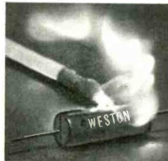
A hot resistor can be trouble. But even at 150°C, Weston Vamistors are the most stable metal film resistors produced. Weston's unique process for internally deposited film protects against contamination and physical shock. Test results to date under MIL-R-10509D show a reliability probability of: 98.78% for temperature coefficient (-55°C); 98.99% for temperature coefficient (+165°C); 99.99% for short-time overload; 99.48% for moisture cycle; and 99.28% for load life.
