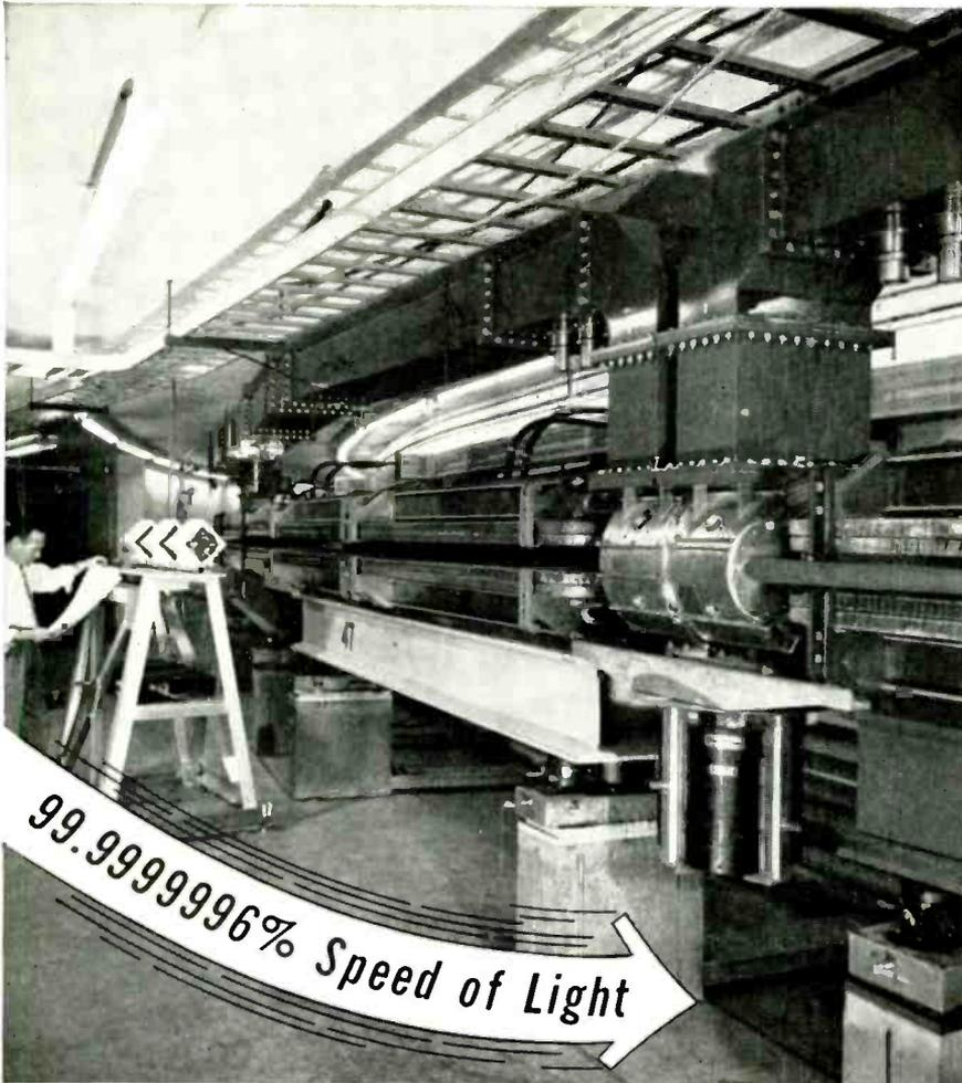
This Cambridge Accelerator is built to deliver about  $6 \times 10^{12}$  electrons per second at 6 Bev—to provide M.I.T. and Harvard physicists with the highest energy electrons and photons ever available within a research laboratory.
