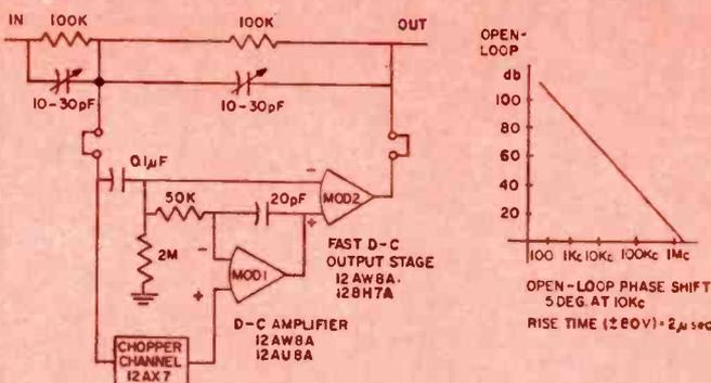
Fig. 2 (left): ASTRAC dc amplifier and phase-inverter network, chopper-stabilized.
