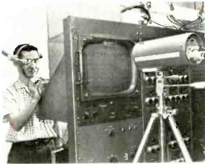
Electrocular TV device, used to speed work in industry is demonstrated by Hughes Co. engineer R. Kiyon. Adjustments are being made on rear of panel, while viewing results furnished to Electrocular unit by closed-circuit TV camera trained on screen on front of panel. Camera may be located in any area to give information necessary to accomplish task. Display was developed and is manufactured by Hughes Aircraft Co., Fullerton, Calif.
