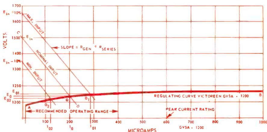
Fig. 8: The operating curve for a regulator tube with load line (C - D) is shown.
