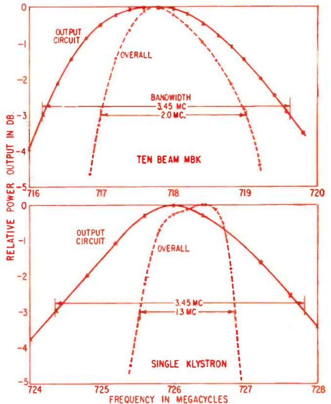
Fig. 6: Ten-beam MBK bandwidth compared with that of a single beam.
