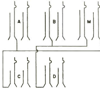
Wiring diagram for the patch cord tester. An ohmmeter is connected at "M."
