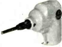
A variation of G-D's standard line of "Wire-Wrap" portable tools, Model 14R2 may be used in remote locations where air or electric power are unavailable or awkward to supply. A permanent magnet electric motor drives this compact tool and is powered by a 2.3a hr. rechargeable nickel-cadmium battery with a built-in charger. It may be equipped for wrapping all wire sizes between 22 and 32 gauge. Gardner-Denver Co., Gardner Expressway, Quincy, Ill.
