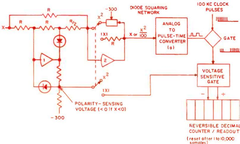
Fig. 5: Digital voltmeter and averaging circuit. A simple pulse-width modulated converter gates clock pulses into a reversible counter for 1 to 10,000 samples.
