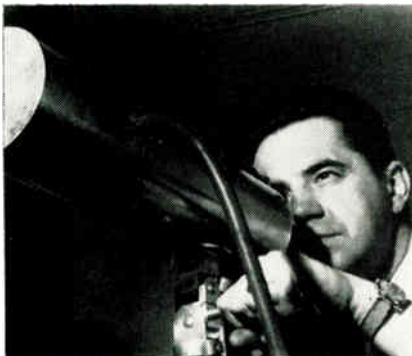
"Laser" is discharged at a rate of 10 bursts a sec. by J. P. Chernoch of G.E.'s engineering lab. It is believed the first time that a Laser beam has been pulsed rapidly and at high power. It's for an optical radar system.
