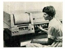
Infrared grating spectrophotometer scans complete wavelength range from 1 to 25 microns and permits continuous recording of spectra without change of components. Model 125 instrument was developed by Perkin-Elmer Corporation's West German affiliate, Bodenseewerk Perkin-Elmer & Co. G.m.b.H.
