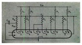
Fig. 6: Circuit used to skip pairs of counts (5 & 6), and to reset to a particular section (3). Target resistors may be desirable in skipped sections as is explained in the text in step number 22.
