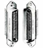
Ribbon rack and panel connectors have diallyl phthalate dielectrics, a material noted for its dimensional stability and high insulation resistance under high temperature and high humidity conditions. For the engineer who must crowd rack and panel connectors into tiny spaces, the Micro Ribbon is probably the answer.
