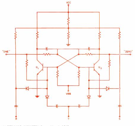
Fig. 1: Schematic of a typical transistor flip-flop suitable for use in counting circuits.
