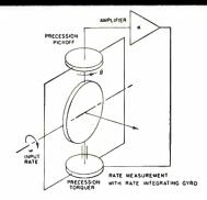
Floated Rate Integrating Gyros. Floated Rate Integrating Gyros are used where exceptionally high-level performance is required. Should the rotor mass of a gyro wheel having an angular momentum of  $1.0 \times 10^{\circ}$  gm. cm. <sup>2</sup>/sec. shift by as little as one micro-inch, a drift of  $0.1^{\circ}$ /hr. could result. The difficulty in achieving ultra-high precision and accuracy is apparent, and the necessity for obtaining low drift gyros is of paramount importance.
