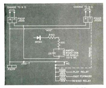
Relays added to "stop" circuit increases flexibility.
