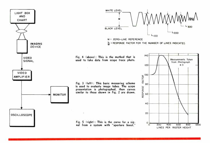
various positions on the chart. Each of these line-groups consists of a wide black and white bar to represent 100% modulation (zero lines) followed by ten groups of four black and three white lines which represent 100 to 1000 TV lines in 100 line increments. This chart, which is available in varying degrees of contrast, makes it possible with one scope presentation (see Fig. 2) to obtain data for a complete square wave response curve.
