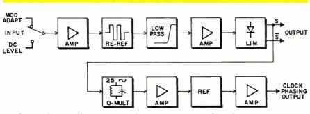
Fig. 5: The preamble is recognized by storing energy in a 25 cycle resonant circuit.
