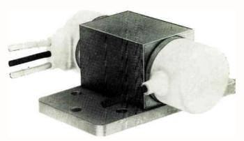
Fig. 3: This rugged, all metal and ceramic reflex klystron is fixed-tuned at 4300 MC  $\pm$  50 MC; provides 1 watt, 100 MC bandwidth.
