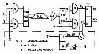
Fig. 28: Logical information delayed and clocked by phase reversal.
