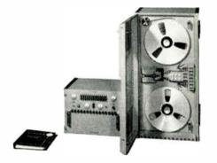
MINCOM'S NEW CMP-100 is the first mobile field recorder/reproducer with wideband and predetection performance. Like Mincom's standard-rack CM-100, the new Series CMP records up to 1.2 mc on seven tracks at 120 ips — with the positive accuracy possible only with longitudinal recording on fixed heads. Its two major components can be placed in an over/under configuration, side by side, or separated; it is easily fitted into many airborne, ship-
