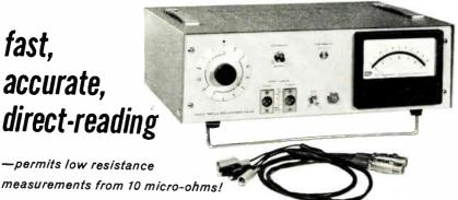
Accurate low resistance measurements can now be read directly with a maximum sample dissipation of only 10 microwatts. Exceptionally stable, the Keithley Model 503 requires no balancing-as encountered in Kelvin Bridges and is designed for rapid measurements. The line-operated 503 supplies an output voltage usable either for chart recording or control functions.
