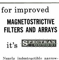
band-pass filters, centered from 20 kc/s to 425 kc/s, are available in bandwidths from 1 cps to 170 cps. Operable from well below  $-100^{\circ}$ C to  $+85^{\circ}$ C, these filters have very low temperature coefficients, as low as 1 ppm/°C in certain ranges. In filter arrays, the differential temperature coefficient is substantially zero. Skirt slopes are 6 or 12 db per band-width octave.
