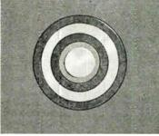
The silicon oxide is thermally grown during the planar diffusion process. It forms a passivated surface over the junction that pravides maximum protection against contamination and degradation of characteristics during the entire life of the transistor. The thin epitaxial layer on low resistivity substrate gives negligible body drop resulting in extremely low saturation resistance and increased uniformity from unit to unit.
