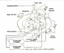
Stable Platforms. Essentially a cluster of gyros mounted within gimbals and utilizing acceleration sensing components, stable platforms perform the important function of having the gyro out-puts control the gimbals by means of a servo loop. By manipulating various arrangements of gimbals and gyros, a variety of platform types can be produced. They are used as reference elements and to stabilize accelerometers, star trackers, and similar devices in space.
