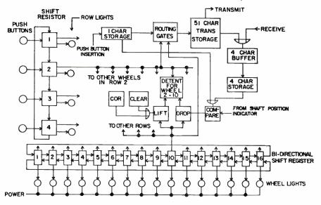
Fig. 14: Wheel selection for message composition is controlled by circuits shown.
