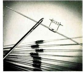
Although 3000 to 4000 of these microminiature units fit in a cubic inch, power dissipation needs would limit it to much less.
