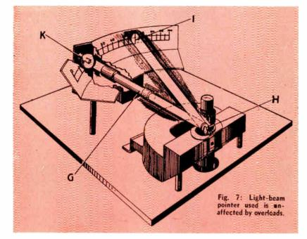
the building of voltmeters with very high resistance values to make them suitable in work where high accuracy, combined with very small current drain from the measured voltage source, is important. Voltmeters with resistance of 1 megohm/v up to 5 megohm/v can easily be built. The only limitation in some cases is the high cost of precision wire-wound resistors when high accuracy and stability are required.
