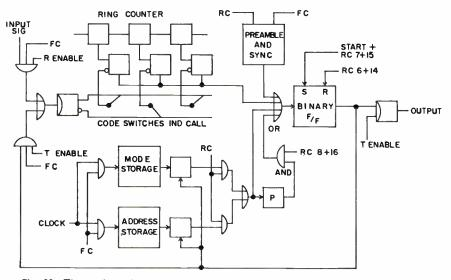
Fig. 13: The marks and spaces are read from ring counter through binary flip-flops.
