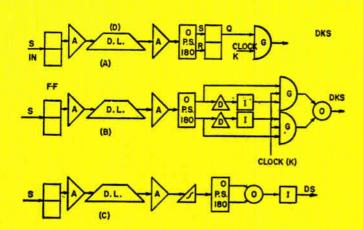
Fig. 25 (left): Three methods of recirculating information by NRZ techniques.
