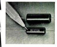
Only Weston missile-line Vamistors give double rating in the same physical size of an ordinary metal film resistor. Why? Because the convection cooling action of inert gas within the Vamistor, together with its internally deposited metal film, dissipates heat at a faster rate.
