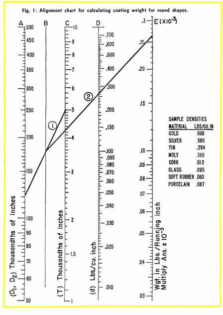
ceiving tubes. From the same principles we later developed the general nomograph shown as Fig. 1. which can be used for any coated round material.
