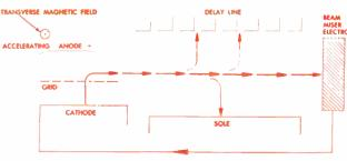
Fig. 1: Schematic of the beam miser indicates function in a standard beam - type tube. was able (under normal operating conditions) to intercept as much as 40% of the total beam current. Return of the intercepted beam current to the cathode (for a given power supply anode current) effectively increased the *total* beam current.
