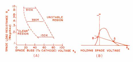
Fig. 2: The spade characteristics are used in the first step for designing circuitry.
