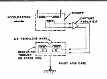
Inertial Accelerometers. A typical force balance pendulous accelerometer utilizing a differential transformer pickoff, a high gain capture amplifier, and a DC permanent magnet force coil is illustrated. This type of accelerometer, together with its amplifier, is a high-gain null-seeking servo in which the current flowing through the force balance coil, measured as voltage across a resistor in series with the coil, is directly proportional to the acceleration applied.
