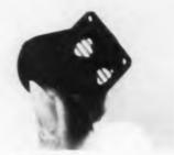
The in sealed miniature magnetic latch-in device has a disc type flag, which may be color coded or imprinted to designate the function being monitored. When energized, it rotates to the "on" position and is held there magnetically even if the energizing source is removed. The device maintains positive indication even when unenergized under vibration from 10 to 500 crs at 10G. Minneapolis-Honeywell, Precision Meter Div., Grenier Field, Manchester, N. H. Circle 308 on Inquiry Card
