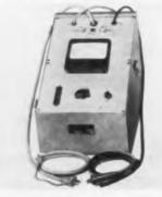
Twenty-two models available with output voltages from 0-1500 v. to 0-10 Kvac, suitable for testing to ASTM, NEMA and UL specs. All models furnished with 5 ft. long input cord, 5 ft. high voltage output leads with clips, continuously variable voltage control, breakdown indicator and adjustable leakage indicator. All units feature completely dead front construction for max. personnel safety. Davenport Mfg. Div., Duncan Elec-tric Co., Inc., Dept. ES2, 2530 N. Elston Ave., Chicago 47, Ill.
