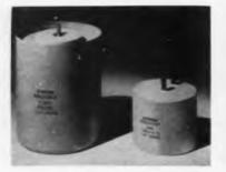
HI-PAK® Capacitors provide rapid discharge of stored energy with noglgible power loss. "Cartwheel" construction minimizes self-inductance and reduces series resistance to low value. A complete discharge can be made in as little as 0.1 µsec. Uses include nuclear systems; explosive initiating circuits; low impedance pulsers; and plasma research. Available in economical polyester-wrap, resinfilled containers. Dearborn Electronic Laboratories, Inc. P. O. Box 3431, Crlando, Fla.
