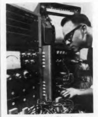
Minutes equal months on this analog computer used by Minneapolis-Honeywell temperature engineers to duplicate climate and building conditions anywhere in the world. Research engineer Donald Nelson can obtain in 15 minutes technical data that would normally take years to assemble. It is used to evaluate performance capabilities of new temperature controls.
