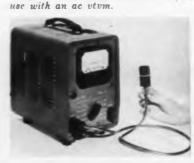
Each unit is individually calibrated in a known field, RMS voltage output is noted as a function of gauss level and is legibly printed on connector shield. Probe consists of an air core inductor, epoxy cast, within an electrostatic shield enclosure. Terminals from inductor are brought out in a pair of electrostatically shielded cables, the other end terminated with standard  $\frac{3}{4}$  in. center banana plugs. Magnetic Shield Div., Perfection Mica Co., 1322 No. Elston Ave., Chicago, III.
