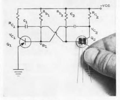
Typical Bendix 2N1008-equipped multivibrator circuit used in digital computers as a frequency divider, and in other medium-speed triggering applications.
