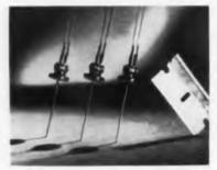
Low current silicon controlled rectifiers in double-ended housing have the stud replaced by a single lead. Units will accommodate high current loads without heat sinks. The 7 models have JEDEC designations 2N1929 through 2N1935. They differ by repetitive peak reverse voltage ratings ranging from 25 v. for the 2N1929 to 300 v. for the 2N1935. The dc load current rating is 1.1 m. General Electric Co., Rectifier Components Dept., W. Genesee St., Auburn, N. Y.
