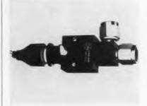
The VA-511 produces 50 w. min. power at 10.0 GC and operates at 10 kv, 60 ma. This fixed-freq., 2cavity oscillator has an FM noise figure less than 1 CPS, and is electrostatically-focused. Weighs less than 24 oz., measures  $6\frac{1}{4} \times 2\frac{1}{4} \times 1\frac{3}{4}$  in. Varian Assoc., Tube Div., 611 Hansen Way, Palo Alto, Calif.
