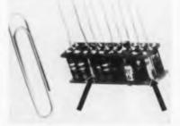
Use include sandwich-type circuit construction. Made in lacquer coated, durez coated or epoxy molded cases, depending on dia. and or test requirements. Body O.D. 10 pf-1000 pf lacquer coated, 0.060 in. max.; durez coated 0.090 in. max.; molded 0.105 in. max. Placquer units can be made as high as a 100 vdc rating. The durez and molded units will meet Mil-C-11015B requirements when tested using Cerafil ratings. Hi-Q Div., Aerovox Corp., Olean, N. Y.
