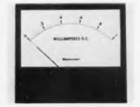
They are gasket sealed to keep out dirt and moisture, and steel enclosures protect the movements from effects of magnetic fields and stray r-f. These front mounting panel meters, (approx. 4.1 x 4.7 in.) use glass windows to eliminate errors due to static charges. Scale length is 3.97 in., standard accuracies are 2%. Among 95 standard models available are ammeters, milliammeters and microammeters. Helipot Div., Beckman Instruments, Inc., 2500 Fullerton Rd., Fullerton, Calif.
