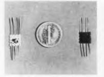
Microminiature flip-flop consists of 12 pre-selected encapsulated components, each passivated by a silicon oxide film and mounted on a ceramic substrate measuring 0.310 x 0.310 in. The flip-flop contains the following microminiature components: 6 semiconductor resistors, 2 silicon dioxide capacitors, 2 epitaxial planar transistors and 2 fast-switching planar microdiodes. General Instrument Semiconductor Div., 65 Gouverneur St., Newark 4, N. J.
