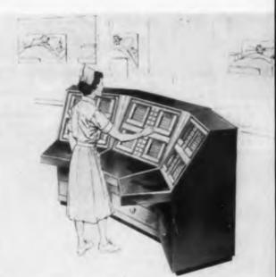
Fig. 1: A single nurse can monitor the condition of a dozen intensivecare hospital patients with this Minneapolis-Honeywell electronic medical system. Mounted on the nurse's central station console is a recorder-alarm unit for each of the 12 patients.
