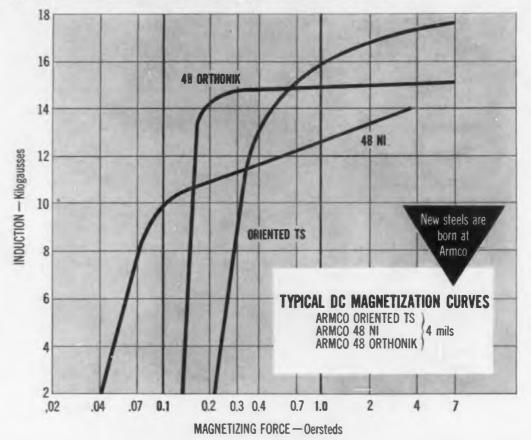
Armco Thin Electrical Steels and nickel-iron alloys. Armco 48 Ni and 48 ORTHONIK®, offer a wide range of magnetic properties, thicknesses and costs. They enable you to select core material for most effective and economical design of communications, computer, control and other high efficieucy equipment.
