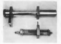
Operating freq. is from 400 to 1000 MC. When used with 2C36 or similar UHF triodes, 10 mw of power into a 50 to load is achieved. A ruggedized anti-backlash tuning mechanism retains accuracy and resetability under severe shock. The oscillator is the heart of the Model TS418 Signal Generator which is both CW and pulse modulated. Entire unit designed to conform to Mil-E-5400. Frequency Standards, P. O. Box 504, Asbury Park, N. J.
