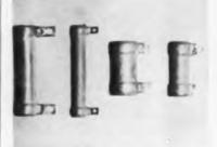
This is due to a new high temp. coating. Operating temp. range is from -55°C to 350°C. All sizes meet functional requirements of Mil-R-26C, Char. V. Six sizes in 4 wattages (5, 6, 7, and 11 w. at 25°C). Resistance ranges from 10 Ω to 200 KΩ, depending on size and tolerance. Tolerances: 0.05%, 0.10%, 0.25%, 0.5%, 1% and 3%. Temp. coefficient 20 ppm/°C. Dale Electronics, Inc., Columbus, Nebr.
