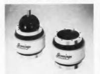
The vacuum dielectric allows smaller units than other high voltage capacitors. It is non-puncturing, and self-healing after moderate overloads. Dielectric or corona loss is low. No plate surface contamination due to dust and moisture. Ceramic vacuum capacitors include variable capacitors up to 1000 pf and peak test voltages to 30 kv. Fixed capacitors are available up to 1225 pf and peak voltages to 45 kv. Jennings Radio Mfg. Corp., P. O Box 1278, San Jose, Calif.
