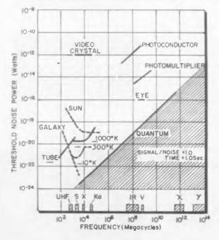
Fig. 5: Sensitivity of linear and nonlinear receivers.
