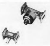
Shielding is provided for interference free operation at low r-f levels even in areas of exterior high level fields. The standard calibrated units provide an attenuation range of 30 db. with calibrations provided at 5 db. points at a single freq. (Model 611 covers 8.20 to 12.4 GC; Model 711 covers 12.4 to 18.0 GC). The standard variable pad attenuator provides an attenuation range of 20 db. (Model 613 covers 8.20 to 12.4 GC). Waveline Inc., Caldwell, N. J.
