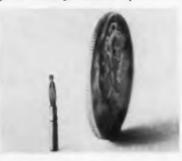
Amphenol Micro-Rac is a rack and panel type connector. The Amphenol strip is for in-line, stacked and special configuration. Max. current rating in each case is 3 a., with a temp. range -65 to +250°F. Miniaturization is through the use of wire-form "poke-Home" beryllium-copper contacts, spring-tempered to resist deformation. The connectors are for use in test and communications equipment, computers and missiles. Amphenol Connector Div., Amphenol-Borg Electronics Corp., Cicero, Ill.
