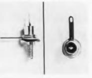
Silicon Power Rectifiers have forward voltage drop of less than 1 v. and a dynamic impedance as low as 0.00350 at rated current. Surge currents to 240 a. can be safely applied on the 12 a. units for 1 cycle at 60 CPS, same amperage can be obtained with the reverse polarity units. Units are said to operate at 1 KC or better. 6 and 12 amp units are available in improved "B" versions of the 1N1199-1N1206 series. Hughes Aircraft Co., Semiconductor Div., 500 Superior Ave., Newport Beach, Calif.
