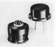
TXBP-018-028 is made entirely of beryllium copper with spring finger construction. Will fit case dia. from 0.175 to 0.190 in. Mount by pushing onto transistor and will not damage case. Suitable for printed circuit boards, chassis and heat sinks. Available in insulube or black cadmium finish. TO-18 Transistor Heat-Dissipating Retainers mount to chassis by screw-attachment. IERC Div., International Electronic Research Corp., 135 W. Magnolia Blvd., Burbank, Calif.
