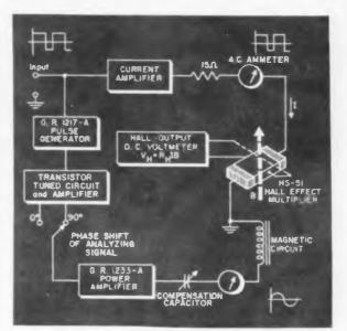
Fig. 2: This Fournier Analysis System is the realization of the block diagram shown in Fig. 1c.
