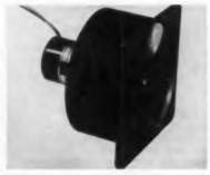
Power requirements: 1  $\phi$ , 117 v., 60 CPS source. Blower is enclosed in a precision cast aluminum housing for max ruggedness. Continuous operation life is rated in excess of 2500 hrs.; unit is designed to meet appropriate MIL specs. Mounting flange dimensions are 3.44 in. sq.; bolt holes spaced 2.75 in. apart. Overall length is 3.25 in. Weight: 12 oz. Globe Industries, Inc., 1784 Stanley Ave., Dayton 4, Ohio.
