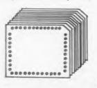
Fig. 2: "Deck" of cards and "needle" Needle" is inserted lifted and cards notched at that point drop out
