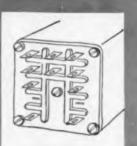
ALL TERMINALS on one panel... permits insertion in printed circuit board.
