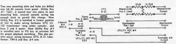
New Mrg Holes MONITOR LEVEL & Slot for New \$22 o Position of o PLAYBACK RECORD VU Key TM'ST'E AUD TM'ST'R TTOJ SP \$23 \$22 66) SIR 5 20 \$17 SIC .2 m MAGNE PGM MAGNE TAPES . New Mtg Holes & Slot New Utility Key for New Utility Key #4 Position GATES SA-40 CONSOLE FRONT PANEL MODIFICATIONS
