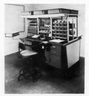
Fig. 1: Dual back to back Hughes Production Station. Also available as a single side station, separate super structure or separate work bench. A wide choice of module boxes, trays, racks, etc., is offered.
