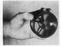
The new 60 CPS Propimax 2 measures slightly over 3 in. in dia.,  $1\frac{1}{2}$  in. deep and weighs  $6\frac{1}{3}$  oz. It moves 17.5 CFM under free delivery conditions. Materials and finishes meet most applicable military specs. Power required is 0.05 a. at 115 v., under free delivery conditions. Mounting is by means of servo-ring. Impeller runs on 2 precision, double-shielded, stainless steel ball bearings. RPM at free delivery is 3250. Rotron Mfg. Co., Inc., Woodstock, N. Y.
