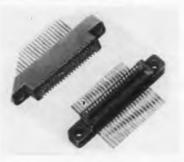
40 contacts with a 0.050 in. centerto-center spacing are mounted in a 1 11/16 in. long molding. Contacts are reliable, patented "bellowform" type, providing coil spring action grip. Recommended test voltage at sea level is 900 RMS, current rating 1 a. Illustrated are wire terminals in 2 positions: straight; and with right angle bend. Body material is glass reinforced Diallyl Phthalate per Mil-M-19833, Type GDI-30 specs. Continental Connector Corp., Woodside 77, N. Y.
