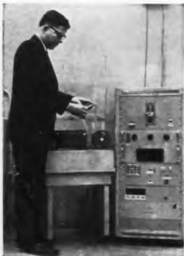
PETROLEUM RESEARCH AND DEVELOPMENT. This precision data logging system, incorporating an NLS V24 DVM, has served Esso Research Laboratories for more than two years in around-the-clock service. The V24 converts millivolt signals to digital form for operating a Friden Tape Punch. The system aids in making pilot plant studies of industrial processes.
