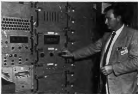
MISSILE PRODUCTION TESTING. An NLS M24 Multi-Purpose Instrument performs an important part in the missile functional test system at Boeing Airplane Company's Missile Production Center in Seattle, Wash. The system automatically applies more than 400 go/no-go sequenced tests to ground-check missile flight reactions from launch to intercept. The M24 and the printout portion of the system monitor application of test stimuli and isolate malfunctions.
