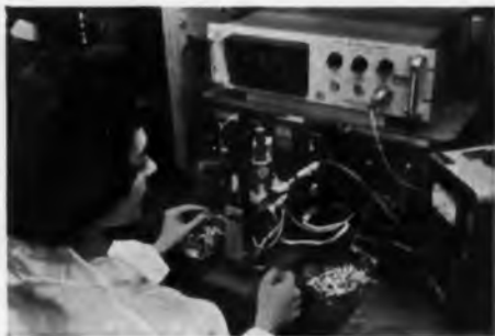
PRODUCTION TESTING. A 481—one of a battery of NLS DVMs—measures Zener diodes for separation into voltage categories at the Semiconductor Products Division of Motorola, Inc. Measuring speed for this operation was doubled by use of the NLS digital voltmeters.
