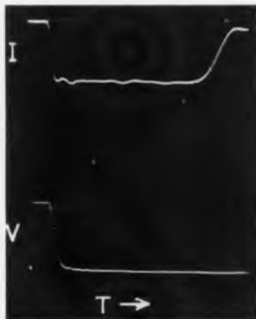
Fig. 5: Photograph shows the current and voltage transients during pulse discharge in the practical circuit (Fig. 4).
