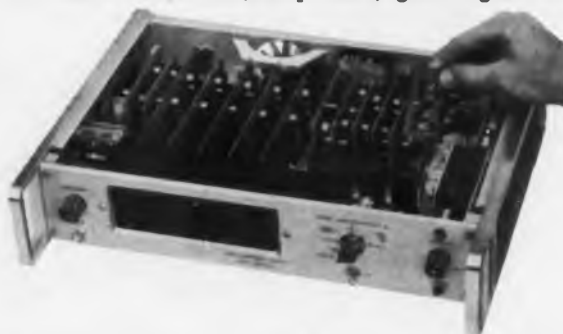
Note clean, compact, easy-to-service physical arrangement of new solid-state counters.
