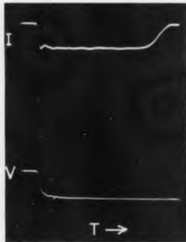
Fig. 3: Scope photograph shows current and voltage transients during pulse discharge in the basic circuit (Fig. 1).
