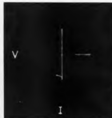
Fig. 2: E-I characteristics of a diode. The scales are 50 v/division; 1 ma/division.
