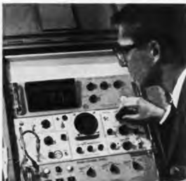
MISSILE TRACKING SYSTEMS. The Azusa Test Set, designed by General Dynamics/Astronautics, A Division of General Dynamics Corporation, includes an NLS V35 DVM. This set checks the power and transmitter portions of the airborne package of the system which is used for tracking all missiles launched from Cape Canaveral. Functions of the V35 include monitoring of 28-, 100- and 1,500-volt power supplies; calibrating telemeter transducers; and adjusting Klystron beam, bias and modulator voltages.
