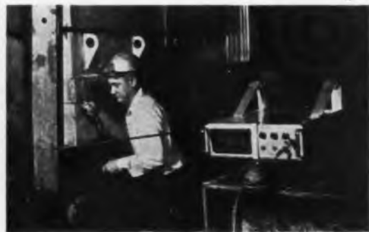
ELECTRO-CHEMICAL ANALYSIS. Savings of as much as $8,000 a year on one particular project are expected to result from use of an NLS 481 DVM at Diamond Alkali Company's plant in Deer Park, Texas. By accurately measuring small changes in voltage and voltage drop, it permits optimizing the efficiency of producing chlorine from sodium chloride brines by electrolysis.
