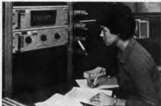
CHECKOUT OF MISSILE COMPONENTS. An M24 checks electronic components at Autonetics, a division of North American Aviation, Inc., as part of the High Reliability Program for Minuteman ICBM. The operator is shown measuring resistance. By turning a front panel knob on the M24, she can also measure DC voltage or DC voltage ratio.
