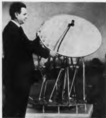
Mack Suliteanu, EDL engineer who developed the antenna system, is shown pointing out antenna's feed horn buried in its foam surface.
