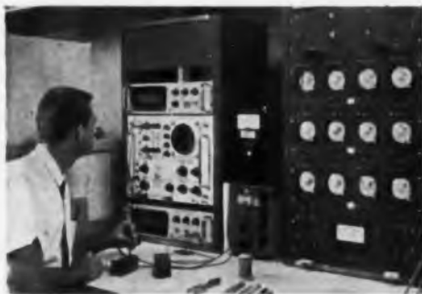
MISSILE CHECKOUT. Two NLS DVMs team up on checkout of equipment for the GAM-77 Hound Dog Missile at the West Coast Laboratories of Mallory Electronics Company, A Division of P. R. Mallory & Co. Inc. The 481 (bottom) calibrates remotely settable timers for the Hound Dog and the V35 (top) is used for final checkout of these devices. "By using DVMs, we are able to eliminate human error in final inspection," said a Mallory executive.
