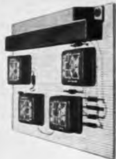
Printed circuit board using 4 FL relays was designed by the Martin Company, Orlando, as part of ground support equipment for a major missile project.
