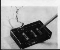
the circuit is ready for service. An excellent bond forms between the original and new resin-only a thin knit line re-
