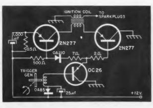
Fig. 5: Drawing illustrates a method of incorporating a speed meter into a conventional type of ignition system.
