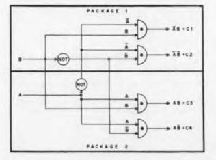
Electronic switching is bringing the telephone industry into a new era. Schematics, loaded with recurring component symbols, would be confusing. Here is a basic circuit building block system which aids the designer, packaging engineer, and maintenance personnel by including logic, packaging, and normal state information as well as test points, connectors and waveforms.
