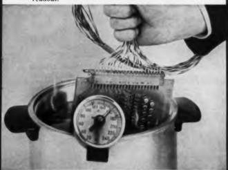
"NO POTS AT ALL" STABILITY of the NLS V44 DVM is checked by the "boil in oil" test at 158°F. This feature eliminates all trimming of decade and amplifier circuits.
