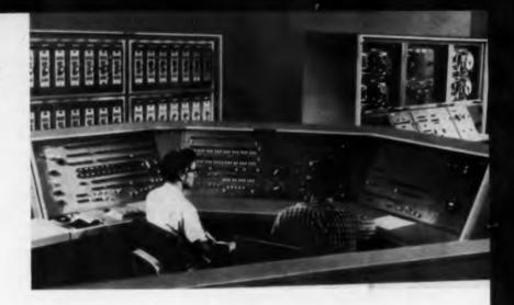
checks for their proper operation. If the operation of an exercise is not proper, an error routine is entered. Additional exercises are introduced, allowing decisions to be made about the source of the malfunction. When the location of the error is ascertained, the computer stops, an indicator labelled "diagnostic error" lights, and a number is displayed on the console panel. This number appears as a pattern of lights in the computer test register indicators.
