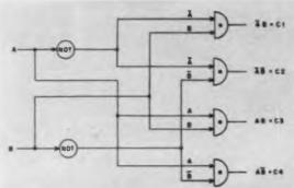
Fig. 7: Four gates are now checked by the same number of combinations which checked one gate in the original example.
