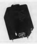
The device features an input impedance of greater than 100 kn, a differential between pull-in and dropout of less than 1%, switching accuracy of ±5% over the temp. range, and adjustability over broad voltage ranges. Available in various contact configurations and ratings, the units are normally hermetically sealed; can be provided to sense either ac or dc voltages, and use either ac or dc auxiliary power depending on type required. HI-G, Inc., Bradley Field, Windsor Locks, Conn.
