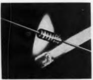
Subminiature mesa diffused junction general purpose glass diodes, designated types 3G05 through 3G30, the 7 types of the new series have peak reverse voltage ratings ranging from 50 to 300 v. Applications include relay circuits for both dc operation of an ac relay and arc suppression, and power supplies where a low cost, subminiature rectifier is called for. Operating temp. range from -55°C to +150°C. International Rectifier Corp., 1521 E. Grand Ave., El Segundo, Calif.
