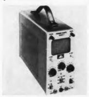
The Primer-Scope®, Mark I, is small and versatile, in the low price range. Weighing under 6 lbs., favors its inclusion in heavy service kits. Its size is 7½ x 3½ x 11½ in. The main scope component is a special 3 in. Rayonic® CRT, incorporating an integral magnetic shield to prevent stray or spurious pickups. Accelerating potential is approx. 840 v. Trace is bright and sharp. An instruction manual is included. Waterman Products Co., 2445 Emerald St., Phila. 25, Pa.
