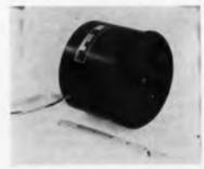
Vaneaxial blower, VAX-4.5, designed for delivery of 140 cfm or air against a static pressure of 5 in. of water at 25,000 ft., sea level output is 77 cfm of air against 5 in. of water. Motor is wound for 200 vac, 400 cps, 3  $\phi$ ; other power requirements can be met, including dc and universal ac/dc. VAX-4.5 is 411/16 in. in dia. by 3½ in. long and weighs 5½ lbs. Unit rated for 1000 hr. life at 110°C ambient. Globe Industries, Inc., 1784 Stanley Ave., Dayton 4, Ohio.
