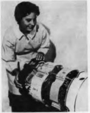
Technician aligns a wheel package on tension bolts during assembly of a missile electronic section at Convair (Pomona, Calif.) Div. of General Dynamics Corp. Wheels constitute the entire airframe of the electronic sections of some guided missiles produced at Convair.
