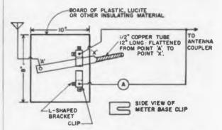
Antenna meter switch can be made from "junk box" parts.
