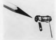
Mini-Trimmer® model, equipped with 1 wire lead and 1 tab lead, made in 4 models with capacitance ranges as broad as 1 to 18 pf. Featuring fixed cavity tuning and a linear tuning curve, the new type makes posisible sturdy, 2 terminal mounting for printed circuit boards or for custom applications. Combination of glass and hardware provides low inductance at high freqs., thermal stability and ruggedness. Electronic Components Div., Corning Glass Works, Corning, N. Y.
