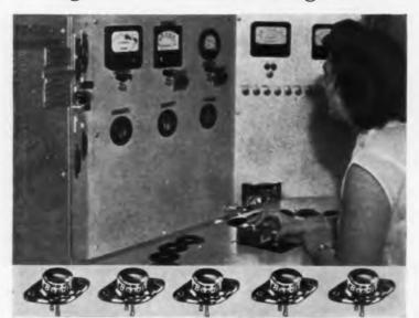
100% specification testing assures transistor rating.
