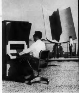
A RADAR display which presents a progressive three-dimensional picture of the trails of aircraft under surveillance by an operating radar, has been demonstrated by Hughes Aircraft Co., Fullerton, Calif.
