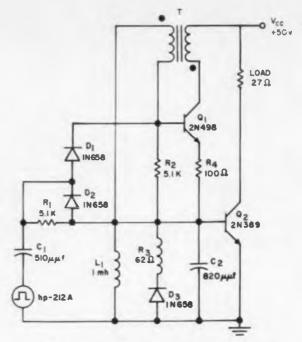
Fig. 9: This blocking-oscillator drives ferrite memory cores.
