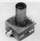
These packaged units, called the SO series produce a signal whose freq. is controlled by applying either a current or voltage, eliminating manual tuning requirements. In a typical vacuum-tube, single-band unit, a change in freq. of 5 to 1 is produced by applying a control current between 0 and 70 ma over the 10 KC to 200 MC range. Units require an extended power source of 150 v. at 30 ma and 6.3 vac at 0.4 a. Increductor Magnetics Dept., Trak Electronics Co., Inc., Wilton, Conn.
