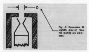
The third offender, handling and storage, pertains largely to the male part. This is because it is not only more apt to be handled, but usually has a pin protruding into space with no physical protection and with mechanical strength sufficient to withstand only a minor jar without bending.
