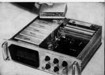
PLUG-IN OIL-BATH STEPPING SWITCHES in Series 30 instruments outlast dry switches by a factor of five . . . completely eliminate periodic disassembly for manual lubrication of switches.
