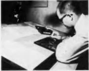
Fig. 3. Master is corrected using specially prepared touch-up fluid.
