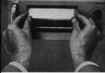
SNAP-OUT READOUT, exclusive on all NLS digital instruments, permits 20-second bulb replacement through front panel without tools. Precisely engraved readout numerals can be read all day from close up or far away without eye fatigue.
