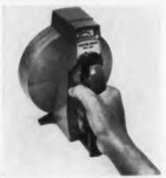
Designed for hand-carrying or to stand and operate unsupported, it has a strong plastic housing, one knob operation without freq. range switching. Model B86B1 operates over a freq. range from 400 MC to 10 GC has a single integral antenna and utilizes standard, large-capacity mercury batteries. Providing a rapid and simplified means for monitoring power density over its wide band, the instrument responds to all planes of polarization. Sperry Microwave Electronics Co., Clearwater, Fla.
