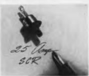
The TI-150 Series of 25 a diffused silicon controlled rectifiers eliminate using low-current SCR's in parallel to handle high-current applications. Packaged in TI's new SCR stud package with an average rectified forward current of 25 a at 100°C, it carries a max. dc current of 35 a at 95°C. Rated breakover voltages, both forward and reverse, for the series are 50, 100, 200, 300 and 400 v. Texas Instruments Incorporated, P. O. Box 5012, Dallas 22, Tex.
