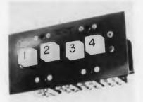
Actuating any of the 4 push button causes the previously depressed button to return to normal position. Combination of over center action station button and interlock inclusion prevents the "all station up" configuration. Electrical rating is 5 a @ 125/250 vac; 5 a (Res) @ 30 vdc; 2.5 a (Ind) @ 30 vdc. Pushbuttons individually illuminated with standard MS 25237 type lamps replaceable from the front. Control Switch Div., Controls Co. of America, 4218 W. Lake St., Chicago 24. III.
