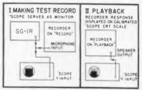
Block diagram shows recorder setup with oscilloscope and SG-1R
