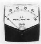
Four sizes offered in transparent and black molded plastic: 220-M, scale length 2.5 in.; 320-M, scale length 3.34 in.; 420-M, scale length 4.5 in.; and 820-M, scale length 7 in. "M" Series have 3-way terminals permitting use of time-saving push-on solderless connectors; or conventional solder terminals; or conventional wrap-around (binding head screws). Have Triplett-Bar-Ring® self-shielded movements with Alnico magnets. Triplett Electrical Instrument Co., Bluffton, Ohio.
