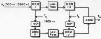
Fig. 7: A third SSB system uses two modulators.
