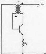
A common-emitter blocking oscillator pulse generator may use either base or emitter circuit timing.
