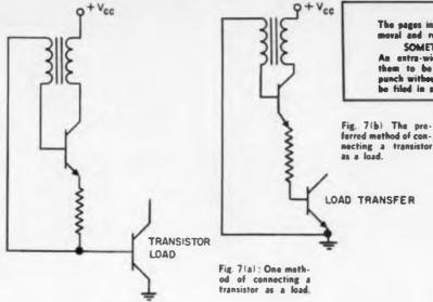
their "clamp" voltages. Two methods of connecting a clamping load are indicated in Fig. 7.
