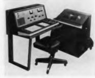
The Analytical NMR Spectrometer System is sensitive to the hydrogen nucleus at an operating freq. of 60 MC and a magnetic field strength of 14,092 gauss. Typical volume of a liquid sample is 0.2 to 0.4 cc. (cylindrical). Instrument can resolve 2 lines separated by 1 part in 10" and has sensitivity sufficient for a wide range of analytical problems. Power is 208-230 v., 1¢, at 50 or 60 CPS (as specified). Instrument Div., Varian Associates, 611 Hansen Way. Palo Alto, Calif.
