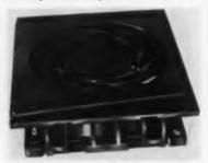
It measures the same as the former Muffin basic configuration providing interchangeable mounting. Output capacity is 100 cfm at free delivery. It operates on 115 v., 60 CPS, 1 ø. Available as a skeleton, venturi, or grilled fan. Incorporated new rigid leads between motor and redesigned terminals, both fabricated as integral parts of the housing eliminate internal electrical breakdown. New bearing design results in smooth, quiet, long life. Rotron Mfg. Co., Inc., Woodstock, N. Y.
