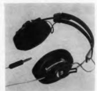
It is also well suited to recording laboratories, record shops and for private practice on such electronic instruments as organs. Max. sensitivity is better than 90 db. SPL for 1 mw. input, achieved with a self-supporting voice coil, has a freq. response of 30 to 15,000 CPS. It has an impedance of 8Ω. Headset consists of a Mylar® diaphragm, Tenite® cups, and one piece stainless steel construction. Communications Accessories Div., Telex, Inc., 1633 Eustis St., St. Paul 1, Minn.
