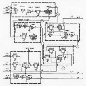
To assist the maintenance man, package connector and test point information for the circuit is shown on the diagram. In addition, associated with each "input-output lead" is a typical waveform picture. The normal state of each basic circuit is indicated by the cross hatching shown within each logical symbol. The cross hatching indicates that the output terminal of the basic circuit is at zero potential.
