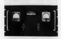
LA Series models have line regulation better than 0.05% or 8 mv, whichever is greater, for input variations from 100-130 vac. Load regulation is better than 0.10% or 15 mv, whichever is greater, for load variations from zero to full load. Swing-open backs permit easy servicing in rack, all major component terminals are accessible from the rear. Rated for continuous operation at 50°C ambient, Lambda Electronics Corp., 515 Broad Hollow Rd., Huntington, L. I., N. Y.
