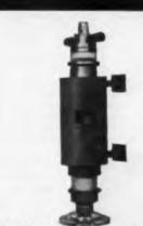
Z-3091: Periodic permanent-magnet focus high-power traveling-wave tube
