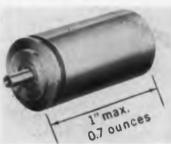
Type 5351-01 is only 1 in. long, weighs 0.7 oz., has 0.12 oz. in. torque at stall and 47,000 rad./sec. torque to inertia ratio. The unit can operate continuously at -55°C to +125°C temp. range. No load speed is 9,500 RPM min. Rated voltage at 400 CPS is 26 v. (can be available in 18 v. or 33 v.). Effective resistance at stall 400Ω. Corrosion resistant materials are used throughout. John Oster Mfg. Co., Avionic Div., Racine, Wis.
