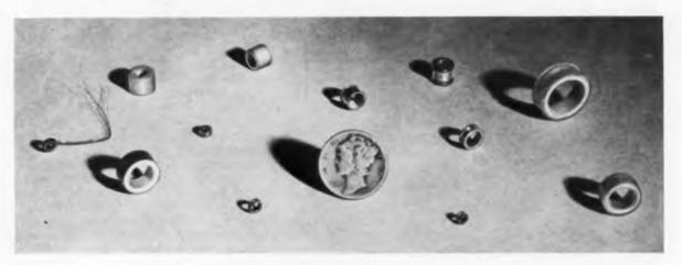
Armco 48 Orthonik and 4-79 Ni offer advantages for wide range of electronic components. Now available in cost-reducing wider widths.
