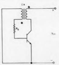
Fig. 1: Elementary common - emitter blocking oscillator with base timing.
