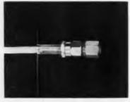
The unit features Crimp-On design and reduces assembly time over 60%. The plug provides a screw-on connection for  $50~\Omega$  cables mating with cable jacks, bulkhead jacks, bulkhead receptacles, cable feedthroughs, printed wiring receptacles, rightangle printed wiring receptacles. The assembly is stronger in pull-out strength than the cable itself. Sealectro Corp., 610 Fayette Ave., Mamaroneck, N. Y.
