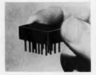
The first BIPCO® module offered is a Binary Coded Decimal-to-Decimal Converter using the 4-2-2-1 code. This device contains 40 silicon diodes and is designed to drive a Nixie® indicator tube directly from inputs encoded in the binary coded decimal form. Typical specs. for the individual diodes are: minimum forward current at 1 v. = 10 ma; max. inverse current at 100 v.,  $25^{\circ}C = 5 \ \mu$  amps; PIV = 200 v. Burroughs Corp., Electronic Tube Div., P.O. Box 1226, Plainfield, N. J.
