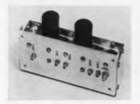
The RF75 is a wide-band r-f preamplifier with sufficient gain (over 15 db) to overcome the noise contribution of a following main amplifier. Typical specifications are: center frequency 160 MC, bandwidth greater than 75 MC  $\pm$ 1 db, gain greater than 15 db, noise figure less than 6 db, input and output impedance 50  $\Omega$ . LEL, Inc., 75 Akron St., Copiague, N.Y.
