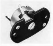
This ¾ in. dia. reliable preset wirewound variable resistor has a mounting plate which insulates the control when mounted on a metal chassis. Connection through the cover to the rotating contact is provided by a solder lug. Rating is 114 w at 40 C derated to no load at 105 °C. Three embossed points on the contactor provide continuous contact between contactor, rotor and cover. CTS Corp., Elkhart, Ind.
