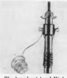
The broadcast band High "Q" Ferrite Antenna Coil can be used with any variable capacitor with a maximum capacitance between 250 and 500 pf. The inductance is easily and accurately adjusted by means of a screw driver slot. The unit is supplied complete with 18 in. of polyethylene insulated antenna wire. Chicago Standard Transformer Corp., 3501 W. Addison St., Chicago 18, Ill. Circle 329 on Inquiry Card
