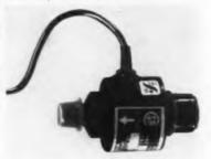
Available in 6 to 64 vdc, 6, 12, 24 and 110-220 v., 60 CPS ac and 110 v., 400 CPS ac models, this valve operates in any position with a max. rate of 1000 CPM at 100 psi. It is also available in water proof and fungus proof models. Using from 1 to 3 w, it will serve under pressures up to 200 psi in temp. from  $-65^{\circ}$ F to  $+350^{\circ}$ F. General Magnetics, Inc. 2641 S. Louisiana Ave., Minneapolis 26, Minn.
