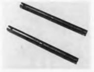
High voltage selenium "channel" cartridge rectifiers are designed for high tension applications such an X-ray, beam welders, precipitators and test equipment. The rectifiers derive their name from the novel channel construction which makes them especially suitable for applications in oil. Dimensions range from 41/2 in. long with a cross section 1/4 in. sq. to 8½ in. long with a ½ in. sq. cross section. Selenium Div., Radio Receptor Co., Inc., 240 Wythe Ave., Brooklyn 11, N. Y.
