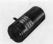
Model BT1004MA measures 1.250 in. long. Designed to operate with transistorized circuitry the unit can also be supplied with any required gear train. Input to the motor is 115 v., 400 CPS fixed phase, 20 v. control phase, center tapped. Tachometer input is 26 v. The output voltage of the unit is 0.24 v./1000 RPM. Total weight of unit is 3.2 oz. Standard operating temp. range is  $-55^{\circ}$ C to  $+125^{\circ}$ C. IMC Magnetics Corp., Eastern Div., 570 Main St., Westbury, L. I., N. Y.
