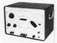
Sine, triangle and arbitrarily modulated suppressed carrier signals of any carrier freq. to 5 kc are available. Applications are: ac or dc servo testing; vibration machine programming; and process control testing. Specs are: freq. range, 0.001 to 10 CPS in 4 ranges at  $\pm 3\%$  of set freq.; output voltage, 20 v. max. peak to peak adjustable; load requirements: min. of 10K; output function: cams supplied are for sine and triangle waveforms. Tensor Electric Development Co., Brooklyn, N. Y.
