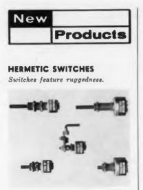
This group of hermetically-sealed, environment-free switches are ruggedly constructed and includes SPDT, 2 PDT, and 4 PDT. Most of these switches are rated at 5 a, 28 vdc res., 2.5 a. at 28 vdc ind., 4 a. motor, or 2.4 a. at 28 vdc lamp load. All these switches feature an ambient temp. range of  $-65^{\circ}$  to  $+250^{\circ}$ F and will pass immersion test Mil-E-5272. Control Switch Div., 1420 Delmar Dr., Folcroft, Pa.
