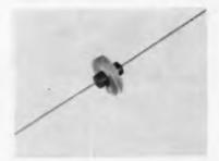
The 1300 series is comprised of 26 video peaking coils designed to assure proper bandwidth and wave shape in high freq. equipment. These coils range in inductance from 20. #h to 950 µh. All but 3 of the 26 coils are wound on 0.187 diameter x % in. long Phenolic form. Numbers 1307 and 1313 are on 22 K resistor form and 1310 on 30 K resistor form. Where resistors are required Mil-R-11 resistors are used. Delta Coils, Inc., 1128 Madison Ave., Paterson 3, N. J. Circle 335 on Inquiry Card
