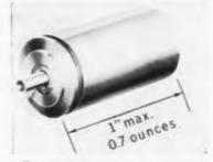
Type 5351-01 is 1 in. long, weighs 0.7 oz., has 0.12 oz. in. torque at stall and 47,000 rad./sec.\* torque to inertia ratio. The unit can operate continuously at  $-55^{\circ}$ C to  $+125^{\circ}$ C temp. range. No load speed is 9,500 RPM min., rotor moment of inertia 0.18 gm.cm<sup>\*</sup>, time constant 0.020 sec. and reversing time 0.034 sec. Rated voltage at 400 CPS is 26 v. (can be available in 18 v. or 33 v.). John Oster Mfg. Co., Avionic Div., Racine, Wis.
