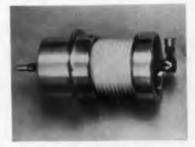
It is for high voltage, high switch rate, floating deck modulator applications. The L-3408's design makes collector current relatively independent of collector voltage over a broad range, resulting in pentode-like current characteristics. Several features of the switch tube are 150 kv max. collector voltage, 20 a. peak collector current, max. 10kw collector dissipation. The tube is 20 x 8 in. and weighs approx. 45 lbs. Litton Industries Electron Tube Div., 960 Industrial Rd., San Carlos, Calif.
