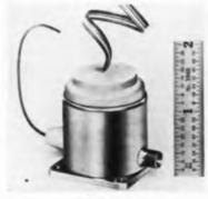
Model LKC-5 is a single cavity oscillator with high efficiency, light weight and no magnetic field requirements. For operation at freqs. from 800 to 13,000 MC, these tubes require only one adjustment to fix oscillation freq. Characteristics are: power output, 5 w cw; beam voltage,  $1200 \pm 50$ vdc; control electrode voltage, 60 v. max.; beam current, 60 ma. max.; half power bandwidth, 7.5 MC. Lewis and Kaufman Electronics Corp., Tube Div., P. O. Box 337, Los Gatos, Calif.
