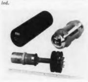
Mercury thermal switch Crystal Oven permits use of a wider range of crystals in both size and freq. The Manson RD-135 Crystal Oven has typical mounting bases: T5½, HC-C/U, HC-13. The unit employs a precision mercury thermal switch, in the form of a miniature thermometer, to provide a constant drift-free reference for close oven control. The heater control circuit is transistorized. The internal structure is completely housed in a thermal bottle. Manson Laboratories, Inc., Stamford, Conn.
