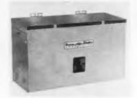
This type of transformer is a code requirement for Class I div. 1 locations in which hazardous concentrations of flammable gases or vapors exist continuously, intermittently or periodically, under normal conditions, during maintenance, because of leakage or during breakdown or as a result of faulty equipment. The line includes ratings from 100 w. to 50 kva, 120 v. input, 120 v. output. Acme Electric Corp., Cuba, N. Y.
