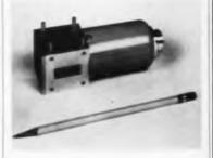
The MA-1064 switches may be pressurized to 45 psi. A low insertion loss of 0.15 db and a max. vswR of 1.10 over the entire waveguide band are featured. Isolation in excess of 35 db is achieved by design of internal chokes and precision machining. Low holding current of 150 MA is achieved without using dropping resistors. This low holding power minimizes heating allowing operation at ambient temps up to  $125^{\circ}$ C. Waveguide Systems Div., Microwave Associates, Inc., Burlington, Mass.
