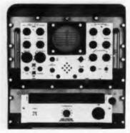
Covers the most widely used communication freqs. for uses including spurious response evaluation, spectrum monitoring, and filter network evaluation. Features are: an operating freq. range of 10 to 1180 Mc. Signal sensitivity is 90 dbm from 10 Mc to 680 Mc, with slightly reduced sensitivity to 1180 Mc. 100 kc and 1 mc crystal controlled calibrator gives precise markers for calibration of viewing screen at any spectrum width setting. Lavoie Laboratories, Inc., Morganville, N. J.
