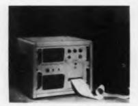
The RS2, has been built as an integrated scanning, measuring and printing system. Unit provides 4digit voltage readings with correct polarity and range. Its accuracy is 0.01% of full scale on each range. Functions include: scanning up to 20-double-pole channels; measuring dc voltage from  $\pm 0.001$  to  $\pm 999.9$  in ranges of  $\pm 9.999/99.99/99.9$ ; printing channel number, 4-digit reading, polarity and decimal point placement. Non-Linear Systems, Inc., Del Mar, Calif.
