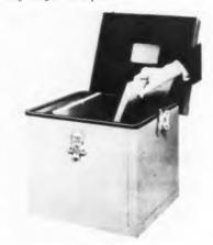
The container is constructed of stress reinforced Netic S-3 magnetic shielding alloy, meeting Mil. drop and environmental specs. Shock absorbing liner allows simple positioning of  $^{1}_{4}$  to 2 in. wide tapes in any combination. Rubber gasket, pressure seals upon locking, make the container virtually moisture proof. Containers are currently available for 14 in. reels; other sizes can be fabricated. Magnetic Shield Div., Perfection Mica Co., 1322 N. Elston Ave., Chicago 22, III.
