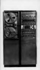
Ampex's Advanced Recorder/Reproducer, the FR-600 used for testing the Minuteman Missile.
