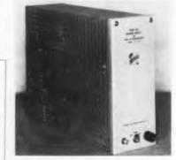
It provides 3 different regulated supplies to these preamplifiers thru octal interconnecting cables. Output voltages include: +135 vdc at 0 to 20 ma,  $\pm 3/v$ ; -90 vdc at 0 to 20 ma,  $\pm 3/v$ ; -6 vdc at 0.7 to 4 a.,  $\pm 5/v$ . Dimensions are 1034 x 4<sup>14</sup> x 13<sup>14</sup> in. Weight is 14<sup>15</sup> lbs. Tektronix, Inc., P. O. Box 500, Beaverton, Ore.
