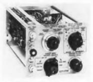
Model 166D Sweep Delay Generator, delays the main sweep of the Hewlett-Packard 160B and 170A o-scopes for detailed examination of a complex signal or pulse train. It offers a new mixed sweep feature to show an expanded waveform segment while still retaining a presentation of earlier portions of the waveform. Thus, both low speed and high speed phenomena can be observed on the same trace. Model 166D's delay time is 1 µsec to 10 sec. Hewlett-Packard Co., 1501 Page Mill Rd., Palo Alto, Calif.
