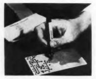
Using the kit's copper-clad Fotoceram grid boards, resist materials to lay out circuit patterns, and etching materials to etch away copper beyond the circuit runs, a designer can produce a printed circuit on glass-ceramic substrate in 15 minutes, without leaving his desk. Corning Glass Works, Corning, N. Y. Circle 347 on Inquiry Card
