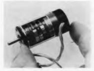
Providing efficiencies as high as 54% through a high flux utilization, the PM-1 requires very low input current at full load. Weighing less than 21/2 oz., the motor is only 7/8 in. in dia. and less than 2 in. long for use in restricted areas. The motor may be provided with internal r-f filters to eliminate obectional freqs. and a governor to control armature speed to within 0.5% of nominal speed under wide terminal voltage and load torque variations. Reflectone Electronics, Inc., Stamford, Conn.
