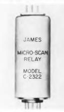
Driving voltage is a nominal 20 v. They have polarized driving systems with center tapped driving coils. Switching circuits are for dry to 10 v. levels with 100 million operations reliability. Models include DPDT and SPDT. Normally open and normally closed circuits are available. James Electronics Inc., 4050 N. Rockwell St., Chicago 18, Ill.
