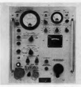
Radio interference set covers from 0.15 to 25 mc. Several types of measurements are available by front panel selection.
