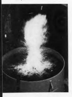
ELECTRICAL explosion techniques are being developed by GE for low-cost shaping of hard-to-form metals like titanium, stainless steel, and tungsten. The controlled explosions create shock waves of such force that intricate contours can be blown into the metals in millionths of a second.
