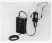
The device consists of a small microphone and a transistorized 10 oz. transmitter. A fixed freq. FM receiver which picks up the transmission can be linked into broadcast or public address systems. The transmitter contains a crystal controlled oscillator operating at high freq. which is directly freq. modulated. It may be used with existing military operations, telemetering, and news and sports events. It covers 20 to 15,000 CPS. The Victoreen Instru-ments Co., 5806 Hough Ave., Cleveland, Ohio.
