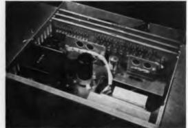
Note the compact, plug-in modular design of the scannerprinter section of the RS2.
