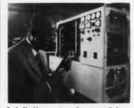
R. A. Koehler examines silicon controlled rectifier used in GE's new inverter designed for use with unconventional power generators.
