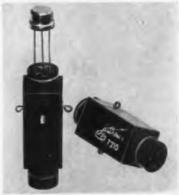
and terminate in rigid solder terminals on each face of body. Body is molded of glass filled Diall FS-5. Socket weighs less than 9 gms. (Cat. No. 72-101.) Jettron Products Inc., 56 Route 10, Hanover, N. J. Circle 357 on Inquiry Card
