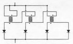
Fig. 6: Reference cell arrangement of balancing transformers.
