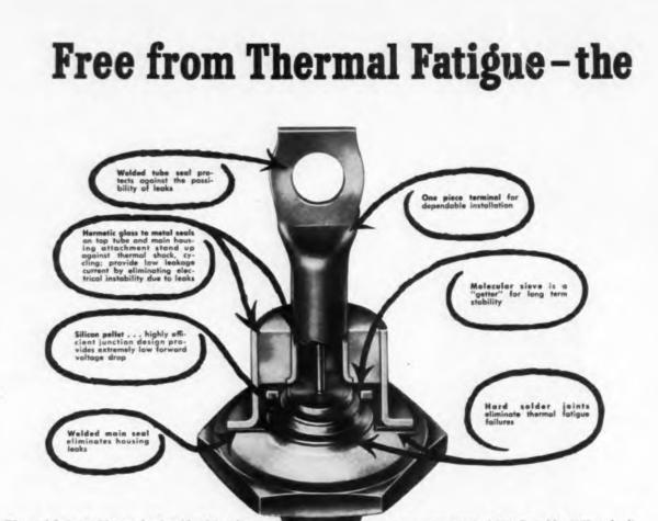
Thermal fatigue of internal soft solder joints has long been a major pitfall in rectifier design. Now, General Electric medium current silicon rectifiers beat the heat and highly cyclical loads with high melting point, hard solder joints that make thermal fatigue failures a thing of the past.
