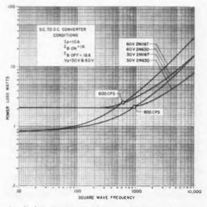
Fig. 2: Cross-over frequency increases with decrease in voltage.
