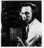
Communications device built by Hughes Aircraft Co. lets jet pilot "talk" to his base by punching indicated panels. Engineer Robert J. Harris demonstrates panel. Communications are twice as fast as normal and can penetrate heavy electrical interference.
