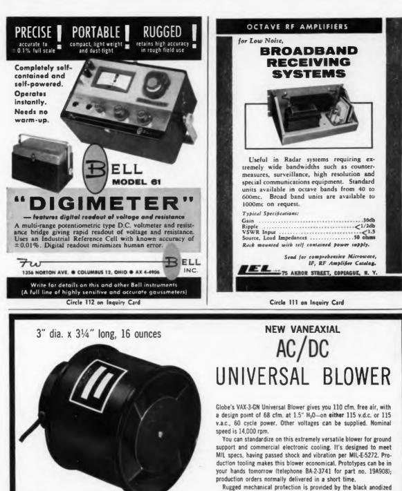
Rugged mechanical protection is provided by the black anodized aluminum housing and propeller. Mount by clamping to servo ring at either end. Nominal life exceeds 1000 hours. Max. current is 0.47 amps at free air delivery. Request Bulletin GNB from Globe Industries, Inc., 1784 Stanley Avenue, Dayton 4, Ohio.
