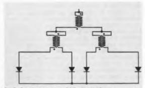
Fig. 5: Cascade arrangement of balancing transformers.
