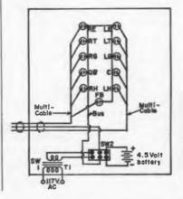
Pictorial hook-up diagram of the announcer's board is seen from the underside. TI is a 6.3 v. 0.7 s. transformers. Battery is actually three flashlight cells in series.
