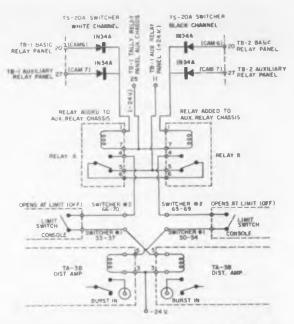
Fig. 2. Shows the connections for controlling burst insertion in the TA-3B Distribution Amplifiers.
