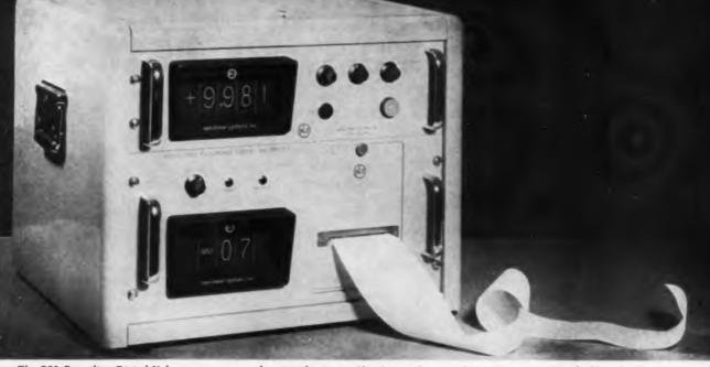
The RS2 Recording Digital Voltmeter – now in volume production at Non-Linear Systems, Inc. – scans up to 20 double-pole input channels . . . measures DC voltage from  $\pm 0.001$  to  $\pm 999.9$  with  $\pm 0.01\%$  accuracy . . . and records input channel number and the 4-digit voltage measurement. Uses include research and development, quality control, environmental and reliability testing.
