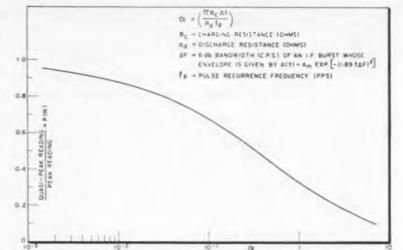
Fig. 6: A ratio of quasi-peak to peak readings as a function of RIFI meter parameters.
