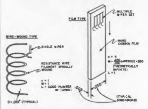
Failure Probability Ratio of Film Pots vs. Wire-Wound ....
