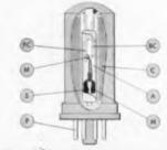
When Coil C is energized, swinger moves from the normally closed contacts BC to the normally open contests FC. This opens the normally closed circuit and closes the electrical circuit through the normally open contacts, FC through stem S, and through proper pins P to external circuit. Mercury M from pool as bottom of switch replenishes mercury dropped after each operation from contact points so circuit is always made and broken through two mercury affaces.
