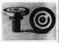
Hermetically sealed transducer pick-up head uses new ceramoplastic.
