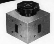
Waveline precision Waveguide Switches are available in seven waveguide sizes to cover the frequency range of 3.95 to 40.0 KMC. These manually operated devices have been designed for applications in the laboratory or for microwave systems to make alternate connections between two waveguide inputs and two waveguide outputs.
