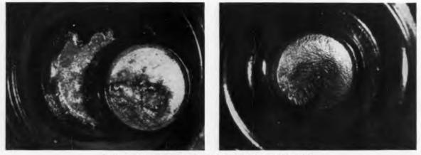
The two test units are shown here. Before the test they were identical in every respect, except that the unit on the left uses conventional tin-lead soft solder, while the unit on the right uses exclusive G-E hard solder joints.
