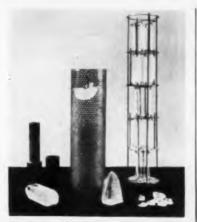
Model of nutrient basket seed plate holder. In foreground (1 to r): synthetic quartz crystal, natural quartz crystal, and nutrient.
