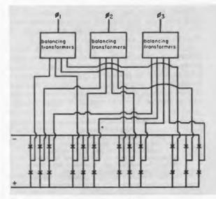
Fig. 7: Three phase bridge of four cells in parallel with the balancing transformers located in the ac leads.
