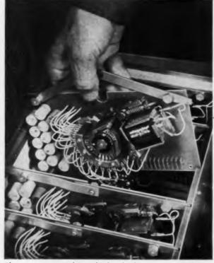
Plug-in stepping switches in the digital voltmeter section of the RS2 permit replacement of all switches and decade resistors in minutes instead of days. The plug-in feature allows almost instant troubleshooting by the substitution method.
