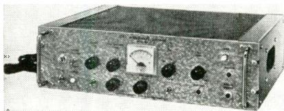
microwave sources constant to  $\pm 1$  db at a fixed frequency. With proper r-f components, power varies less than  $\pm \frac{1}{2}$  db over L, S, C and X bands at slow and fast sweep speeds. Operates with CW signals and internal square wave generator will modulate the r-f signal. Input may be 3 mv to 1 v. Output is 100 v. max. in the range of -50 to +100 v. Frequency response is dc to 100 kc. Alfred Electronics, 897 Commercial St., Palo Alto, Calif.
