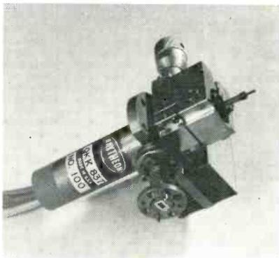
minimum output of 10 milliwatts. The r-f output is through waveguide formed by a mica window. The output flange mates with a standard UG385/U cover-flange. Raytheon Company, Waltham 54, Mass.
