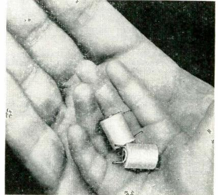
encapsulated in epoxy resin. They meet MIL-C-15305A, Grade 1 and Class B. The units have stable inductance at extreme temperature variations, and also high reliability along with the light weight and miniature size factors. Essex Electronics, Division of Nytronics, Inc., 550 Springfield Avenue, Berkeley Heights, New Jersey.
