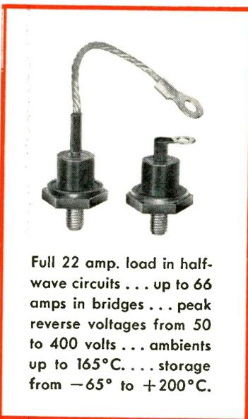
Full 22 amp. load in half-wave circuits . . . up to 66 amps in bridges . . . peak reverse voltages from 50 to 400 volts . . . ambients up to 165°C. . . storage from -65° to +200°C.
