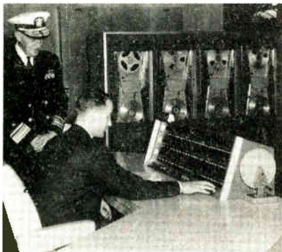
Nucleus of the new weather system is the Control Data Corp.'s 1604 computer. Ampex tape units which provide the system's high transfer rates are shown in the background.
