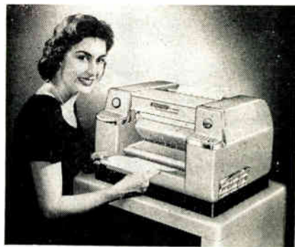
Fig. 14: Ozalid machine can make 200 copies an hour.
