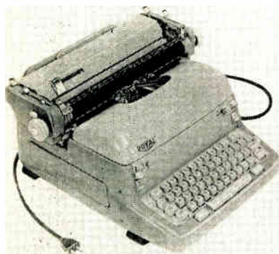
Fig. 2: The electric typewriter offers stroke-controlled operation.
