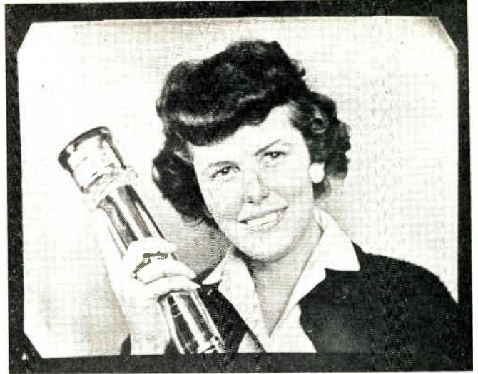
reduction in this problem with the new field mesh image orthicon. Note also the reduction of edge-effect at the fingers and collar.
