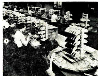
Allen B. Dumont Co., Indus. Electronics Div., Clifton, N. J. has shortened individual assembly modules from 6 ft. to 3 ft. using Bathey Flobins arranged on a bench-type rack mounted on a Lazy Susan capable of revolving 360°. Gilbert-Tucker Assoc. is the designer.
