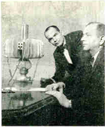
Fig. 20: J. Donald Rauth (R), VP, Martin Co., and Dr. Mostafa E. Talaat, Head of new Energy Conversion Group at Martin, examine Russian-built thermoelectric Generator. Kerosene lamp supplies heat for generator used to power radios in remote Asian areas. Martin acquired the generator to evaluate Soviet technical approaches.
