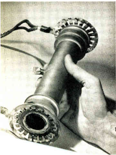
Fig. 28: RCA and Hunter-Bristol Div., Thiokol Chemical Corp. built this thermionic generator which uses rocket exhaust heat. It produced 270 w (80 w/lb) under test. Hollow cylinder fits over rocket-flame tube.
