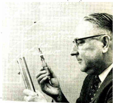
Fig. 27: Dr. William E. Shoupp (Westinghouse) holds combination thermoelectric thermionic test device designed to extract power directly from the fuel elements in a nuclear reactor. Thermionic unit is in the center and thermoelectric elements surround it.
