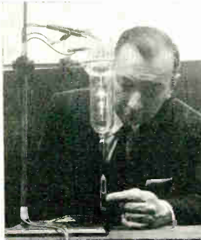
Fig. 23: Dr. J. W. Coltman, Mgr., Electronics and Nuclear Physics Dept., Westinghouse Research Labs., demonstrates experimental thermionic generator. Capsule at base of tube holds Cesium used for neutralizing the space charge effect.
