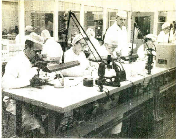
Ultra-clean assembly line techniques are used in thermionic converter assembly line at GE's Schenectady tube plant. Techniques are needed because of small tolerances (0.5 mil) between cathode and anode of vacuum thermionic converters.
