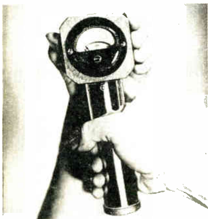
Perspiration can be a serious problem in some manufacturing processes. This perspiration tester by Ameresco, Inc., facilitates screening those persons which may not be satisfactory for handling certain items.
