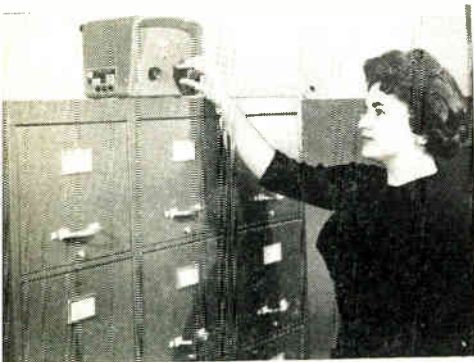
Capacitance alarm developed by Kidde & Co. can be used to protect metal filing cabinets and small safes. Anyone touching protected item will set off an alarm.
