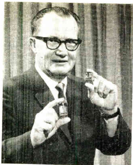
General Electric's I. D. Daniels holds two of the Company's newly developed compactrons. Multifunction tubes are smaller and may decrease costs.
