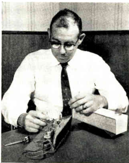
General Electric Development Engineer, Earl Bond, plans typical layout for a small radio using new compactrons. Two of the devices replace five con-miniature electronic tubes. Case under his left hand shows how a compactron radio may look—virtually all speaker.
