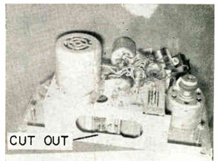
Chassis cut-out will greatly facilitate drive wheel changing on record players.
