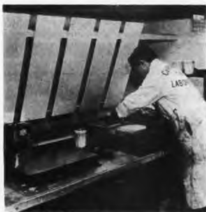
2 Color phosphor 'ink' is applied to glass target plate by silk-screen process. Squeegee passed over stencil forces color through spaces, printing the desired parallel strips
