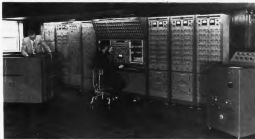
Analog computation center opened by Electronic Associates provides facilities for small companies unable to afford computers of their own. Complete problem patch panels are preset and inserted
