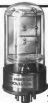
JK STABILIZED G-12 99 kc to 180 kc Frequency tolerance: ±.0005%, 25 to 70°C
