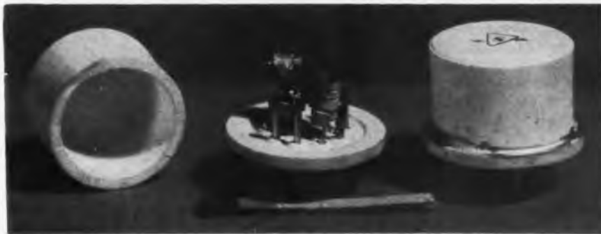
Compactness of "stacked tube" is demonstrated by comparison with match. Ceramic envelope (l) and assembly (c) are placed in bell jar device for evacuation to produce finished tube (r)
