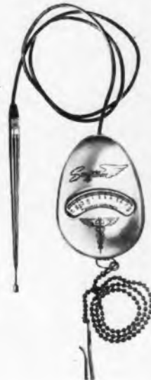
Electronic thermometer takes reading in 3 to 5 seconds. Unit employs thermistor in tip
