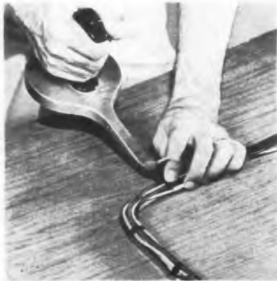
Tape gun speeds electrical harness wrapping
