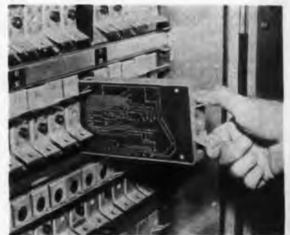
Fig. 2: Standardized etched circuit package is one of two types used as basic building blocks. This delay line unit is one of nearly 800 such packages which provide for 90% of circuit, excluding memory and input
