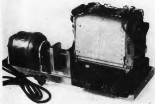
Fig. 3: (l) Pattern recorder with synchronous repeater replacing original paper drive. Fig. 4: (r) Pattern for elliptically polarized antenna
