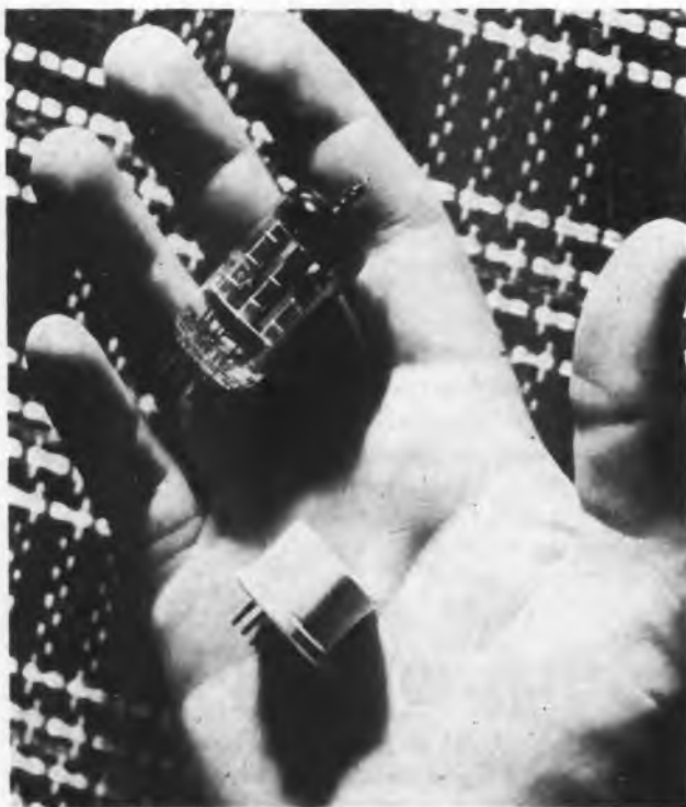
Compactness and ruggedness are major features of "Stacked tubes" developed by Sylvania Electric Products. Conventional tube at top is compared with new type in a ceramic envelope. Both use the same 9-pin miniature basing, but the stacked type is half the height, not including glass type's tip. The new tube culminated in a development contract with the U. S. Navy's Bureau of Ships, and limited production is in progress at the company's Product Development Laboratories, Kew Gardens, N.Y. Details on page 65
