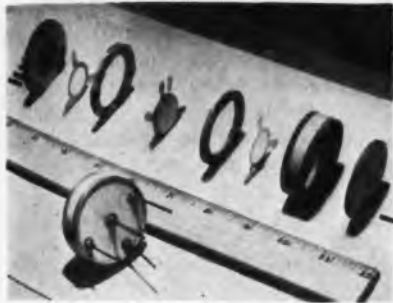
Fig. 9: Exploded view of ceramic twin triode. When assembled, all parts are brazed solidly
