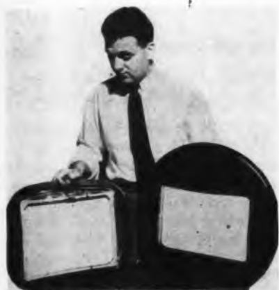
1 At right is a 22-in. metal Chromatron, at left, a developmental 21-in. rectangular glass model. Rectangular glass bulb is better suited for mounting in receiver cabinets.
