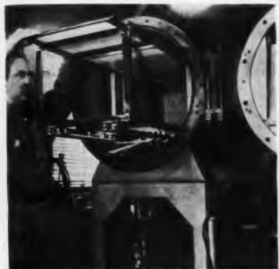
4 Plates are mounted in a vacuum tank for aluminizing. Aluminum is vaporized under vacuum conditions creating a film on the exposed glass surface of the target plate
