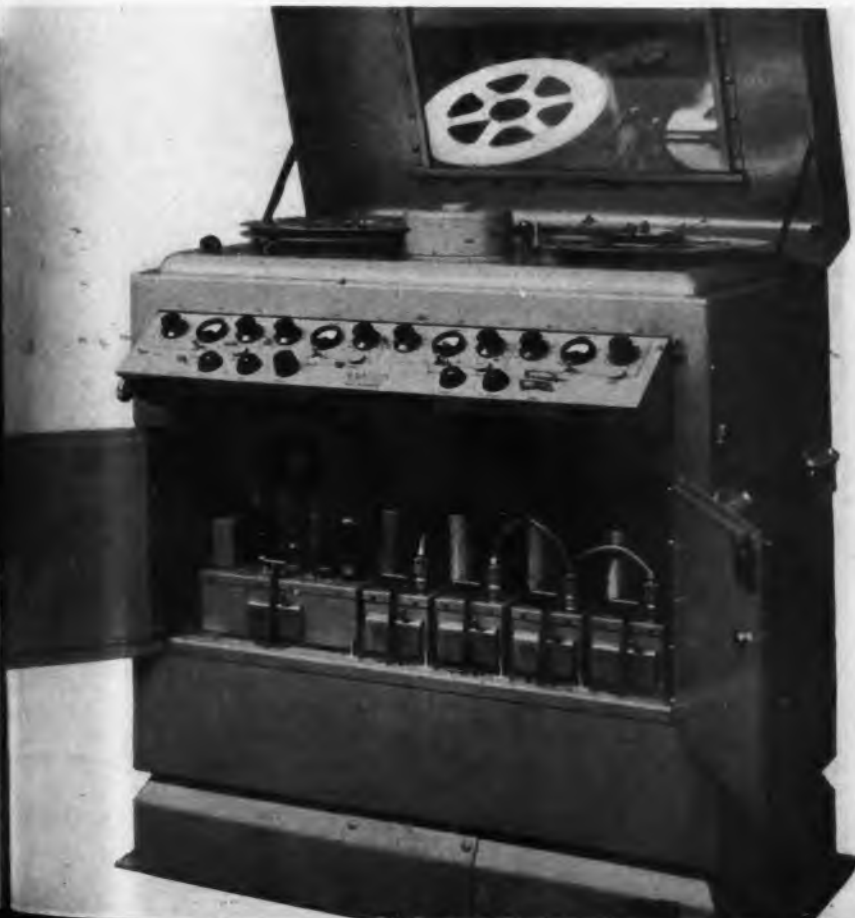
This precision recorder boasts 80 db signal-to-noise ratio, records 4 channels on a single 1/2 in. tape
