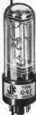
JK STABILIZED G-9J 1 kc to 10 kc Frequency tolerance over range of -40 to +70°C: w/o ckt. adj. ±.03% with ckt. adj. ±.02%
