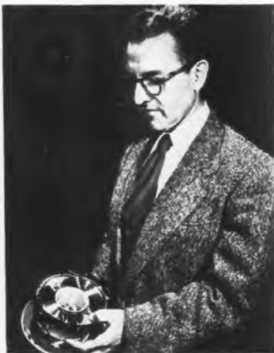
New magnetic deflection yoke for 19-in., 3-gun color TV tubes introduced by General Instrument's F. W. Sickles Div. is held by company's vice-president, Edgar Messing. High efficiency and close convergence are prime features
