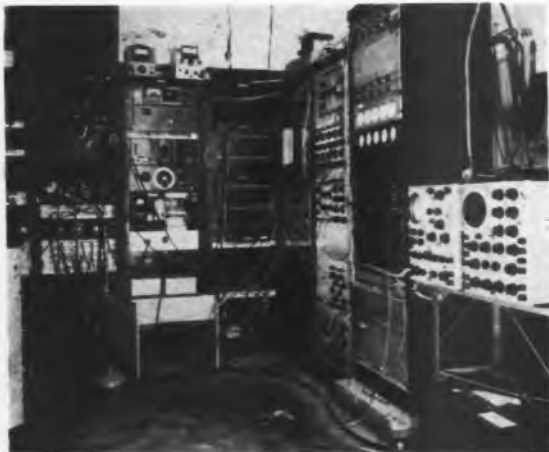
Fig. 2: (l) Room adjoining soundproof room where animals are tested holds "huge kluge" containing 10-channel oscilloscope-camera recorder, master control unit, sound generator and calibration equipment. Fig. 3: (r) Huge kluge system arranged for typical experiment
