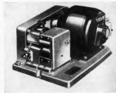
Fig. 7: Oscillator covers range of 500-1,000 MC
