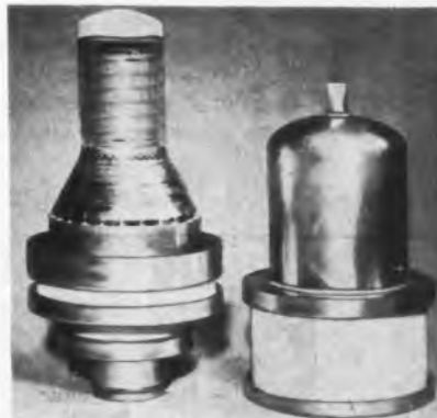
Fig. 6: 20 kw tetrode has ceramic-to-metal seals
