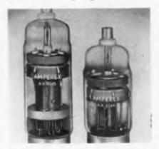
directly interchangeable with RETMA tubes with the same designation. Each is a three electrode Xenon-filled tube with negative characteristics. The inert gas filling enables reliable operation at maximum ratings over a wide temperature range. Complete data is available at the Engineering Department, Amperex Electronic Corp., 239 Duffy Ave., Hicksville, L. I., N. Y.—TELE-TECH & ELECTRONIC INDUSTRIES.
