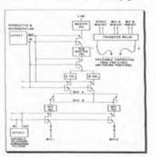
Studio microphone system shows method of switching effects into various circuits. One effect is the telephone and bandpass filters, which may be inserted in any mike channel
