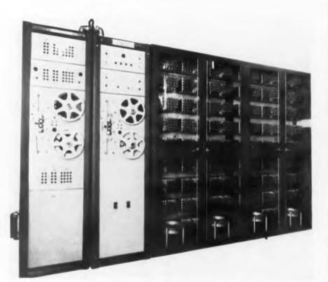
Fig.. 1: Equipment for storing and coding data produced simultaneously by 100 sensing devices
