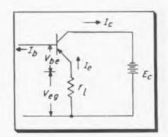
Fig. 17: The grounded collector stage
