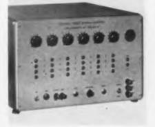
delays from 1 usec to one sec. may be generated or measured. The number of usecs is selected by 6 10-position switches-one for each digit of the delay in usecs. To measure a time interval, the instrument counts the exact number of pulses produced by a 1 MC, crystalcontrolled oscillator during the interval. Potter Instrument Co., Inc., 115 Cutter Mill Rd., Great Neck, N. Y.-TELE-TECH & ELECTRONIC INDUSTRIES.
