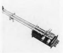
carrier-frequency range extends from 60 to 2,300 MC, and 100% amplitude modulation can be obtained throughout this carrier range. Double sideband suppressed-carrier modulation, and pulse modulation with 60-db carrier suppression between pulses are possible throughout the entire carrier frequency range. General Radio Co., 275 Massachusetts Ave., Cambridge 39, Mass.—TELE-TECH & ELECTRONIC INDUSTRIES.
