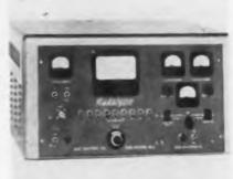
loss or gain, and a receiver frequency of 30 MC. Operating (signal) frequency range is 40 MC to 10 KMC-furnished by external equipment under test. Input rating is 50 mv maximum of 30 MC into 50 ohm line. Attenuators are 0-101 db-(steps, 1, 2, 3, 5, 10, 20, 20, 20, 20.) Precision 10-turn potentiometer, 0-10 db, calibrated. Kay Electric Co., Pine Brook, N. J. ---TELE-TECH & ELEC-TRONIC INDUSTRIES.
