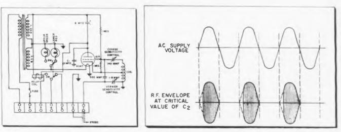
Fig. 4: (1) Operation with positive grid improves stability. Fig. 5: (r) Pattern of oscillation shows crisp snap action between pulses
