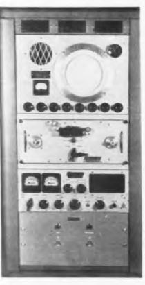
Fig. 1: Playback unit of radar recorder
