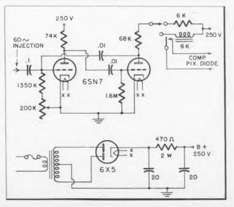
% modulation is seen visually by sampling video signal with this multivibrator and relay arrangement
