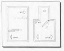
Fig. 1: Movable baffles provide variation in echo
