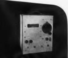
3 Stock models cover 225 to 420 mc. 470 to 890 mc. and 850 to 1275 mc. Special ranges on request.
