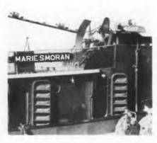
Tugboat lowers mast to duck under low bridges. vessel's radar transmitter and receiver is built entirely within the vessel's antenna housing
