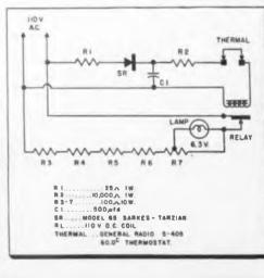
(1) Wiring diagram for crystal even. (below) Box is lined with aluminum, and fastened directly to transmitter. Crystal projects into even through hole in back
