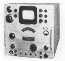
frequency spectrum. A swept i-f yields constant dispersion characteristics independently of the frequency setting. Frequency dispersion from 250 kc to 25 kc can be realized with a resolution of 25 kc. An internal marker measures frequency differences up to  $\pm 12.5$  kc on a 5 in. CTR display. Polarad Electronics Corp., 100 Metropolitan Ave., Brooklyn 11, N. Y.—TELE-TECH ELEC-TRONIC INDUSTRIES.
