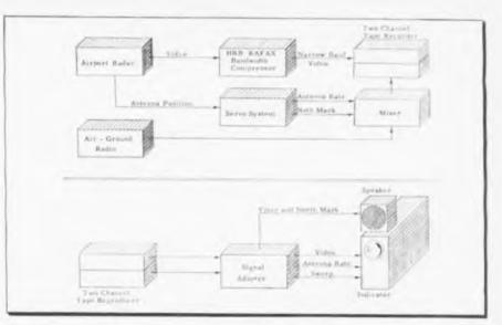
Fig. 2: Air-ground voice, radar video, and antenna position are recorded simultaneously on tape
