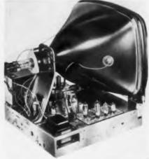
New Admiral TV chassis with 21-in., 90° deflection tube also include printed circuits
