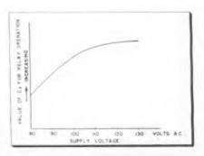
Fig. 3: Supply voltage affects tank capacitance
