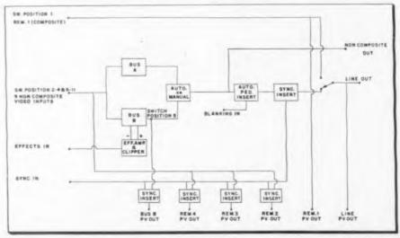
Block schematic of video mixer. Remote 1 bypasses mixing system. Remote 2 through 4 and Camera 1 through 6 (sw 2-4 and 6-11) feed individual tubes on the A and B buses with a standard 1 volt noncomposite video signal. Position 5 picks up any signals on the effects bus. Sync is then added
