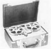
tape speeds with low flutter of  $\pm 0.25\%$ over the full winding cycle of 30 minutes is accomplished by a patented centrifugal flyball governor on the spring motor. Dual track recording provides 2 hr./track or 4 hrs. total playing time on a 5 in. reel that accommodates 600 ft. of standard  $\frac{1}{4}$  in. width tape. **Magnemite Div., Amplifier Corp. of America, 398 Broadway, New York 13,** N. Y.-TELE-TECH & ELECTRONIC INDUSTRIES.
