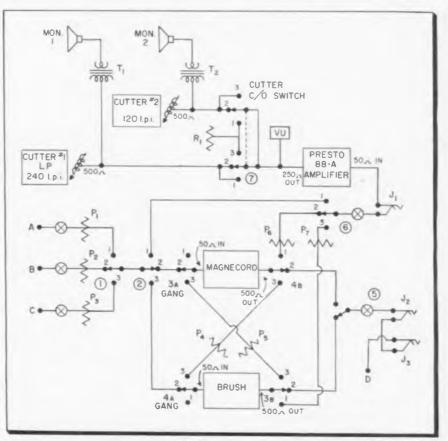
Arrangement of the six switches as seen in diagram allows recording from many sources
