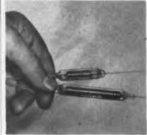
200 kilohms and dissipates up to 5 w. Type RX5 has a rating of 200 ohms to 650 kilohms and is capable of loads up to 10 w. Tolerances can be furnished from a maximum of  $\pm 10\%$  to a minimum of  $\pm 1\%$ . Operating temperature for maintained stability for all three types is listed as from -65 to +225°C. Available in production quantities. Victorcen Instrument Co., 3800 Perkins Ave., Cleveland, O.-TELE-TECH & ELECTRONIC INDUSTRIES.
