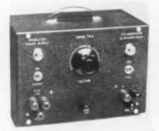
is 0 to 50 ma, max. Regulation, less than 0.1% from no load to full load at line voltages 105v—125v. Ripple, less than 1.5 mv, rms. AC output, 6.3 v at 1.2 amp, max. Output impedance, 2 ohms. Power source, 105-125 v, 60 CPs, 50 w. Dimensions, 5 x 6 x 9 in. Available for standard rack and panel mounting. G. W. Associates, P. O. Box 2263, EL Segundo, Calif.—TELE-TECH & ELEC-TRONIC INDUSTRIES.
