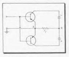
Fig. 18: Parallel n-p-n and p-n-p transistors
