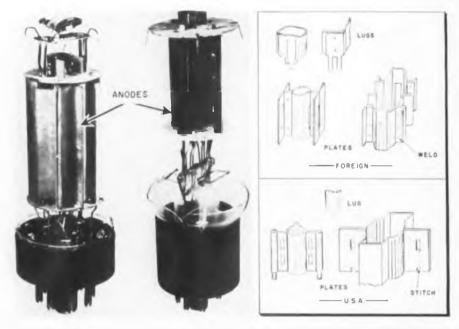
Fig. 9 (1) Aluminized iron plate on imported 61.6 (1). Fig. 10 (r) Simple plate designs cut tooling costs
