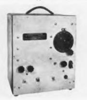
to 890 MC; type 2144-03 from 850 to 1275 Mc. A self-contained passive marker furnishes accurate frequency indication. Marker calibration is in 5 MC steps and frequency accuracy is better than  $\pm 1$ MC in the low range unit and  $\pm 2$  MC in the high range unit. The unit has a 50 ohm output impedance with a source of VSWR of 1.25 : 1 or less. Kollsman Instrument Corp., 80-08 45th Ave., Elm-hurst, N. Y.—TELE-TECH & ELEC-TRONIC INDUSTRIES.
