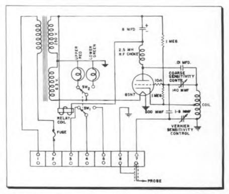
Fig. 6: High level is indicated by de-energized relay in this high level fail-safe indicator
