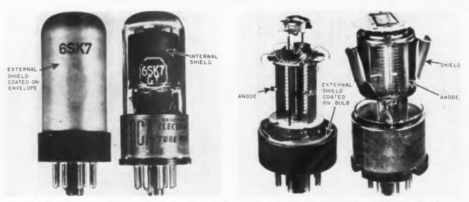
Fig. 1: The well-known 65K7GT pentode (r), with its foreign equivatent (1), Fig. 2: Cutaway view illustrates sharp differences in construction
