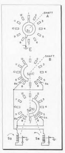
Fig. 1: 3-deck construction and wiper action
