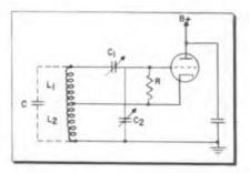
Fig. 1: Basic Hartley oscillator circuit
