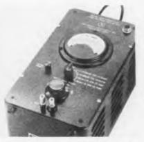
mv to 200 v peak-to-peak is read directly in four decade steps with an accuracy of 3% throughout the spectrum of 0.05 CPS to 30 KC. When corrections are applied, measurements between 0.01 CPS and 0.05 CPS are possible. Pointer flutter is negligible down to 0.05 cps while discharge of the storage circuits for a rapid sequence of readings may be effected by a reset device. Ballantine Laboratories, Inc., Boonton, N. J. TELE-TECH & ELECTRONIC IN-DUSTRIES.
