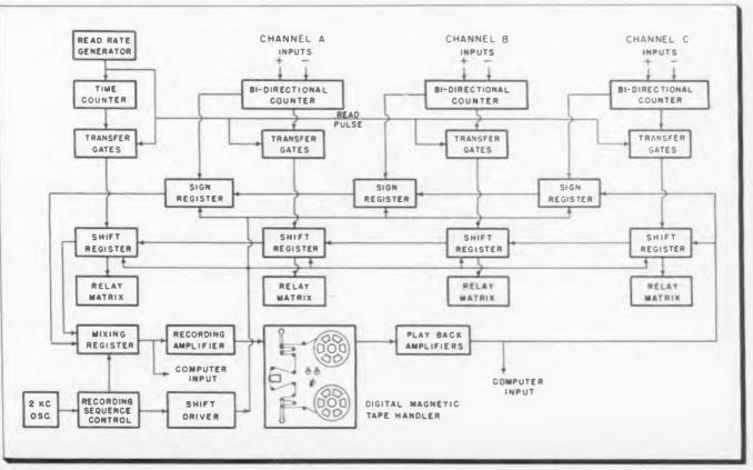
Fig. 4: System for transferring information from magnetic tape to punched cards employs shift registers and relay matrices
