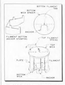
Fig. 15: Filament is part of cage assembly
