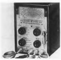
17 megohms, shielded ac and r-f leads, and screw-on connectors. Reads peakto-peak voltages from 200 mv to 2,800 v; dc voltages from 200 mv to 2,800 v; dc voltages of plus or minus polarity from 50 mv to 1,000 v; ac voltages from 50 mv to 1,000 v, r-f voltages from 100 mv to 300 v in the bond of 10 Kc to 300 Mc. Sylvania Electric Products Inc., 1221 West Third St., Williamsport, Pa. —TELE-TECH & ELECTRONIC IN-DUSTRIES.
