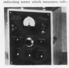
ages between 0-510 v. Reference voltage is indicated on dials associated with adjustments of the voltage. Two adjustments are made in steps of 100.0 v and 10 v. A calibrated multi-turn potentiometer equipped with a vernier dial subdivides the 100.0 or 10.0 v steps, depending on selected range, into 1,000 divisions corresponding to 100 or 10 mv. Furst Electronics, 3322 W. Lawrence Ave., Chicago 25, III.—TELE-TECH & ELECTRONIC INDUSTRIES.
