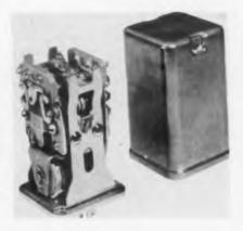
switch circuits are open. One polarity of coil current or unbalance current closes one throw of the switch. Opposite polarity closes the other switch. Rated double-pole sensitivity is 12 mw. The relay measures 25% in. high above octal or magnal socket by 15% in. square. Sigma Instruments, Inc., 170 Pearl St., South Braintree, Boston 85, Mass.— TELE-TECH & ELECTRONIC INDUS-TRIES.
