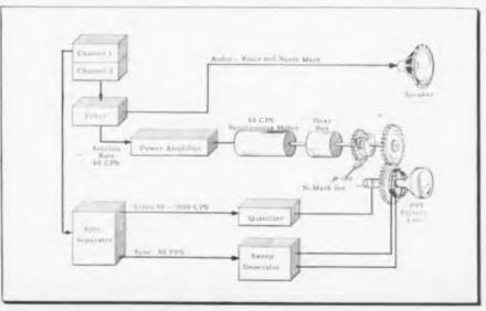
Fig. 4: Reproducing the PPI picture. Video signals may be fed to indicator or through quantizer
