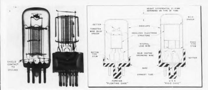
Fig. 5: (1) Overseas 65K7 (1) as seen by X-ray. U. S. tube right. Fig. 6: (r) Excellent shock resistance is provided by tungsten spacer in foreign model
