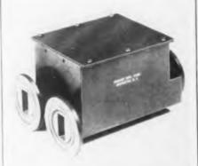
the disconnected member automatically, which provides a termination for the switched member and increases the isolation between arms to better than 60 db. VSWR is less than 1.10 over a 17% bandwidth, and the entire unit is operated by a momentary pulse at 115 v., 60 cps. power. Insertion loss through the connected member is less than 0.1 db. Bogart Manufacturing Corp., 315 Seigel St., Brooklyn, N. Y.-TELE-TECH & ELECTRONIC INDUSTRIES Equalizer Units S
