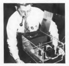
Transistorized 20 watt linear audio amplifier, developed by GE, uses two 6-watt, three 2-watt, and four 1/10-watt experimental transistors. The power transistors will be commercially available within two years
