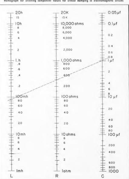
Nomograph for selecting component values for critical damping in electromagnetic circuits
