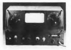
Fig. 1: FM demodulator and deviation meter
