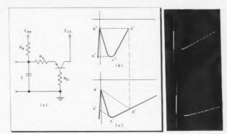
Fig. 4: (1) Circuit (a) and N-curve (b) when R, is much smaller than R. Comparison with N-curve of Fig. 3 (c). Fig. 5: (r) Scope traces of Fig. 4b (a) and 4c (b)
