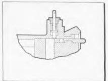
Fig. 6: Diagram illustrating skid type connector
