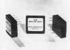
stored digit, and it is capable of working at rates up to 350 KC. Designed for dip-solder assembly, its overall size is  $1_{10}$  x  $1_{10}$  in Nominal shift current is 300 ma. Shift pulse width is 0.5 to 1.5 µsec. Output signal amplitude is 15 v. Epsco, Inc., 126 Massachusetts Ave., Boston 15, Mass.—TELE-TECH & ELECTRONIC INDUSTRIES
