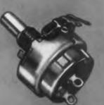
TYPE CC-35, 1 1/8" diameter variable composition resister. Wattage ratings 3/4 wett for resistances through 10,000 alms, 2/3 watt for resistances over 10,000 alms through 25,000 alms, 1/2 watt with 200 alms for resistmum across and terminals for resistances over 25,000 alms. Available with ar without illustrated attached switch and in concentric sheft tandom construction C2-35 as shown above.
