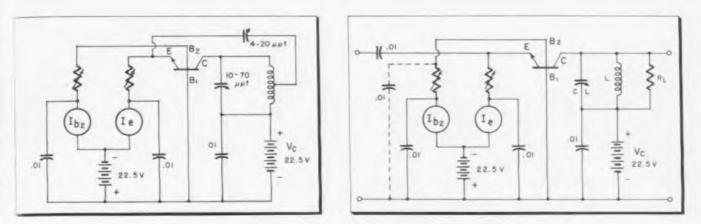
Fig. 1: (I) Oscillator circuit employing tetrode transistor. Fig. 2: (r) Tetrode transistor tuned amplifier
