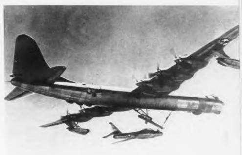
Parasite F-84F about to make contact with retrieving mechanism of RB-36F carrier plane
