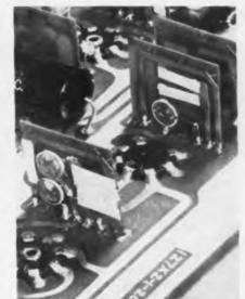
Close-up of "Reliaplate" printed circuit uzed in TV set shows perpendicular construction
