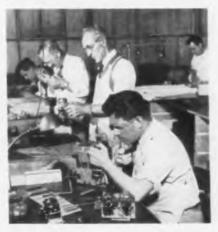
3 The assembly of precision units machined to within 0.0005 in. requires skilled workmanship. Here, jeweler's glass alds delicate adjustment of Computer section
