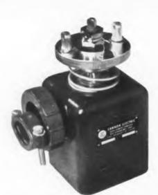
Fig. 1: Type GME ball and detent type latch, hand-wheel actuated engagement, manual lanyard release. One of seven variations of general GME type having 39, 41, 44 and 56 contacts ranging from No. 16 to No. 2
