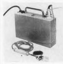
Heart microphone system developed by Altec Lansing includes small mike attached to stethoscope and power supply. Special cardiac conditions may be tape recorded for medical study. Amplifier is also used
