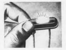
2. INDICATE LIVE CIRCUITS With a little G-E indicator lamp, operators can tell at a glance whether electronic equipment is operating correctly.
