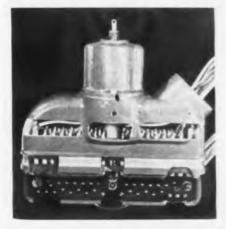
Fig. 8: Cut away view of early GMC type multicontact connector designed for missile use. A number of contacts have been wired.
