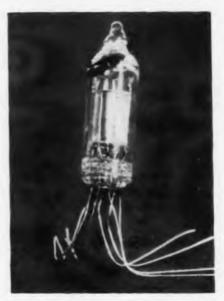
Fig. 8: High temperature subminiature tube
