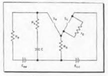
Fig. 8: Equivalent circuit for time analysis
