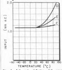
Fig. 3: Full scale deflection, full wave bridge with 0-1 ma, 100-ohm dc meter. (C) 0.080-In. dia. cell; (D) 0.5-In.; (E) 0.187-in.
