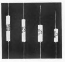
then sealed with silicone cement which precludes moisture coming in contact with the resistance element. The units are supplied in standard watt ratings of 5, 7, and 10 w. and maximum resistance values of 1,000 ohms, 5,000 ohms, and 7,500 ohms, respectively. Tru-Ohm Products, Div. of Model Engineering & Mfg. Inc., 2800 N. Milwaukee Ave., Chicago 18, III.—TELE-TECH ELEC-TRONIC INDUSTRIES
