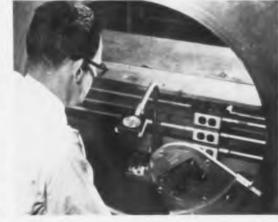
Units mounted on the instrument panel must be checked for magnetic properties. Compass needle indicates effect of computer control being rotated in magnetic field
