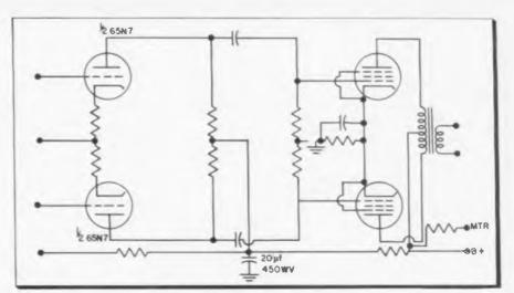
Simple addition of 470 k, resistor from grid to ground cures noisy volume control
