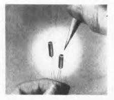
Transistors reported having 1% failure rate in first year of operation in hearing aids
