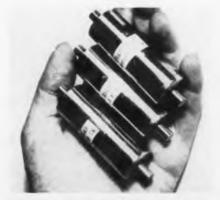
Unusual atomic battery developed by Alexander Thomas of Tracerlab uses radioactive tritium, can produce up to 400 volts at 0.01 to 1.0  $\mu w$ , and has a useful life of 10 to 30 years.
