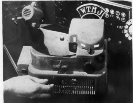
Here is how Station WTMJ, Milwaukee, Wis., keeps an air check of all shows going out over the airwaves from its broadcasting station. Broadcasts are monitored on an Audograph. Paper-thin plastic disc records clearly and economically a full half-hour show on each side. A hundred hours of broadcasting can be permanently recorded and filed in a box only an inch and a half deep and nine in, sq.
