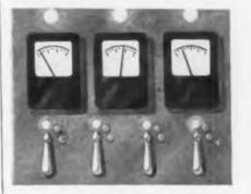
1. FLASH WARNING SIGNALS General Electric filament and neon glow lamps on control panels quickly indicate "trouble spots" in circuit operations.
