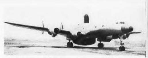
Fig. 4: Flying radar station with bulging radomes is part of extra-early warning system
