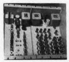
Revised version of recording chassis used in video tape recorder developed by Bing Crosby Enterprises. Complete technical data on p. 77.
