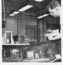
Amplifier being vibrated. All units undergo sustained four-hour vibration test. Prototypes of this equipment have operated for two years without servicing.
