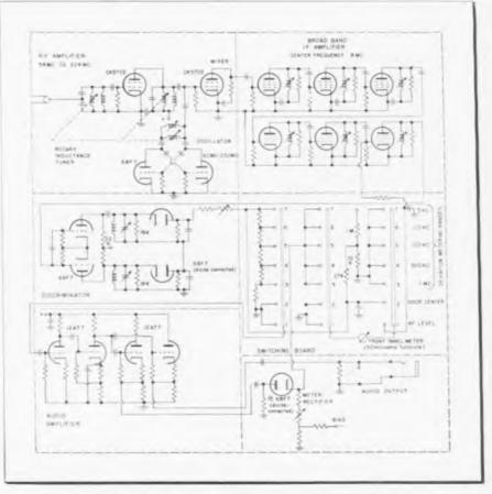
Fig. 4: Circuit diagram of FM demodulator and deviation meter
