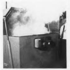
5 Hot salt spray rises from tank subjecting units to 50 hours of corrosive atmosphere. Hermetic sealing and durability of plating and paint are rigidly controlled
