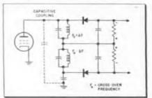
Fig. 2: "Amplitude" type FM discriminator
