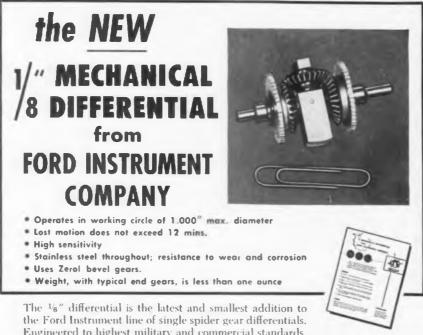
the Ford Instrument line of single spider gear differentials. Engineered to highest military and commercial standards, this highly reliable unit provides extreme accuracy in additive and subtractive operations, while functioning with minimum friction and backlash.
