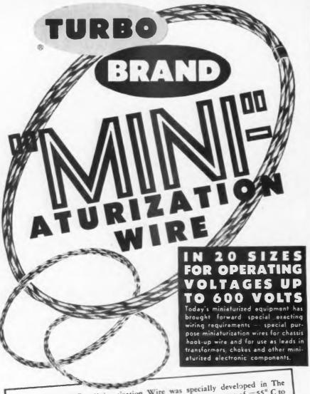
TURBO BRAND Miniaturization Wire was specially developed in The William Brand laboratories to meet a use need within the range of -55° C to +105° C and maximum operating voltage of 600 volts rms. This "mini" wire is available in 20 strandings, ranging from 7/38 to 19/25 and in a graduated scale of AWG sizes from 30 to 12, It is available in both solid and stranded - in solid colors or "candy striped" with 1, 2 or 3 tracers.
