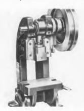
The drive collar is also of steel alloy, heat-treated and ground. Connecting rod and crankshaft bearings are of special bronze alloy. Ram and ram guides are of the over-size length 90° V type. The standard stroke is ¾ in., though a 1 in. stroke is optional at extra charge. Kenco Manufacturing Co., 5211 Telegraph Road, Los Angeles 22. Calif.—TELE-TECH & ELECTRONIC INDUSTRIES.
