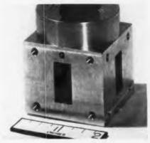
9600 MC. and isolation between output channels is nominally 30 db. General Precision Laboratory Inc., 63 Bedford Road, Pleasantville, N. Y.—TELE-TECH & ELECTRONIC INDUSTRIES.
