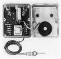
amps. Standard ranges are 0° to 100 300°, or 500°F, and C., but any range between the limits of 200° to 500°C, can be supplied in conjunction with an appropriate resistance bulb from the Fielden list. Sensitivity is 0.1°F, on all ranges Only two vacuum tubes are employed The unit is encased in a 6½ x 7½ x 4 in cast aluminum housing. Fielden Instrument Div., Robertshaw-Fulton Controls Co., 2920 North 4th St., Philadelphia, Pa.—TELE-TECH & ELECTRONIC INDUSTRIES.
