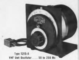
... semi-butterfly tuning circuit varies inductance and capacitance simultaneously to supply at least 80 mw into 50 ohms ... slow-motion drive gives 1% accuracy in dial settings. Price: \$190
