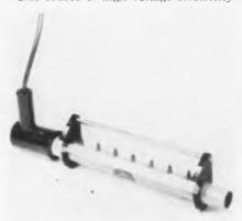
to neutralize static charges during the processing of paper, plastics, paper, etc., the unit combines three grades of "Synthane" with a thermoplastic bar, an aluminum bar, and copper emitter points. The bar is made from Grade XXX tube stock; the brackets from Grade XX black sheet stock. The end connector is Grade C black, and the end plugs are Grade XX black. Synthane Corp., Oaks. Pa.—TELE-TECH & ELECTRONIC INDUSTRIES.
