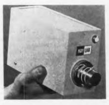
the camera control which consists of an 8 MC video amplifier, horizontal and vertical deflection chassis, and a power supply. Up to 500 ft. of cable can be used between camera and control unit. Kalbfell Laboratories, Inc., P. O. Box 1578, 1090 Morena Blvd., San Diego 10, Calif.—TELE-TECH & ELECTRONIC INDUSTRIES.
