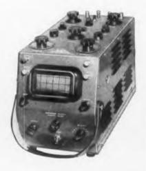
Repetitive or trigger sweep is variable from 5 cps. to 500 kc with 5X sweep expansion. Sweep, marker, and dc. calibrating voltage is available externally. Operates from 50 to 400 cps. at 115 v. ac. Size, 8½ x 6¾ x 13¾ in. Weight, 22 lbs. Waterman Products Co., 2445 Emerald St., Philadelphia 25, Pa.—TELE-TECH & ELECTRONIC INDUSTRIES.
