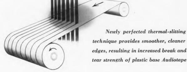
IN THE manufacture of Audiotape, particular care has always been given to the slitting operation, in which the processed tape is cut into reel-size widths. Precision straightline slitting has been one of the reasons why Audiotape tracks and winds perfectly flat and has no fuzzy edges to impair frequency response.
