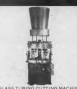
GLASS TUBING CUTTING MACHINE VERTICAL TYPE
