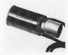
ceivers. Horizontal resistance is 3.59 ohms; vertical resistance, 161 ohms. Horizontal inductance is 0.92 mh; vertical inductance, 53.2 mh. Dimensions: 1% in in diameter by 4 in in length. Weight, approximately 4 oz. Resistor Div., I-T-E Circuit Breaker Co., 1924 Hamilton St., Philadelphia 30, Pa.—TELE-TECH & ELECTRONIC INDUSTRIES
