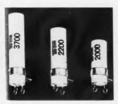
from the winding. The units are supplied in 10, 15, 20, and 25 w. ratings in 1½, 2, 2½, and 3 in. heights, respectively. All are ½ in. in diameter and fit in a ¾ in. chassis cutout. Tru-Ohm Products, Div. of Model Engineering & Mfg. Inc., 2800 N. Milwaukee Ave., Chicago 18, Ill.—TELE-TECH & ELECTRONIC INDUSTRIES.
