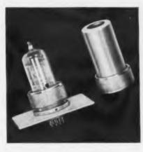
News that is bound to make headlines again for Elco Corporation is its new hermetically-scaled socket for use at high altitudes; and to give complete protection against moisture conditions. Floating contacts of heat-treated beryllium-copper assure complete relief of strain from glass of tubes. The Kel-F body is retained in an aluminum or brass
