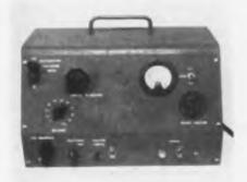
current is applied. These harmonics can be accurately interpreted in terms of v. coeff. Resistance range, 1,000 ohms to 1.1 megohms; test voltages, 0-500 v., power dissipation, 2 w. Supply, 105-135 v. ac., 60 cps. Brunswick Instruments, P. O. Box 813, New Brunswick, N. J.—TELETECH & ELECTRONIC INDUSTRIES.
