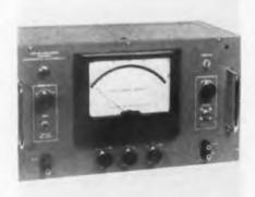
range, 0-36°, 0-90°, 0-180°. Accuracy, maximum error is less than ±3% or ±2° at any range. Input voltage 0.1 v. to 70 v. from 8 cps. to 150 kc. Input power, 115 v. or 230 v. rms, ±10%, 50-60 cps, 60 w. Advance Electronics Co., Inc., 451 Highland Ave.. Passaic, N.J.—TELE-TECH & ELECTRONIC INDUSTRIES.
