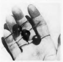
and leads are then assembled and vacuum-impregnated with tropicalized r-f wax. Values of inductance range from 2.2 to 220 mh. Nominal tolerance is ±10% ± one turn. Nominal Q tolerance is ±20%, Core material is Ferroxcube 3C. Curie temperature, 172° C. (342° F.) Weight, ½ oz. Mico Instrument Co., 75 Trowbridge St., Cambridge 38, Mass.—TELE-TECH & ELECTRONIC INDUSTRIES.
