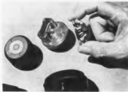
Transistor amplifier being held in hand fits into mouthpiece of a handset or a microphone
