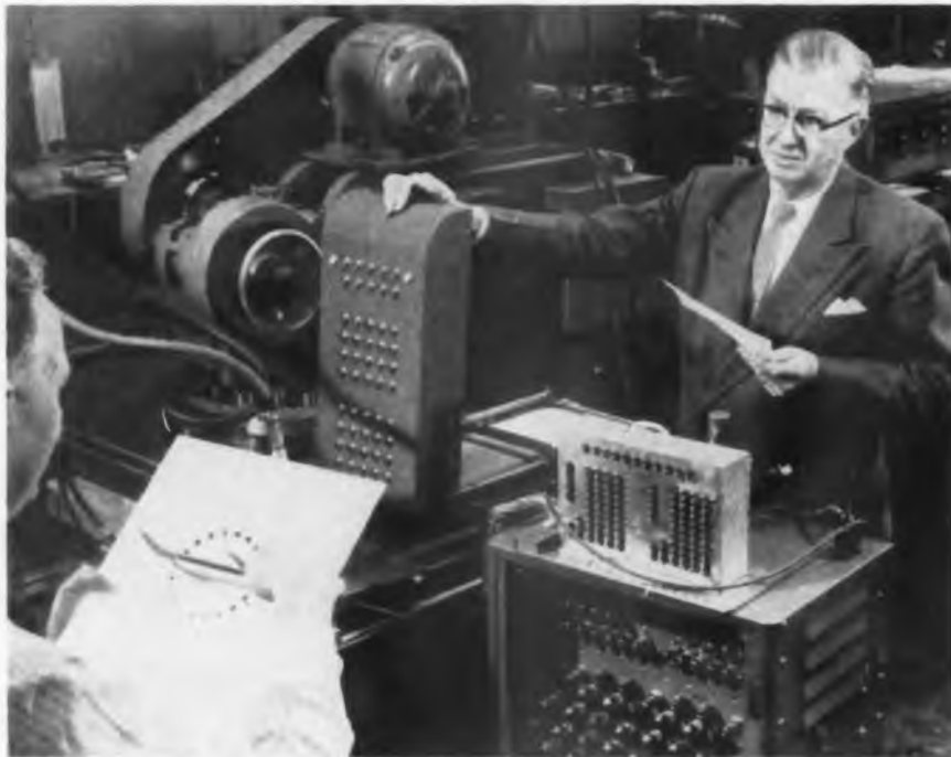
Forerunner of automatic assembly machine for electronic components, punch press controlled by digital computer is extremely versatile. Quick set-ups facilitate small lot production jobs
