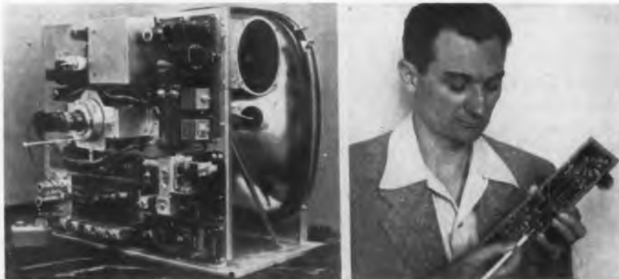
TV receiver (l) with printed circuit chassis. Note concealment of high voltage circuit. Remote control unit turns set on, adjusts volume, and changes channels. Fred Miller (r), Kaye-Halbert Ch. of Engineer, points to circuit etched on copper-phenolic plate
