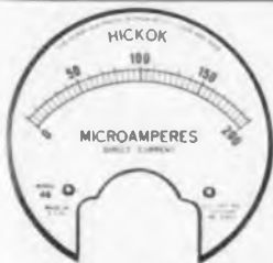
Conventional 100 Degree Arc-Angle instrument showing 0—200 microampere range.
