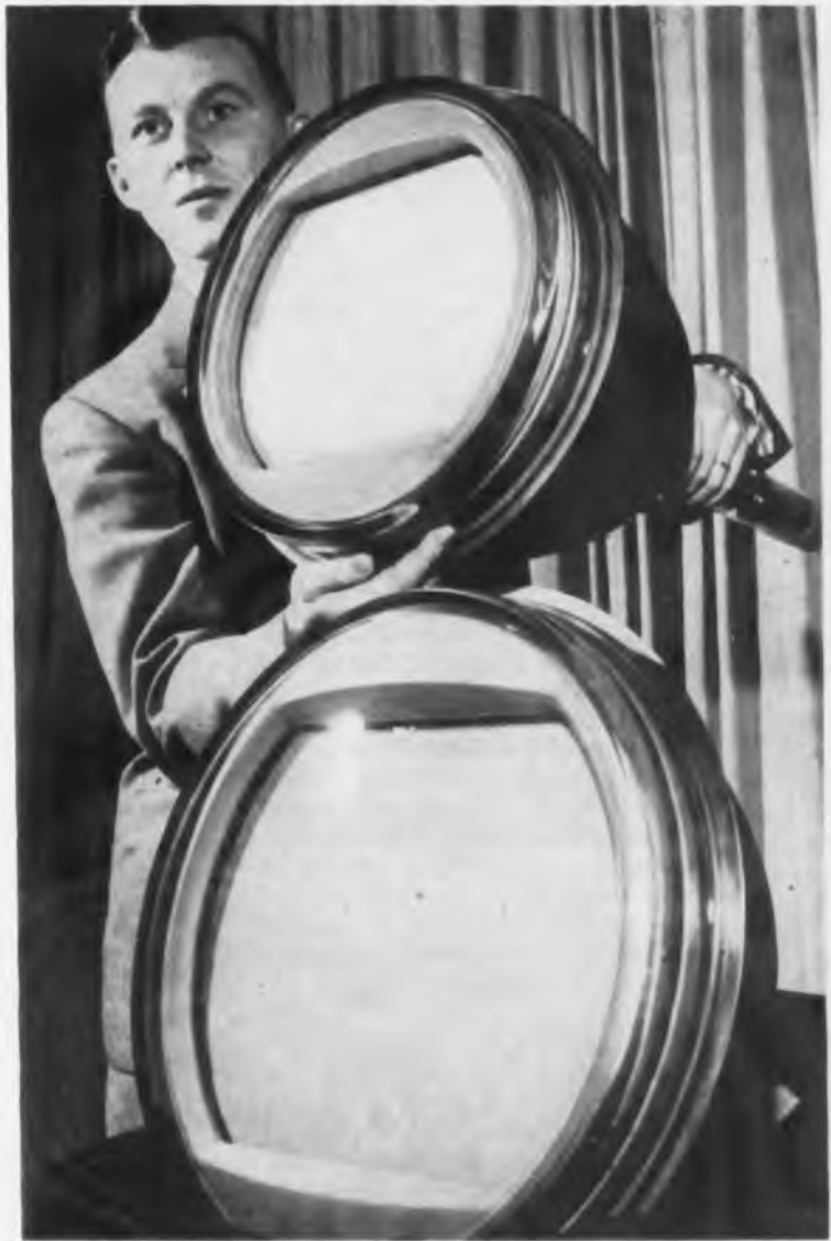
One of the big limitations on the growth of color TV has been the small size of most of the picture tubes available. This obstacle is starting to disappear, and one of the most welcome indications is the announcement of a 19-inch tricolor tube, which RCA plans to make available in limited quantities during the latter half of 1954. Dr. D. Joseph Donahue is shown comparing the 15-inch shadow mask tube with the new model. RCA reports that it is also working on a focus-mask type rectangular tube, 21 inches and very bright, for production next year.
