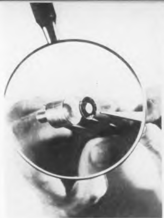
Closeup showing two basic elements of atomic battery. Strontium-90 is at right
