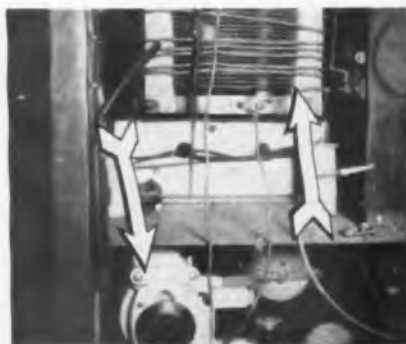
12 turns of No. 14 wire around final tank and tuned provide efficient 2nd, harmonic trap
