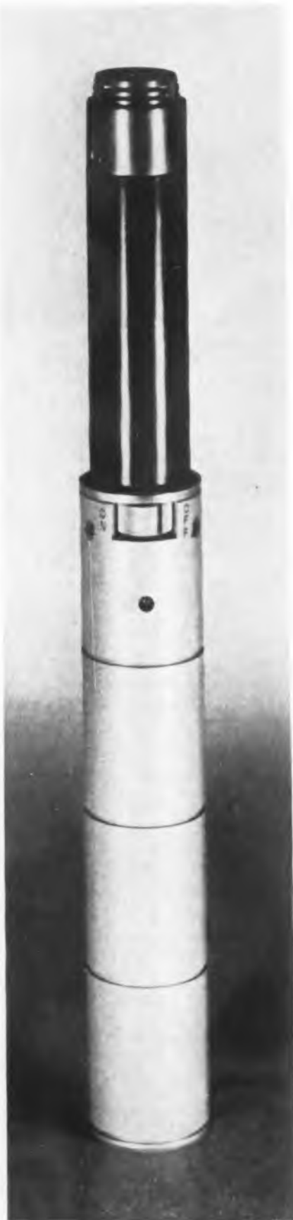
"Vagabond" microphone contains transmitter, antenna and batteries, employs induction system for public address and entertainment work
