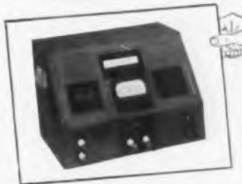
P. R. 5 AUTOMATIC RESISTANCE COMPARATOR permits unskilled operator or automatic set-up to test, grade, sort or match as many resistors a minute as can be touched across two front terminals. Range 100 ohms to 100 megohms. Three scales of deviation from your standard: -5% to +5%, -25% to +30% or -50% to +100%.
