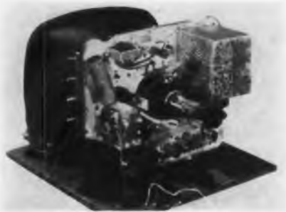
New compact TV receiver employs vertically mounted chassis through which tube projects
