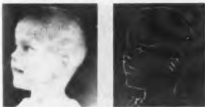
Video picture (l) of photo is changed to outline form (r) by differentiating and rectifying signals, and then clipping to constant level
