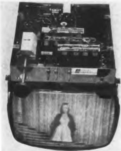
Replacing "rat's nest" wiring with compact modular component sections gives TV new look
