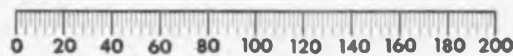
HICKOK 250 Degree Arc-Angle instrument showing same range on a scale approximately 2½ times as long in the same size instrument.
