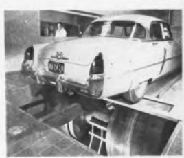
Rear wheels of auto turn drums coupled to dynamometer measuring speed-torque characteristics. Westinghouse electronic controls simulate wind resistance and road grades
