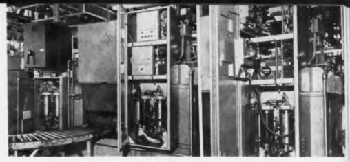
Ring gears are welded to cover with Weltronic welder at Chrysler. At completion of operation, parts are passed along roller track (I) to next station. Welder's electronic controls (r) include sequence timer and phase shift circuit (upper) to control firing of Westinghouse Ignitrons (lower)
