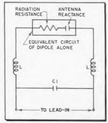
Fig. 3: Simplified circuit of matching network
