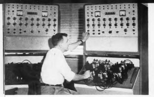
Analog computer recently added to Ford facilities is Goodyear L-3 Electronic differential analyzer
