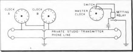
Slave and master clock connections made using one side of private phone line
