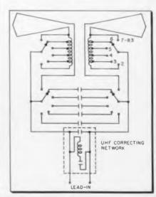
Fig. 4: Double-wafer four-pole selectro switch selects channels in complete circuit
