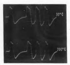
Fig. 6: Temperature effect on gate circuit output is practically same at 30° and 200°C
