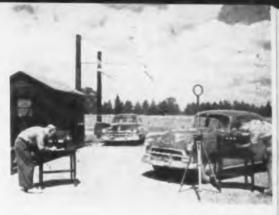
Radiation from ignition system is checked to see if it will cause radio or TV interference on General Motors Proving Grounds
