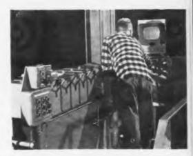
From 300 feet inside Ford stamping pant, operator uses TV screen to observe loading of steel trimming bales into waiting freight cars
