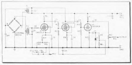
Fig. 13: Output of square-wave amplifier with gain of 100 may be used to modulate escillator
