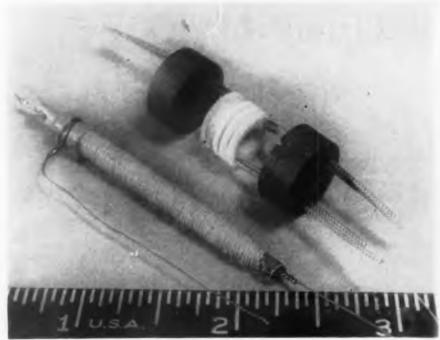
Fig. 2: High temperature delay line and pulse transformer are silicone resin impregnated
