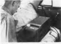
Automobile acceleration during GM road test is measured with the assistance of time-distance oscillograph made by Consolidated Engineering
