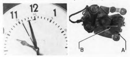
Close up of clock face showing switch lever and lifter. Right setting relays switch
