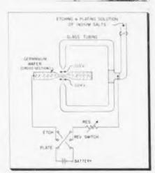
Fig. 3: Electro-chemical etching of germanium water is controlled by polarity switch. Etched area is plated with indium and leads soldered
