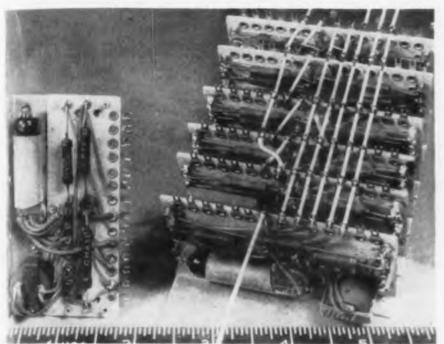
Fig. 3: Component mounting boards are riveted to "L" bracket to form sub-chassis. Note interwiring
