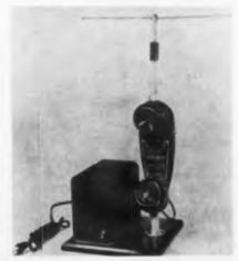
Stewart-Warner's "Portatone" two-way radio is one of first of its kind to receive FCC approval. Unit operates at 465 mc, Transceiver in 10.5 in. case weighs 28 oz. alone; 5.5 lbs. with portable case and battery. Output is 500 mw, and receiver sensitivity is about 12 HV
