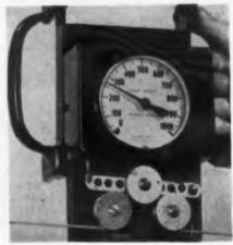
dling tensions of 20 lbs. and more, such as are used in wire and cable making. Free from gear trains, the unit assures freedom from tooth deformation. The same meter is also provided with wider rollers which enable measurement of rayon tow strands, paper strips, plastic tapes, slit film, etc. Tensitron, Inc., Harvard, Mass.—TELE-TECH & ELECTRONIC INDUSTRIES.
