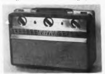
pact, and equipped with retractable legs and a shoulder carrying strap. Its low tape speed (1.87 in./sec.) enables it to record or play for a full hour. Frequency response is 200-4,000 KC. Flutter and wow, ½ of 1%. Distortion, less than 10%. J. C. Warren Corp., 21 Hanse Ave., Freeport, N. Y.—TELETECH & ELECTRONIC INDUSTRIES.
