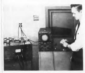
Chrysler engineer adjusts Hewlett-Packard audio oscillator to analyze frequency patterns on DuMont scope. Ampex recorder plays back sounds taped earlier in vehicle test runs
