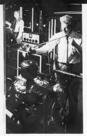
Chryster engine on mount produces sounds which are picked up by mike and taped on Magnecorder. Subjective sound tests aid designers
