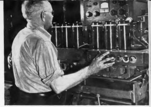
Ultrasonic escillator resonance rapidly checks volume of cylinder head cavities within 0.2 cc accuracy on Ford production line. Previous method required that each cavity be hand-filled with ail
