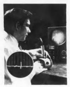
GM-developed Sonigage utilizes ultrasonic resonance to measure thickness and detect intern I flaws. Inset shows vertical trace deflection on CRT for measuring 0.07 in, steel
