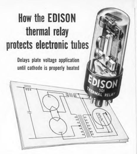
PROTECTION OF CATHODES in electronic tubes, such as thyratrons and gas filled rectifiers, depends on allowing cathodes to reach operating temperature rather than delaying application of plate voltage for a fixed time. A thermal relay, since its operation also depends on attaining a predetermined temperature, is eminently suitable for cathode protection.
