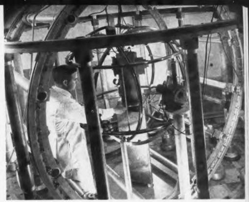
Nature of magnetism is studied within framework which supports Helholtz coils. Current in coils sets up magnetic field to counteract that of earth. Extremely sensitive current control is effected by amplifier which incorporates two phototubes as error detection elements
