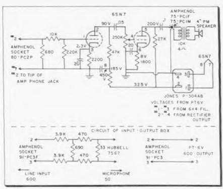
Adding different input and output sockets and monitor speaker to Magnecord PT6-VA
