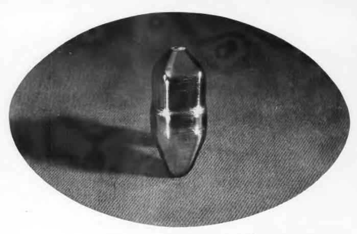
Germanium crystal grown at Bell Telephone Laboratories (life size). It is sliced into hundreds of minute pieces to make *Transistors*. Transistor action depends on the flow of positive current-carriers as well as electrons, which are negative. Arsenic—a few parts per 100,000,000—added to germanium produces prescribed excess of electrons. With gallium added, positive carriers predominate. Latest junction type *Transistor* uses both kinds of germanium in the form of a sandwich.
