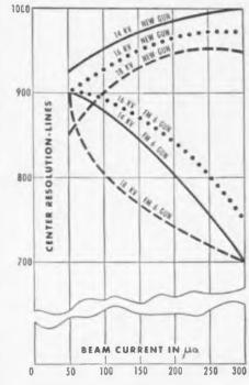
This chart illustrates the ability of the gun to maintain sharp definition despite changes in beam current—relating center resolution to beam current over a range of anode voltages.
