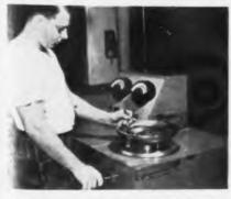
nomically balanced on Chrysler's Tinius-Olsen schine which compares off-center pulse with reference pulse to locate unbalance
