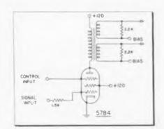
Fig. 4: Circuit of computer coincidence gate
