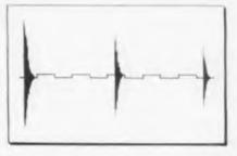
Reflectoscope acreen shows (1) u'trasonic pulse transmitted into material; (c) portion of pulse reflected back from defect; (r) first bick reflection from apposite side of part, Horizontal position indicates depth in work
