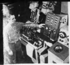
mpulses produced by rotating Ford crank;hafts are stored in electronic memory. With crankhaft stationary, drills automatically remove hetal to bring part to 0.5 oz.-in. perfect dyamic balance
