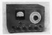
tive output indicator, type 205 will detect phase angle with an error less than 0.1° in communication systems. The unknown signal is delayed until the reading on the output indicator becomes zero or minimum, and the unknown phase angle is read on the dial of the continuously variable delay line.
