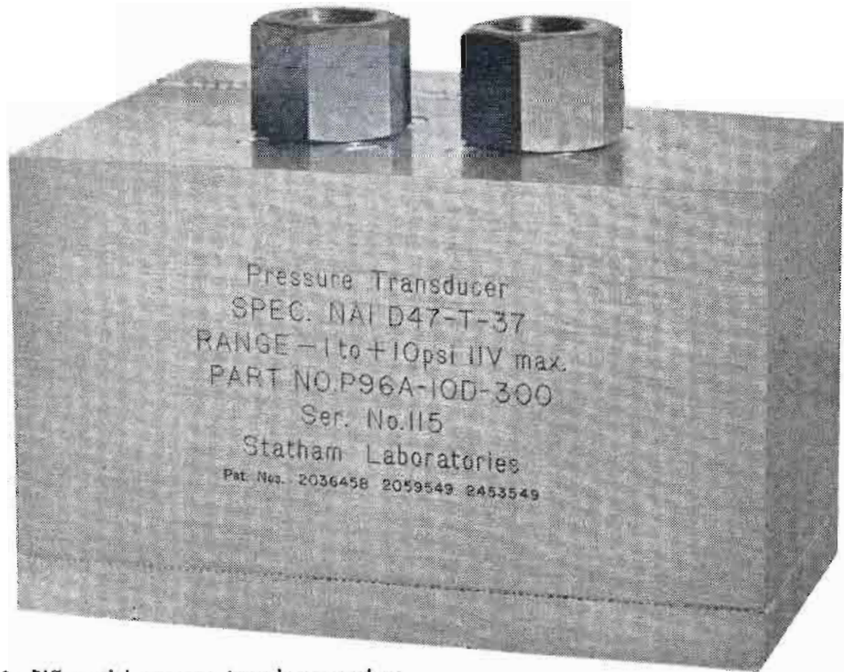
Fig. 2: Differential pressure transducer used as the sensing element
