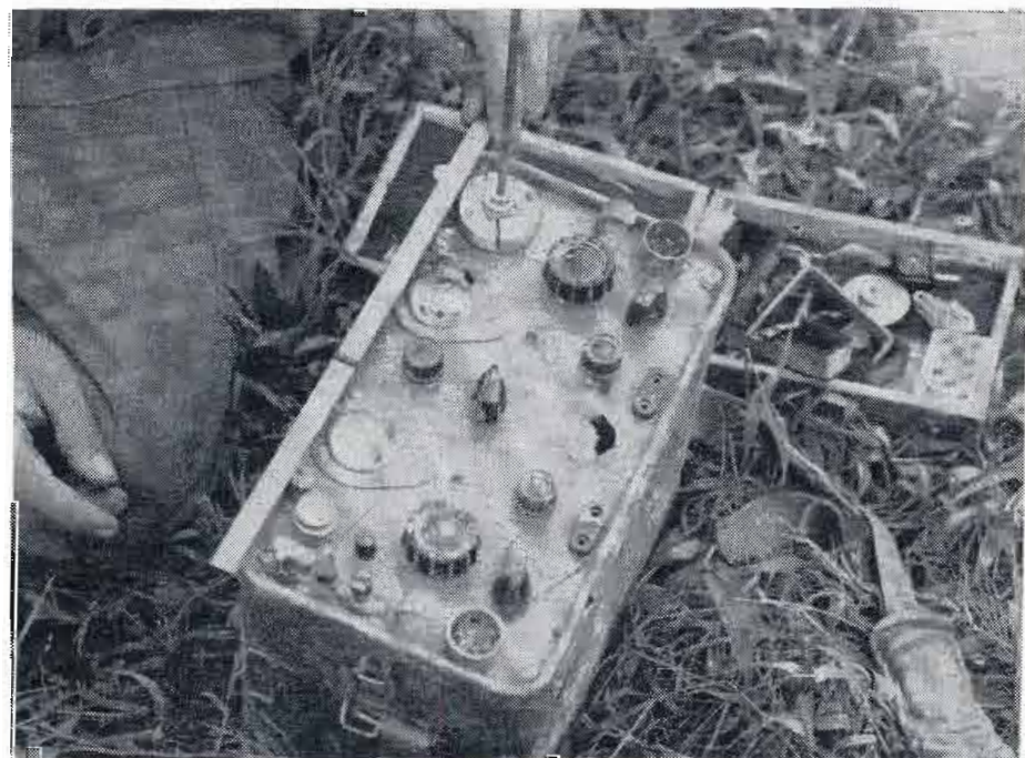
See following pages for photographs of captured radio equipment from Korea. Pictured above is a Russian field radio set.—U. S. Army photograph
