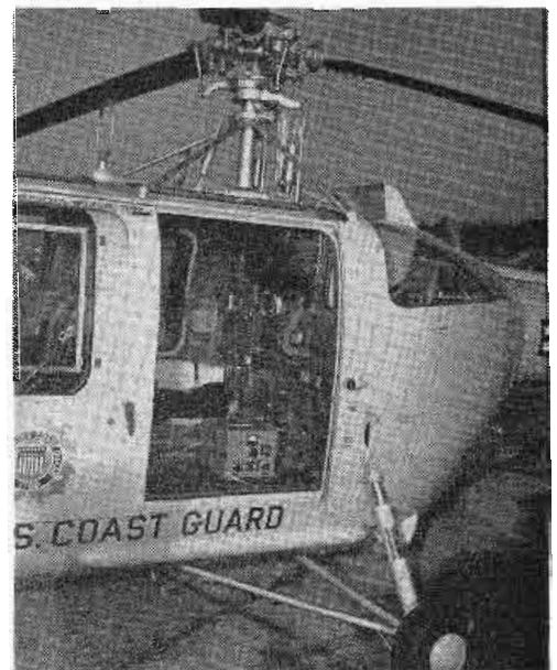
Raydist system installed in Coast Guard helicopter permits craft to be "talked down" by ground operator. Installation requires only one transmitter
