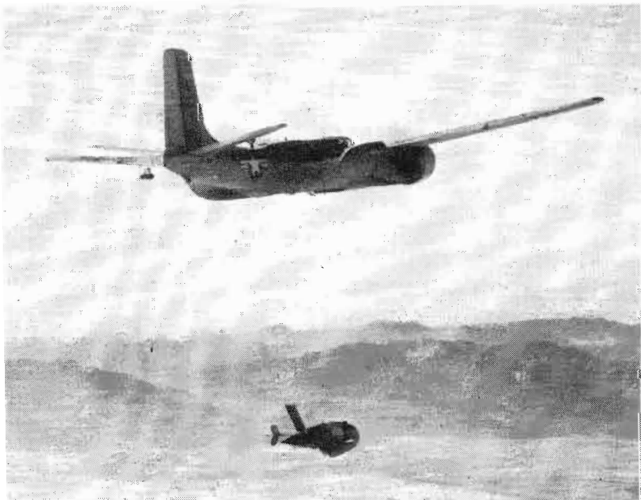
Near Alamogordo, N. M., the Ryan Q2 pilotless target-plane is launched from its “mother” B-26 and proceeds under radio remote control from the ground installations of the Holloman Air Development Center
