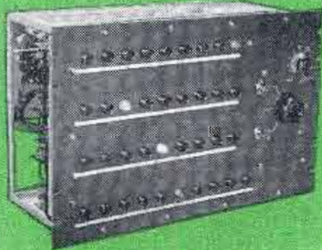
NINE CHANNEL SWITCH UNIT
