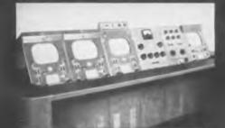
TC-4A with master monitor unit, preview mention unit, and two comerc control units some live and one film or two film). If desired, pections can be arranged United to the Control of the weighted provided to the control of the contr
