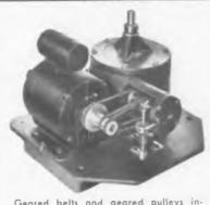
Geared belts and geared pulleys insure accurate timing for all 3 speeds.
