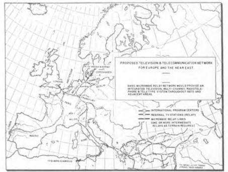
Map showing how principal cities of Europe can be linked in a microwave relay system that could provide an international television service along with both civilian and military communications facilities. Stations would be placed on mountain peaks and designed to operate unattended. Helicopters to be used to provide any necessary services. This system can also be integrated with a Trans-Atlantic TV System (see Aug. issue editorial and page 66, this issue). Full details in Tele-Tech next month.
