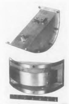
USAF Specification No. X-7196, and is particularly suitable for F-80 type airplanes. This antenna weighs 12 oz. and has the following dimensions: overall length, 7.75 in.; overall width, 4 in.; overall width, and width of element, 8.24 in.; and width of element, 1.75 in.
