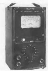
KC. The new meter has been extended to 6 MC. The instrument has a six-state amplifier with a novel ac regulated power supply. It measures voltages between 70 and 1000 v — Millivac Instrument Corp., 444 Second St., Schenectady 6, N. Y.—TELE-TECH
