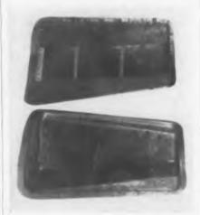
is in the experimental development category. it operates over the frequency range of 108 through 122 MC, and is horizontally polarized. RG-8/U or similar 52 ohm coaxial cable is used in connecting the antenna to the radio set. One antenna is installed on each side of the nose of the F-90 aircraft and the two are fed in phase opposition through a balun, thus obtaining 360°
