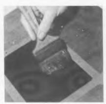
Fig. 3: Sensitizer is applied to film with a very soft camel hair brush, and then dried
