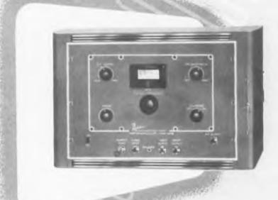
he Type 907 is a fundamental oscillator which can be swept in frequency over a band of not less than 10 mc/s for a center frequency of 35 mc/s. The sweep width is greater than 20 mc. for carrier frequencies above 60 mc/s. Output is continuously variable over a voltage range of 10 microvolts to 1 volt. Other features include a video blanking circuit for providing a true horizontal zero base line and a terminal for inserting external frequency markers.
