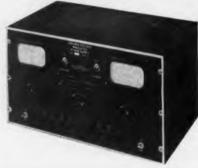
0.5% regulation at loads from 0 to 200 ma. At the users wish, the two outputs may be paralled to double the output current or seriesed to double the output voltage. Also
