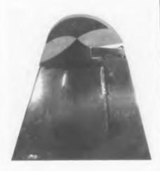
early part of 1946 to satisfy the requirements of a broadband antenna covering the frequency range of 100 to 400 MC and could be used with the following current equipments: VMF Command Equipment, IFF Equipment, and UHF
