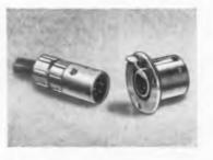
There are 12 items in the XL line. Insert arrangements available: 3-15 amp. contacts, 4 - 10 amp, contacts - working voltage 250 volts. Zinc and steel plugs with bright nickel finish are standard. Satin chrome finish also available on steel plugs.
