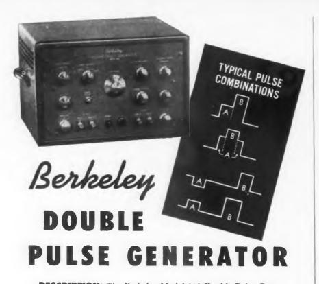
**DESCRIPTION:** The Berkeley Model 903 Double Pulse Generator is a general-purpose laboratory instrument that produces either single or paired pulses. Pulses are individually variable in width, amplitude, and spacing. Pulse polarity is individually selectable. Separate connectors provide impedance levels of 50 or 1,000 ohms for each pulse output.
