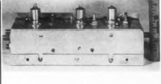
Fig. 7: (L) Circuit diagram of typical receiver front end. Using 26.5 volt tubes such as type 5908, it produces gains as high as 28 with bandwidth of 0.5 MC. Fig. 8: (R) Photograph of receiver front end showing size
