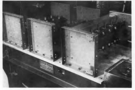
Fig. 5: Photo of machine used in conducting sampling tests for mechanical fatigue
