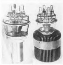
erate up to 220 MC. Tubes are compactly constructed with thoriated tungsten filament, disc type screen grid seal to minimize in-ductance, and two control grid pin con-nections with low capacitance and induct-ance.-Amperex Electronic Corp., 25 Wash-ington St., Brooklyn 1, N. Y.-TELE-TECH.
