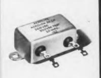
Series P30ZN Aeroleneimpregnated metallizedpaper capacitors housed in "bathtub" metal cases with vitrified or glass terminal seals. Operating temperature range of -55 C. to +100 C. at full rating; to +125 C. at 75% of voltage rating. Capacitances available from 0.1 mfd. up to 15.0 mfd. at 150 V. D.C., and up to 3.0 mfd. at 600 V. D.C.
