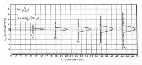
Fig. 3: Photo of diffraction pattern of 10 MC waves in water shawing effect of source length
