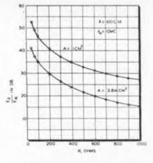
Fig. 4: Calculated midband loss as function of R for 10 MC shear wave delay line 100 cm long
