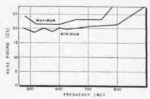
Fig. 13: Converter noise figure response
