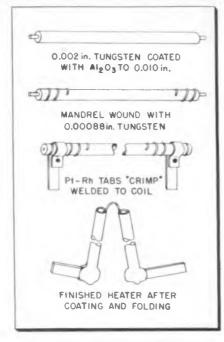
Fig. 1: 26.5 volt heater made by crimp welding to reduce heat transfer to coil wire
