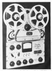
response is  $\pm 2$  db from 40 to 15,000 cps at 15 in, sec., and  $\pm 2$  db from 50 to 9,000 cps at 75 in./sec. Signal-to-noise ratio is 55 db and harmonic distortion is 2% at zero VU. Flutter and wow is 0.1% rms at 15 m./sec and 0.2% at 7.5 in./sec., with play-back timing accuracy  $\pm 0.2$ %.—Berlant As-sociates, 4917 W. Jefferson Blvd., Los Angeles 16, Calif.—TELE-TECH.
