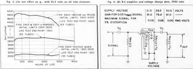
Fig. 4: (R) R-C amplifier and voltage change data, 5905 tube
