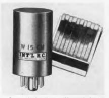
to fit standard sockets. All standard tube mountings are available. The unit illustrated (no. W15CM) is rated at 390 v. rms input; 550 v. peak inverse; 120 ma., 160 v. dc out-put at 35° C. ambient. Half wave and bridge circuits are also available—International Rectifier Corp., 1521 E. Grand Ave., El Se-gundo, Calif.—TELE-TECH.
