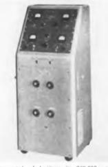
to one part of helium in 290,000 parts of air, or a leakage flow of less than 0 00001 standard cc.hr. presence of a leak is indi-cated by meter deflection or increase in pitch of an audio note. The unit is 22 in. wide, 21 in. deep, 52 in. high and weighs 350 lbs. Power consumption is about 800 watts at 115 v., 60 CPS. No cooling water is required. — Vacuum-Electronic Engin-cering Co., 756 Third Ave., Brooklyn 32, N. Y. — TELE-TECH.
