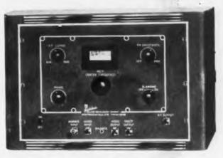
The Type 907 is a fundamental oscillator which can be swept in frequency over a band of not less than 10 mc/s for a center frequency of 35 mc/s. The sweep width is greater than 20 mc. for carrier frequencies above 60 mc/s. Output is continuously variable over a voltage range of 10 microvolts to 1 volt. Internal blanking circuits provide a "true zero" base line for an oscilloscope display.
