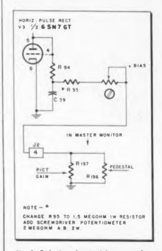
Fig. 3: Reduction of potential across pedestal and gain controls by use of resistor
