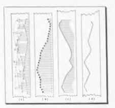
Fig. 4: Four types of commutated channel presentations; (A) unseparated sub-carr.er; (B), (C) and (D) after automatic separation
