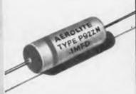
Series P92ZN Aeroleneimpregnated metallizedpaper capacitors are modified plastic-tubular duranite-end-sealed units in paper cases Operating temperatures of -30 C. to -100 C 200, 400 and 600 V. D. C. 0.01 to 2.0 mfd.
