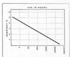
This curve results from actual life tests of capacitor networks under pulsing conditions in a radar modulator. Service life, for varying values of "K", starts at 2 tenths of one hour and stretches out to something over 40,000 hours (more than  $4\frac{1}{2}$  years of continuous operation at full-rated voltages.)
