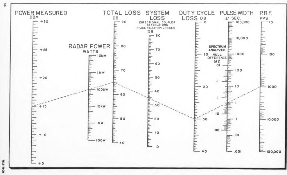
Nomogram for Peak Power Output when Pulse Width, Repetition Frequency, System Loss, and Average Power are Known
