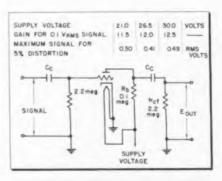
Fig. 2: R-C amplifier using 5904 tube shows stable gain over wide range of voltages
