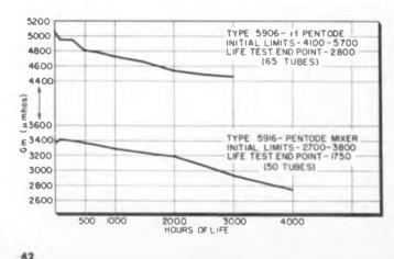
Fig. 9: (L) Effect of life test on  $g_{\rm m}$  of two tubes with 26.5 volt heaters and 100 volts on plate and screen. Fig. 10: (R) Cumulative life failures of subminiature tubes. Measurements taken at 30° C ambient temperature
