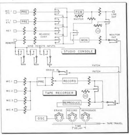
One advantage of this reverberation generator is the fact that one has an exact copy of the whole process from microphone or turntable to line output for audition or re-use. One disadvantage of the system is the limit of running time. For example, if 7.5 in. reels are used the tape will run for 30 minutes at 7.5 in/sec and 15 minutes at 15 in/sec. At KSTL we have a Raytheon studio console and a Presto PT-900 tape recorder.
