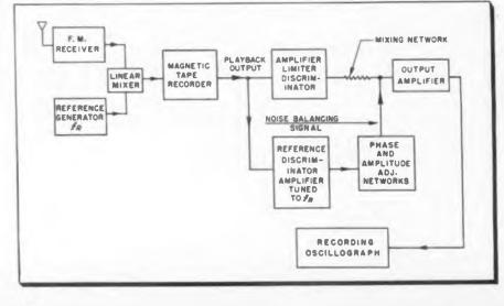
Fig. 7: Compensation system mixes reference signal with incoming signal before recording on tape
