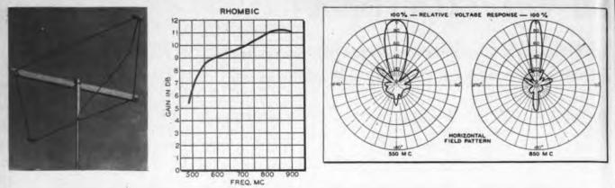
Figs. 11-13: Physical appearance, gain vs frequency curve, and horizontal field pattern directivity for rhombic antenna
