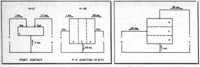
Fig. 7: Comparison of transistors
