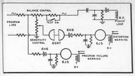
Transmitter quality monitor provides distortion indication through audio harmonics
