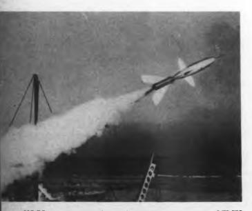
NACA two-stage radio-guided interceptor missile MX-570 taking off at Wallops Island test station, Langley Field, Va.
