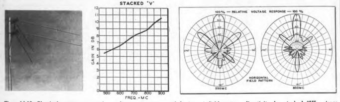
Figs. 14-16: Physical appearance, gain vs frequency curve, and horizontal field pattern directivity for stacked "V" antenna
