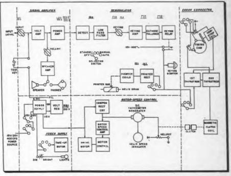
Fig. 8: Block diagram of recorder electronic assembly which consists of signal amplifier and demodulator shaper circuits, motor helix speed control, automatic synchronization or error corrected circuit and a power supply
