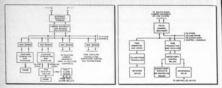
Fig. 4: Time division multiplexing at a microwave station
