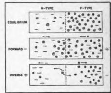
Fig. 4: Rectification by a P-N Junction
