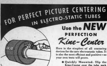
MORE EFFICIENT Rings are closer to deflection yoke (the ost effective operating area) and to the tube neck. They are stabil-ized magnetically.
