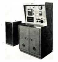
furnace control instrumentation. It has an F-4 modified furnace with a 4<sup>3</sup>/<sub>4</sub> in. ID Kanthal-wound doublecore of 5-zone construction. Arcweld Manufacturing Co., Grove City, Penna.
