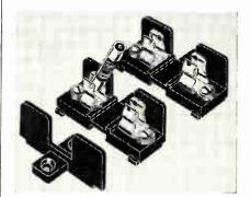
single pole blocks interlock and each unit is locked in place by a single screw. Additions may be made at either end. Poles may be added or removed without disconnecting terminal leads on other units. Each fuse may be a circuit disconnect. Clips permit raising one end of the fuse to a right angle position to the block. Bussmann Mfg. Div., McGraw-Edison Co., University at Jefferson, St. Louis 7, Mo.
