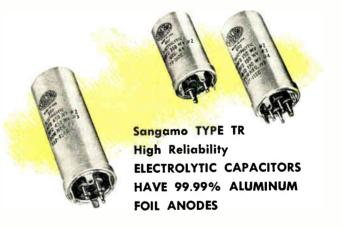
The use of 99.99% high purity aluminum anodes in Sangamo Type TR Twist-Tab Electrolytics, surgically clean papers, and a highly effective end seal gives these capacitors excellent operating life and superior electrical characteristics. They are designed to operate in a temperature range from  $-20^{\circ}$ C to  $85^{\circ}$ C and are available in ratings from 3 to 450 volts D.C.
