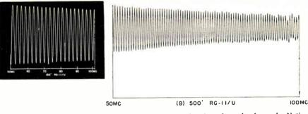
Fig. 7: (A) Ripple pattern from 150 ft. of RG11/U cable, shorted at the far end. Notice that the pattern is about the same as that for 66 ft. piece of RG59/U, in Fig. 6(B). The attenuation of RG11/U is about one-half that of RG59/U for a given length; so doubling the length just about cancels the attenuation improvement due to the larger cable. (B) shows the pattern from about 50 ft. of RG11/U showing the great reduction in ripple height at this length.
