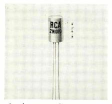
microphone preamplifiers, and hearing aids in which low noise factor is important. Designed to operate from extremely small input signals, it has a noise factor of 5 db with a generator resistance of 1000 ohms and an integrated noise bandwidth of 15 KC. Typical small-signal current gain is 35. Alpha-cutoff frequency is 2 MC. Semi-conductor and Materials Div., Radio Corp. of America, Somerville, N. J.
