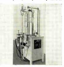
led, and an arrangement to rapidly center the process bar within a straight walled quartz tube supported between gas-tight, water-cooled end plates. Lepel High Frequency Labs., Inc., Woodside, N. Y.
