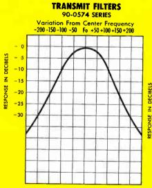
ATTENUATION: (Typical) Insertion power loss = less than 5db Band width @ 3db relative: ±55 CPS Band width @ 25db relative: ±170 CPS
