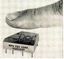
and subsequently an 8.0  $\mu sec.,$  300 ma shift pulse. It is encapsulated in an epoxy compound and occupies 0.2 cu. in ESC Corporation, 534 Bergen Boulevard, Palisades Park, New Jersev.
