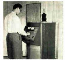
waist high panel sloped for easy reading. Two 41/2 in. meters on the panel indicate output voltage and leakage current. Safety features are incorporated. The output test potential is continuously variable from zero to maximum and indicated by metering directly in the final output. Associated Research, Inc., 3777 W. Belmont Ave., Chicago 18, Ill.
