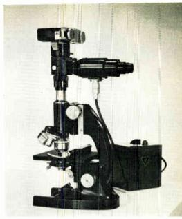
In the Bausch & Lomb U-V Photo-Microscope, the Ultrascope is mounted at right angles to the usual viewing axis. A camera is in position to record the image, under ultra-violet light, which can now be focussed visually.
