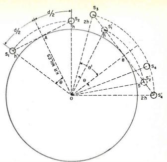
Fig. 6: Satellite communication geometry with the earth as a relay sta-
