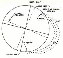
Fig. 3: Radio waves at 10 KC are conducted in this rare duct of about 2000 km dia.
