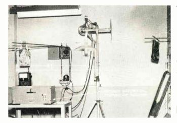
Fig. 5: Solar radiation test in unventilated, sealed room.
