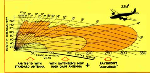
300% increase in coverage and warning time of type AN/TPS-1D radar results when Raytheon's new QK-653 Amplitron and 40-ft. high-gain antenna are added to the system. With other radars of more limited range, improvement factor may be even greater.
