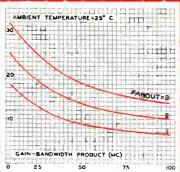
Curves illustrate typical delay time per stage vs. gain-bandwidth product and fanout for the switching circuit shown belaw.
