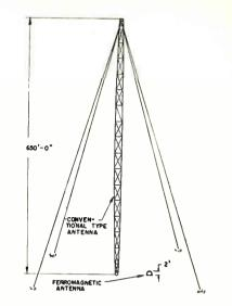
Fig. 7: A comparison of the ferromagnetic antenna with the conventional type.
