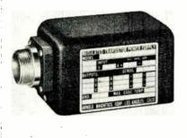
vdc; output voltage: 26 and 115 vac standard. Output frequency of 400 CPS is standard, with 1200, 1500 and 2000 CPS available. Output power: 40 va. Operating temperature range:  $-55^{\circ}$ C to  $+71^{\circ}$ C. Three standard terminations are available—A/N connector, wire-lead pigtail, and solderlug terminals. Arnold Magnetics Corp., 4613 W. Jefferson Blvd., Los Angeles 16, Calif.
