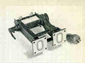
One of several unclassified designs in advanced development, this 100-watt CW tube features a multiple helix structure, involving four parallel beams for higher power output over a wider bandwidth. Frequency range is 7.5 to 11.3 kmc, with 25 db gain minimum.
