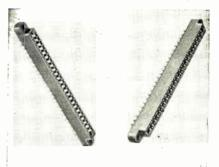
having 0.156 centers. They accommodate Class 1 (broad limits) tolerances on NEMA nominal 0.062 in. laminates. Maximum contact resistance is 4 mohm measured on a 0.054 in. card after insertion of a 0 074 in. card. The double side card receptacle maintains a minimum of 1 oz. per contact on a 0.054 in. thick card after 1000 insertions of a circuit board having a thickness of 0.074 in. Methode Mfg. Corp., 7447 W. Wilson Ave., Chicago 31, Ill.
