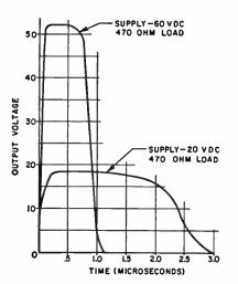
These are typical output curves for the "1PB600" Series "One-Shot" switch, illustrated above.
