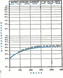
LEAKAGE CURRENT vs. THME AT 125° C "KEMET" K5H30 SOLID TANTALUM CAPACITOR (Average of Typical Capacitors)
