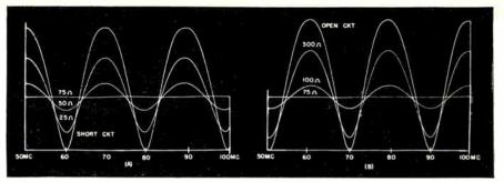
Fig. 8 (above): Patterns from several resistive terminations: when they are (A) lower than the characteristic impedance; (B) higher than characteristic impedance.
