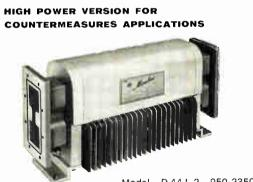
Power average – 400 w Peak – 10 kw Insertion loss (max) – 1.0 db Isolation (min) – 10 db  NARROW BAND-Improved characteristics for Radar
