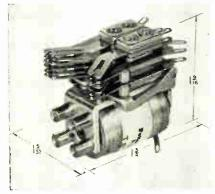
as 100 mw per movable arm and can be furnished to operate on voltages up to 110 vdc. It will switch up to 4 a. at 155 v. 60 CPS, resistive loads. It is mounted with tapped #4-40 studs on  $\frac{3}{8} \times \frac{3}{8}$  in. centers, and measures  $1\frac{3}{4}$  in. long x 1 5/32 in. wide x 1 9/16 in. high. Weighs app. 3 oz. Relays are furnished with pierced solder lugs or taper tabs. Potter & Brumfield, Inc., Princeton, Ind.
