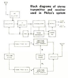
FM signals is accomplished in a manner that permits any standard AM receiver to pick up and reproduce, distortion-free, balanced monophonic sound, while a stereophonic receiver—with separation circuit and multiple speakers will convert these AM and FM signals into true stereophonic sound.
