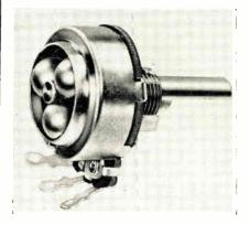
rotation approximately 4000°. Type VA-45 is 15/16 in. dia., ¼ to ½ w. Resistance range is 250 ohms through 10 megohms (linear taper). Voltage rating across end terminals is 500 vdc and voltage rating bushing to terminals 1000 volts ac for 1 min. hi-pot test with 750 vdc operating maximum. Chicago Telephone Supply Corp ration, Elkhart, Ind.
