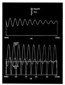
sipate energy. so the wave is reflected from a purely reactive termination at full amplitude. Its phase is shifted depending on the magnitude of the reactance relative to  $Z_0$ . Thus the ripple pattern obtained with purely reactive terminations has the same amplitude as with an open or short circuit, but the minima and maxima are shifted in frequency. Fig. 9 (A) shows the patterns obtained with two sizes of capacities compared with open and short circuit patterns.
