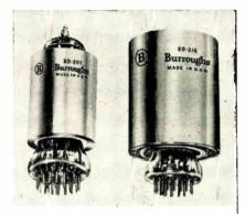
switching tubes. Dimensions are reduced by 35%. They may be used in direct contact with each other. They are 10 position tubes for distribution, counting, coding and decoding, sampling and conversion. Each tube may replace 20 or more transistors or other components. They can be arranged to switch in sequence or at random, can be preset to any position, and interconnected as distributors to any number of positions. Burroughs Corp., Electronic Tube Div., P. O. Box 1226, Plainfield, N. J.
