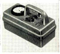
measurements by regulatory agencies. The unit has two controls: a range switch and a zeroing knob, and a 3-in. meter. The zero knob is protected against inadvertent movement. High impedance circuitry is hermetically sealed and range switching is performed in the low impedance portion of the circuit. The Victoreen Instrument Co., 5806 Hough Ave., Cleveland 3, Ohio.
