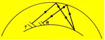
In the other case, transmitted power can be scattered back along the path transmitter—ionosphere ground—ionosphere—receiver, as show in Fig. 2.
