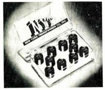
all transformers are in a 1-to-1 ratio. On 6, the 3rd winding is in a 1-to-1 ratio with 3 taps, and on 4, the 3rd winding is in a 1-to-5 ratio with 3 taps. A combination of 20 different ratios is possible. Designed for blocking oscillator circuits, computer circuits, and interstage coupling. High permeability, low-loss cores are used. They plug into a standard miniature 9 pin tube socket. New York Transformer Co., Alpha, N. J.
