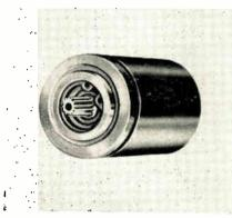
tapped winding for transistor use, and develops 0.33 oz. in stall torque in a standard size 8 BuOrd frame. The 2-phase winding is 26 v. on the fixed phase and the center-tapped control phase is 20/0/20 v. Power input is 2.7 w/phase at stall; operating temperature range  $-55^{\circ}$ C to  $150^{\circ}$ C; speed at max. power output 3500 RPM; rotor moment of inertia 0.65 gm. cm<sup>2</sup>, and weight 1.6 oz. Meets Mil Specs. Induction Motors Corp., 570 Main St., Westbury, N. Y.
