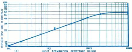
Fig. 5 (above): Noise level of the amplifier is a function of the input termination.
