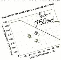
age. Units exceed MIL-T-19500A. High dissipation is realized through direct contact between the header and the active element. Texas Instruments Incorporated, P. O. B. 312, Dallas, Tex.
