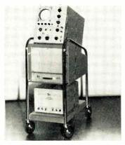
attenuation of 10% of the input signal per step; has a 72-ohm characteristic impedance. Vertical-input system withstands crest voltages of 3 kv of the standard 1.5 by 40  $\mu$ sec surge testing waveform. It has 11 calibrated sweep rates: from 20 m $\mu$ sec/cm, to 50  $\mu$ sec/cm. Sweeps can be triggered internally or by external signal and can be operated singleshot. Tektronix, Inc., P. O. Box 831, Portland 7, Ore.
