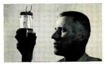
Seawater and sediment in bottle characterize ocean floor. Test sample of insulation on coiled wire is checked for bacterial attack by conductance and capacitance tests.
