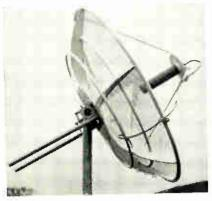
tion. Gain is 23 to 26 db over an isotropic source, nominal beam width is 8° to 14°. Frequency range is 940-980 MC. VSWR of the complete antenna is less than 1.3. Azimuth adjustment is 360°; elevation adjustment 0-90°. Used for orbital and into-space telemetering or TV-Studio Transmitter Links (STLT) by feeding the dish with a 1990-2110 MC feed. Technical Appliance Corp., Box GC 38, Sherburne, N. Y.
