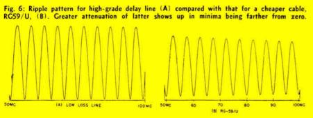
tained by connecting a short circuit across the end of the line. This reverses the phase of the reflected wave so that the two components are 180° out at the short, and produce zero voltage there. At the detector, this produces a minimum at zero frequency (effective line length 0). a maximum at 25 MC, (reflected wave shifted 180° having travelled  $\frac{1}{2}$  wavelength extra), and a minimum again at 50 MC.
