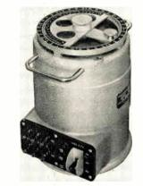
standards, wattmeters, power-factor indicators, induction relays, and instrument transformers. Direct-reading scales on the instrument, are calibrated in deg. for the electrical angle of displacement and in corresponding power-factor values. True-power-factor can be read directly. Ratings are: 1000 va continuous duty; input 120/ 240 v.; output, 120 or 240 v, 3 phase. Knopp Inc., 1307 66th St., Oakland 8, Calif.
