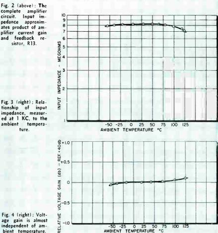
the current gain is a function of transistor parameters, the input impedance can be expected to be a function of ambient temperature. Fig. 3 is a plot of the input impedance at 1 KC vs. the ambient temperature.
