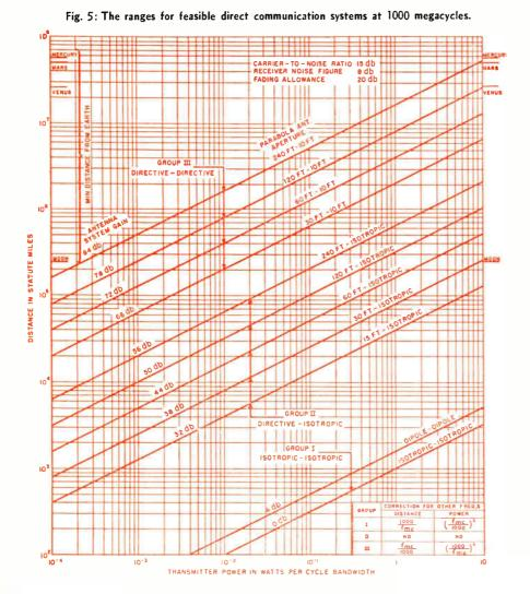
IN the present study, a fading margin of 20 db will be allowed in all cases. For space-to-space communication, this margin may be too severe but for either spaceto-earth or earth-to-space communications, this margin may not be enough. Fading may be reduced by circularly polarized antenna systems or diversity techniques.
