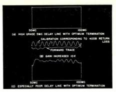
Fig. 17: These traces show the extremes that may be encountered in cable reflections.
