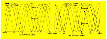
The impedance of a load giving a minimum at the same frequency as a short circuit is resistive and lower in resistance than  $Z_o$ .
