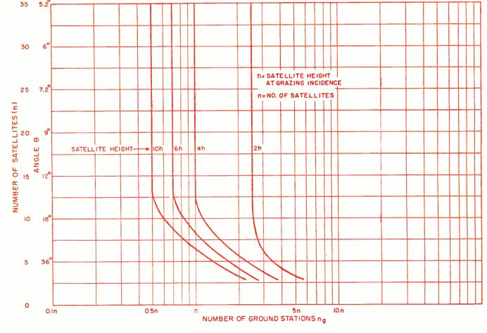
Fig. 8: The relationship of the number of ground stations to the number of satellites, orbitting at different heights, for relay purposes.
