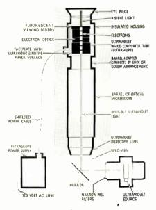
This simple drawing illustrates how specimens under ultraviolet light may be studied directly. The ultrascope unit, including power supply, is priced at \$1500; it replaces a TV system costing \$15,000.
