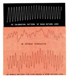
Fig. 18: Accurate measurements are made difficult by irregularities in delay line.
