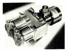
$-65^{\circ}$ F to  $+200^{\circ}$ F. Compressor capacity is 0.025 ppm at 30 psia outlet with 7 in. Hg. absolute inlet pressure. For vacuum it will reduce 800 cubic volume from 29.92 in. Hg. absolute to 0.5 in. Hg. absolute in 2 min. with outlet discharging to sea level. Motor is  $\frac{14}{4}$  HP, 400 CPS, 3 phase, 207 v. and is fan cooled. Great Lakes Manufacturing Corp., 4223 Monticello Blvd., Cleveland 21, Ohio.
