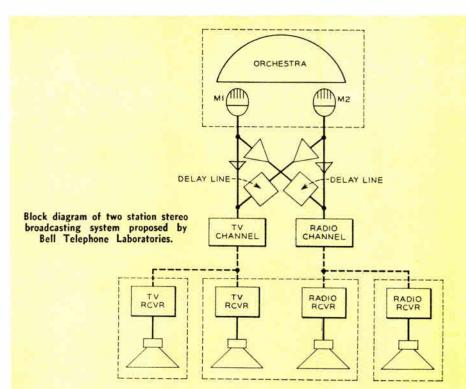
delayed several milliseconds (thousandths of a second) in one, the listener will "hear" the sound as if it came only from the speaker from which he heard it first. He will judge the second loudspeaker to be silent. The amount of the Precedence Effect depends somewhat on the length of delay builtin; at 10 milli-seconds, the sense of direction for an average observer is as if the echo were 8 to 10 decibels softer than the sound preceding it.
