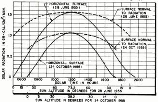
Fig. 4: Incident solar radiation recorded on surfaces at Dugway, Utah.
