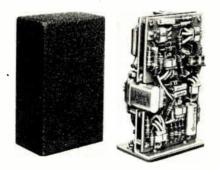
ings are 2a at 28vdc. Repeatability of trip point is  $\pm 1$ mv. and overload capacity is 1000 times rated sensitivity. Meets MIL-E-5400A and MIL-E-5272. Trio Laboratories, Inc., Plainview, L. I., N. Y.
