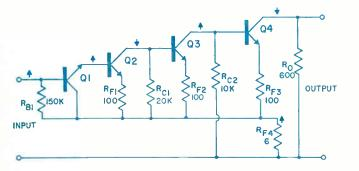
Fig. 1: Simplified circuit of the high in put impedance amplifier has common-emitter collector stage followed by 3 common-emitter stages. temperatures in excess of  $150^{\circ}$ C, but other components used in this amplifier limited the maximum safe temperature to  $125^{\circ}$ C.
