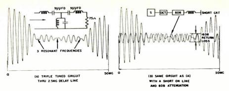
Fig 16: To determine the return loss: pattern for triple tuned bandpass filter connected to end of line (A) is superimposed on pattern of a shorted line with 8 db attenuation (B).
