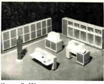
Honeywell 800 computer performs 30,000 three-address operations per second handles 8 separate programs simultaneously
