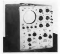
handling versatility. Risetime of the two main vertical amplifiers is 0.012 usec, and both have 0.2 usec signaldelay networks. The Type 551 sweep is common to both beams. It has 22 calibrated direct-reading sweep rates. Amplitude calibrator has 18 fixed steps. Tektronix, Inc., P. O. Box 831, Portland 7, Ore.
