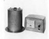
inserted in the transmission line between the receiving antenna and receiver. The frequency range is 210-250 MC. Rantec Corporation, P. O. Box 18, Calabasas, Calif.
