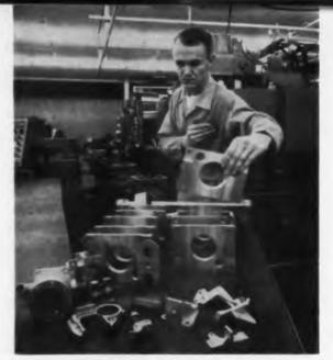
At Hughes Aircraft these precisely machined parts are turned out on a numerically controlled machine tool
