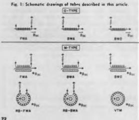
left and the output at the right, the load being indicated by the resistor with one side grounded; (2) the backward-wave amplifier, BWA, with the direction of rf power flow reversed with respect to the direction of beam travel; (3) the backward-wave oscillator, BWO, which is a BWA operated above starting current and without any rf input.
