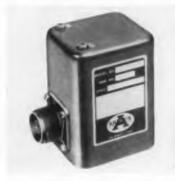
TME-2 SD are for use with fastresponse, 100-ohm-resistance temperature transducers to produce a full 5 volt output for a span of only 75 F. TME-1 SD is a single-channel unit; TME-2SD, a dual-channel unit. They meet Specification MIL-E-5272A. Arnoux Corp., 11924 W. Washington Blvd., Los Angeles 66, Calif.
