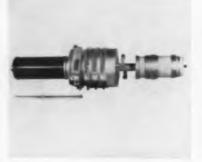
watt drive—a power gain of 10,060 times at an efficiency of 35-40%. It incorporates a modulating anode which allows simple, continuously variable control of power applied to the tube, and which permits shapedpulse and amplitude modulation as well as CW operation. Eitel-McCullough, Inc., San Bruno, Calif.
