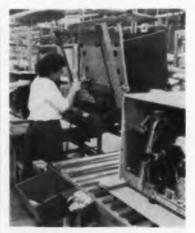
At Westinghouse's radio-TV division, Metuchen. N. J., an air operated tilt section simplifies aligning the TV chassis with the cabinet and fastening them securely together.
