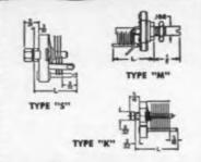
**TYPE "5" CAPACITORS** — The Type "S" Capacitor falls midway between the type "M" and "K" capacitors in physical size. Peak voltage rating 850 volts—plate spacing.013, other spacings available on special order. Square mounting studs tapped 4-40 on 17/32" centers.
