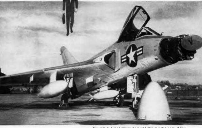
Westinghouse Aero 13 Armament Control System, mounted in nose of Navy F4D Douglas carrier-based interceptor, is typical of systems using FLEXOLON wire for faster assembly, lower production costs.
