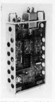
Unitized plug-in modules permit change from direct recording to frequency-modulated or PWM telemetering in seconds.
