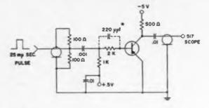
CAPACITOR ADDED FOR STORAGE AND FALL TIME MEASUREMENT Fig. 12a: Circuit for switching characteristics
