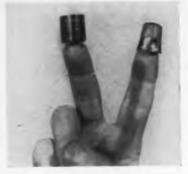
completely hermetically sealed. Stepless adjustment of inductance over a 10% range is provided and torque adjustment is such as to preclude possible strain on printed circuit mounting. Weighing approximately ½ oz. the ATE-11 and ATE-12 will find wide application in the guided missile and similar miniaturization fields. Burnell & Co., Inc., 10 Pelham Pkwy., Pelham Manor, N. Y.
