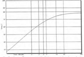
Fig. 3 (above): Temp. curve with diode mounted directly to chassis.
