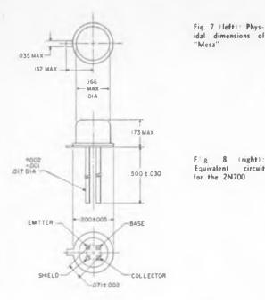
This new header configuration was necessitated in order to improve the electrical and mechanical properties.
