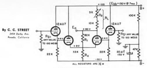
Fig. 3: Final circuit of the transformerless bridge null detector.
