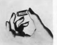
Series 341 ten-turn potentiometers are the smallest available on standard or-Only one-half der. inch in diameter by one inch in length. Double wipers are used, and backlash is eliminated. Resistance values from 1 K to 200 K are available. Daystrom Pacific, Booth 704.
