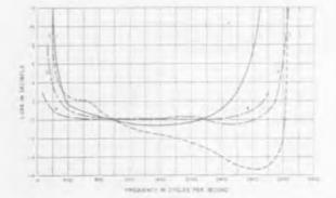
Fig. 5: Attenuation-frequency characteristics of carrier channels,
