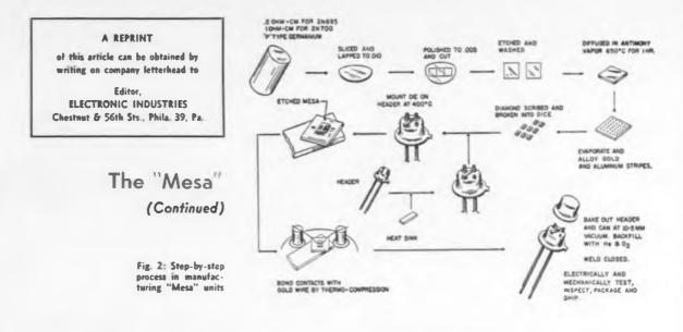
entirely germanium. That is, there are no alloys involved in the formation of the collector junction. Thus, thermal runaway in power dissipation modes of operation is far less dangerous.
