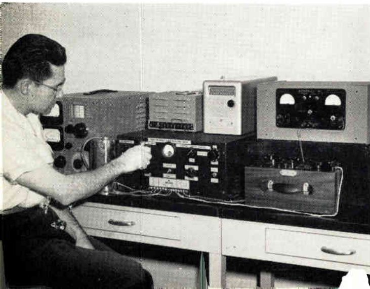
Fig. 2: The simple, reliable, single thermistor rf-power measuring bridge developed at NBS employs a constant-dc (or constant-af) current source and a shunt branch (R) to make direct measurements of the rf power equivalent.
