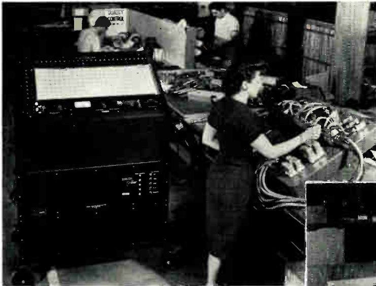
Fig. 4 (above): The automatic cable harness checker is used chiefly for circuit testing chassis and cable harness.
