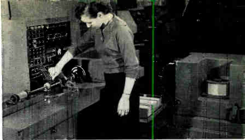
Fig. 2: Pot checker measures resistance, function, hi-pot, and noise. Accuracy: mechanical, \pm 2' of arc; electrical \pm 0.015\% of the full scale.
