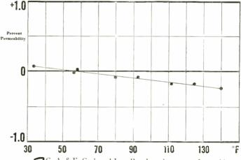
**3** G. A. & F. Carbonyl Iron Powder advantages: Low eddy current, residual, hysteresis losses (resulting in higher Q). Excellent temperature and magnetic stability. Savings (as against air-cored coils) in volume, weight, wire length. Graph above: the small permeability change due to temperature of uncompensated toroids of G. A. & F. Carbonyl Iron Powders, Grades E, TH and SF.
