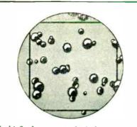
Used chiefly for cores in high frequency magnetic fields, G. A. & F. Carbonyl Iron Powders are especially high in iron content, and free from disturbing non-ferrous metals. The individual particles are spherical. Some grades contain agglomerates of several particles. Microphoto above: Grade TH at 350X. Average particles of this grade have a diameter of 5 microns.
