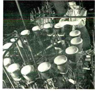
Automatic sealing machine. Tubes are preheated in circular rack at left of operator, then placed in machine; handles 7 and 10-in.
