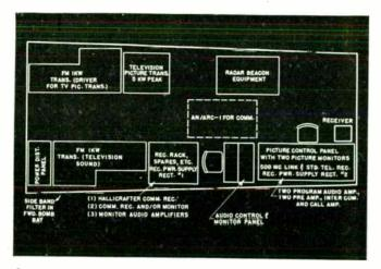
Layout of the stratovision airborne equipment in converted B-29
