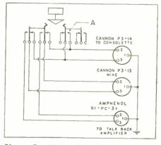
Above: Detail of talk-back switch wiring. Below: Diagram showing the connections
