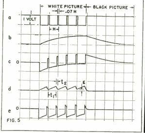
Fig. 5: Idealized representation of video signal output of second detector. A full explanation is given in the text
