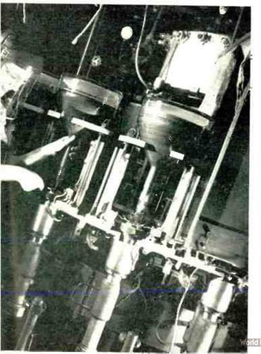
Light output is checked for brightness after electrical tests are made. Samples are operated at maximum voltage for 500 hrs.
