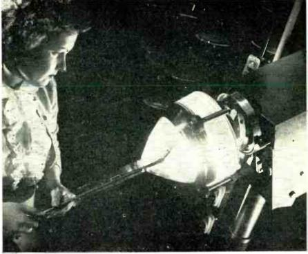
Inside walls of CR tube shown being coated with graphite which serves as part of high voltage anode and improves screen contrast. Bulb turns on a lathe
