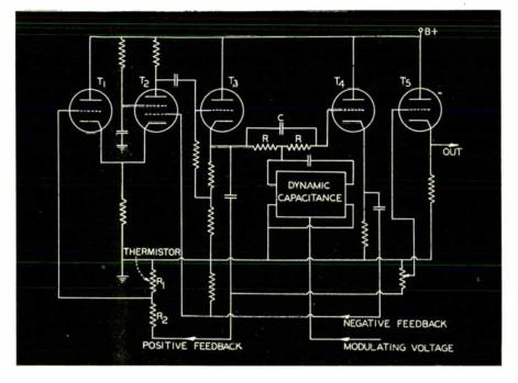
The manner in which  $Z_{in}$  varies is determined by the characteristics of the triode T<sub>v</sub>. In order to prevent the plate current of T<sub>v</sub> from distorting the output wave form, the value of resistor R should be very large compared with the output impedance of cathode follower (1).
