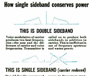
One sideband is suppressed by filters and carrier is reduced. Power thus saved is available for remaining sideband. This method of transmission conserves space in frequency spectrum, requires only a fraction of the power of double sideband, and provides an improvement of 9 db in signal-to-noise ratio.
