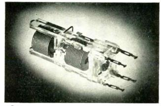
I-F and H-F applications of G. A. & F. Carbonyl Iron Powders include: I-F transformer cores, H-F adjusting cores, AM inductance tuning cores, TV wave trap cores, short-wave transmitter tank coil cores, direction finder loop antenna cores, carrier telephony cores and cups. Photo above: "K-Tran," revolutionary top quality I-F transformer, only possible with cores of G. A. & F. Carbonyl Iron Powder.
