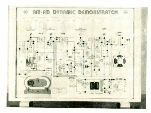
Incorporating for the first time FM as well as AM radio receiver circuits, the new RCA "Dynamic Demonstrator" is a complete six-tube receiver with circuits and components mounted on a panel 45 inches long and 33 inches high. Background of the panel is divided into six large color blocks, defining the six basic functional sections of a six-tube AM-FM radio. Jumpers to close or break the circuit are inserted at selected points
