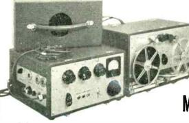
Series PT6-P, Portable Mixer-Amplifier and cover, shown with basic Recorder mounted in carrying case for portable field operations.
