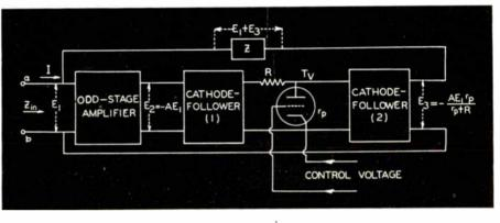
Fig. 1: Diagram of dynamic impedance circuit. Varying control voltage increases values  $1 + \bar{A}$  times
