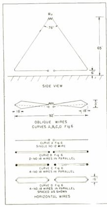
Fig. 1: Multiple-wire, delta-type antenna
