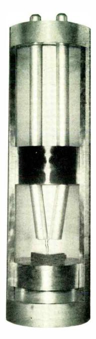
amateurs, are made to the semiconductor only two-thousandths of an inch apart. Input power delivered to one of these contacts is amplified at least 100-fold and transmitted to the other terminal where it is delivered to an output circuit. The transistor is energized by voltage supplies, such as batteries, which apply bias voltages to the two points. The power actually consumed in the transistor is less than a tenth of that used by an ordinary flashlight bulb.
