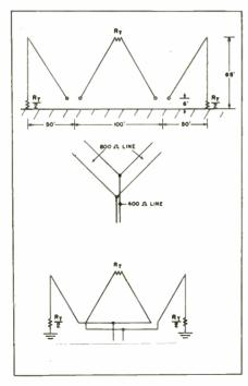
Fig. 3: Antenna and transmission line design
