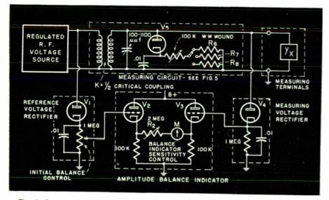
Fig. 4: Circuit includes conductance diode, differential VM, oscillator, power supply
