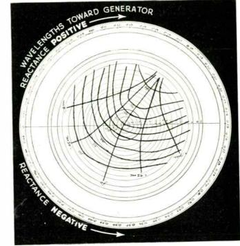
points successively by means of the double slug tuner. In this way a complete traverse of the Smith chart is made. Power and frequency readings are plotted for several standing wave ratios, different graphs representing different values of coupling of the oscillator to its load. A succession of power and frequency points of the same or approximately the same value are connected to form a system of curves, as in Figs. 2, 3, and 4.
