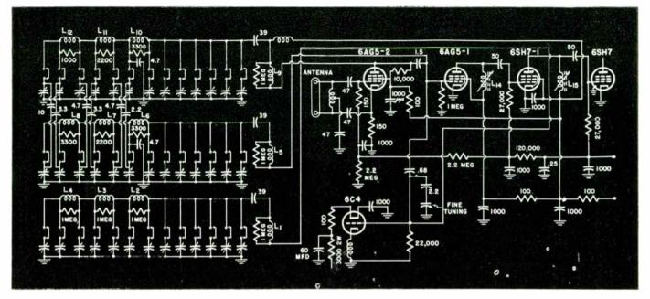
Fig. 7: Three groups of 13 trimmers mica connected to series tuned circuit of Hallicrafter's low-cost television receiver
