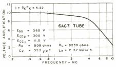
Fig. 4: Compensation curve of amplifier indicates good input and output linearity
