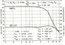
Fig. 3: Theoretical curves of compensation characteristics. See text for full details
