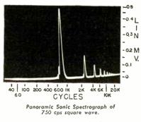
Use Model AP-1 for analyzing... • Hormonics • Intermodulotion • Vibrotion • Noise • Acoustics • Materials
