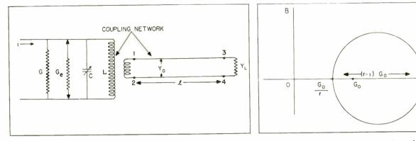
Fig. 5: In equivalent circuit of loaded oscillator,  $G_{\circ}$  is equivalent conductance coupled into oscillator circuit
