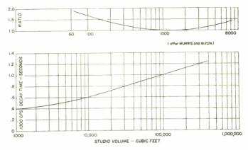
Lower curve gives decay at 1000 cps for volume in question. For decay at other frequencies, multiply by ratio value in top curve
