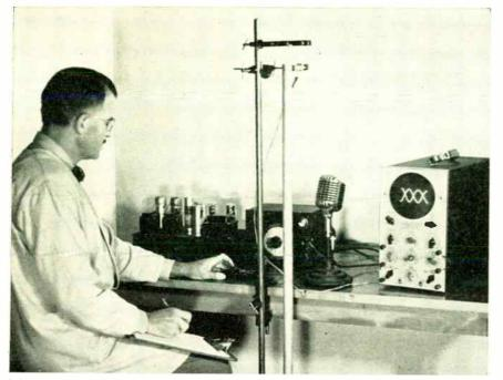
Laboratory set-up for measuring tone of chime tubes. Lissajous figure on screen of cathode ray oscilloscope is being used to determine the frequency (cycles per second) of the chime's fundamental note.
