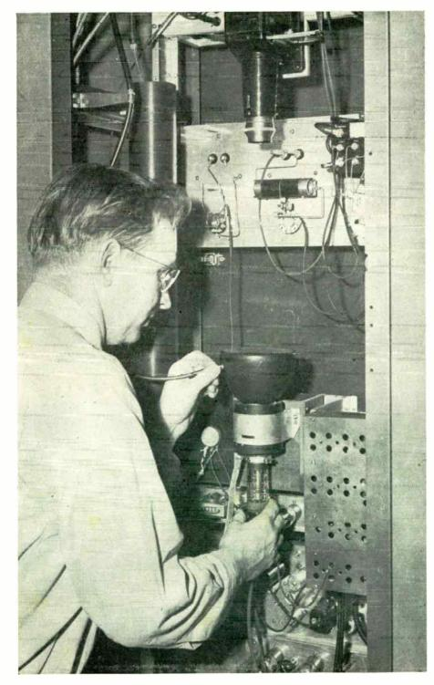
UNTIL the advent of Farnsworth's dissector tube and Zworykin's iconoscope, earlier methods of scanning live television scenes utilized the flying spot method whereby a highly intense beam of light was projected on the subject through a succession of lenses on a scanning disc.
