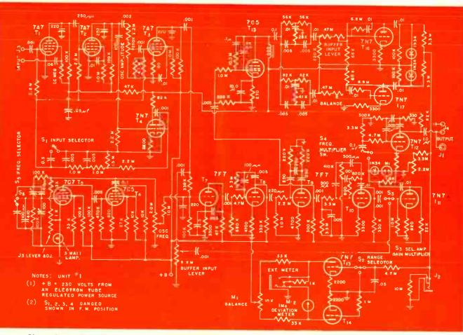
Above shows schematic of the pitch perceptor and below is the low frequency voltmeter and wave analyzer circuit
