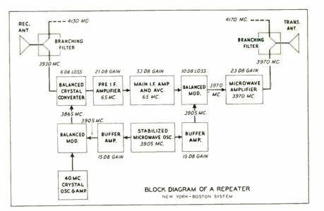
Fig. 6: Block diagram of currently used repeater station in Bell relay system
