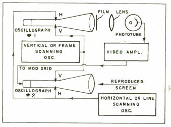
Fig. 1: Basic fixed picture television or facsimile system using the new flying spot cathode-ray tube from the oscillograph tube
