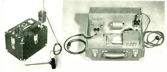
Photos below show sound testing equipment, Left: Sound level meter with vibration pickup. Right: High-speed level recorder
