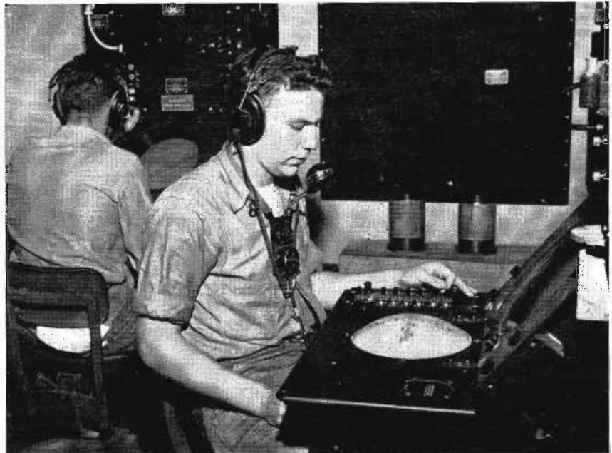
Fig. 18—The two operators sit back-to-back, operator for the Approach Indicator being in the foreground, with the Elevation operator in the background
