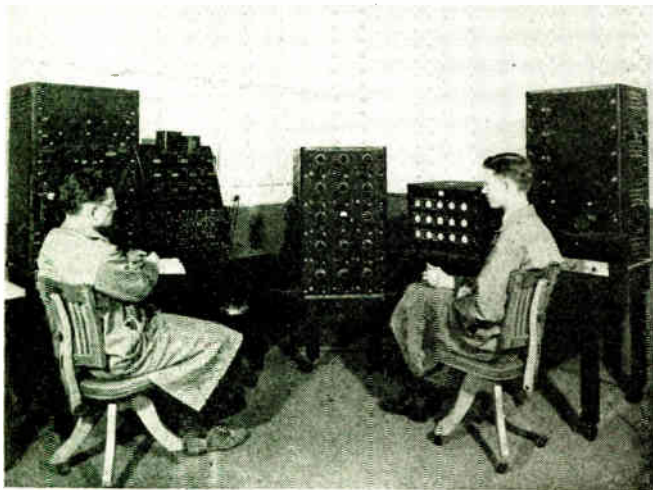
Left, the audio spectrometer, which splits sounds into 13 bands, in operation. Right, general view of the anechoic chamber showing manner in which surfaces have been treated. Equipment under test is mounted on a car and rolled in on tracks
