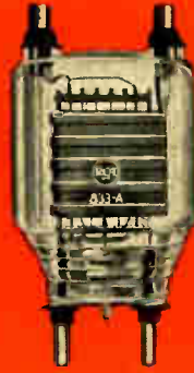
RCA-833-A Natural or forced- air cooled. 11 kw at 30 Mc. Mu=35.
