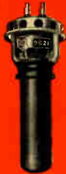
RCA-9C21 Water cooled. 100 kw at 5 Mc. Mu=38.
