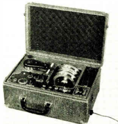
Above, new Brush magnetically coated paper tape recorder. Below, recorder using plated non-ferrous wire instead of stainless steel
