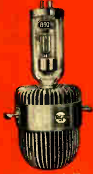
RCA-892-R Forced-air cooled. 10 kw at 1.6 Mc. Mu=50.
