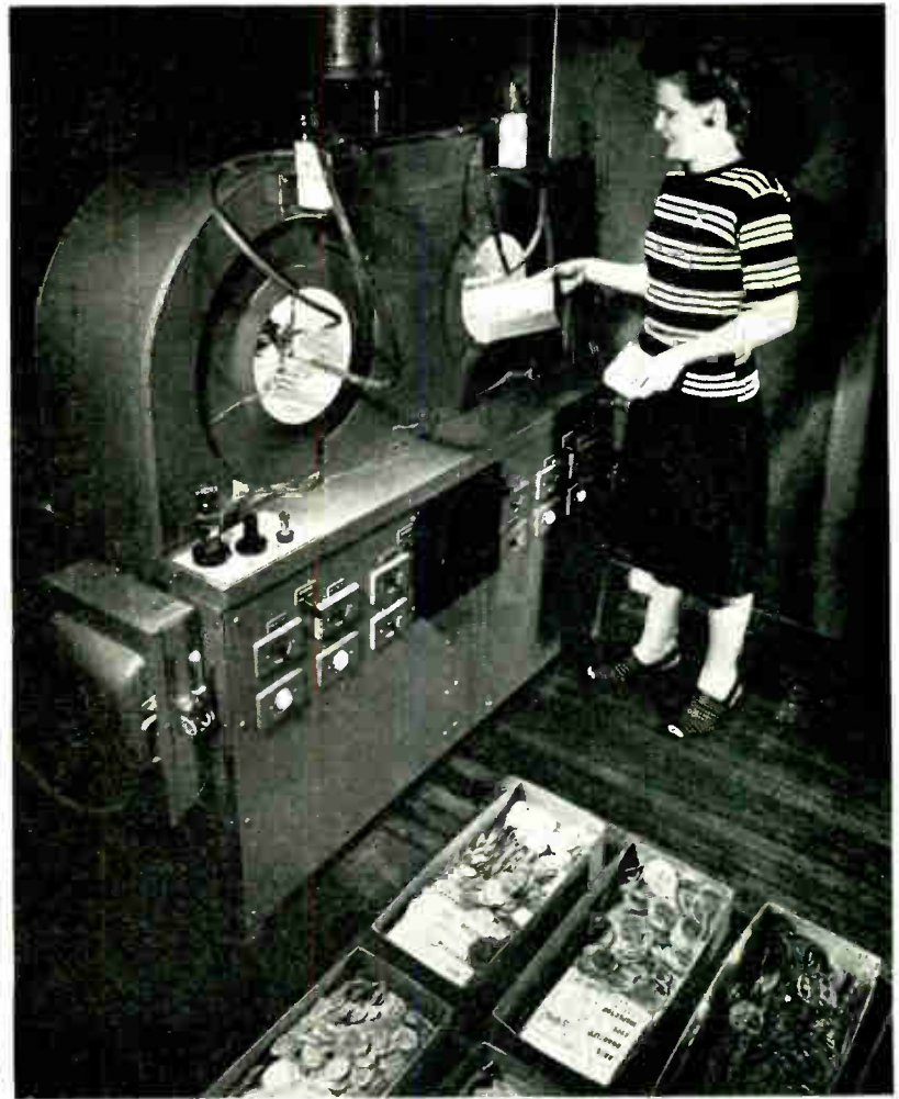
Above, a metal-tube test equipment group consists of preheaters, shorts and electrical test set, and an audio frequency noise set. Below (right), Mica insulators often are sprayed with an insulating material to decrease electrical leakage
