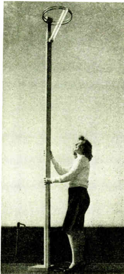
Shown upside down here, this 10-ft. shaft of aluminum will be hinged to the underside of one of the Stratovision planes from which Westinghouse will broadcast FM and television
