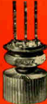
RCA-7C24 Forced-air cooled. 4 kw at 110 Mc. Mu=25.
