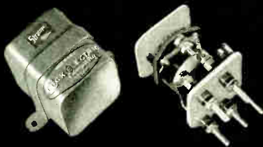
Contactors ready for Stratopaxing before covering. Wrap around mounting bracket, blister on cover for adequate terminal clearance, and binding post terminals meet specifications for unit.
