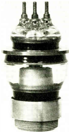
The Federal type 6C22 tube which found use in CBS transmitter the setup of which is shown in block form on opposite page
