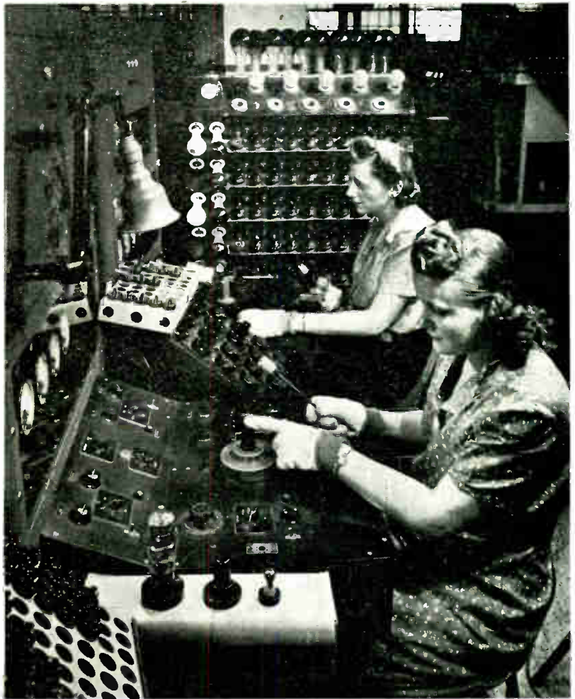
Above, a metal-tube test equipment group consists of preheaters, shorts and electrical test set, and an audio frequency noise set. Below (right), Mica insulators often are sprayed with an insulating material to decrease electrical leakage
