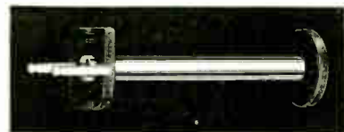
Coil core on d.c. relays is solid rod of magnetic iron, the ends machined to give an absolutely flat surface. One end is drilled and tapped for fastening to heel-piece.
