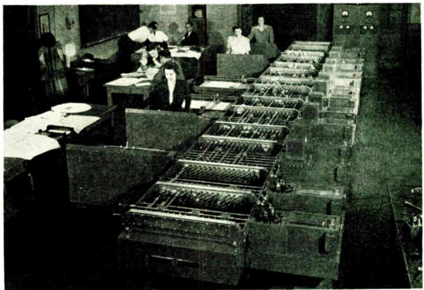
Highly sensitive polaroid photoelectric systems in this mechanical brain will permit the handling of differential equations with fourteen simultaneous integrations.
