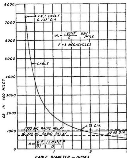
Showing reduction of repeater power needed as transmission frequency is raised
