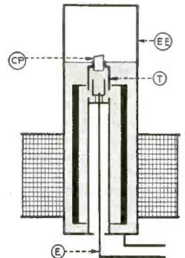
ENERGIZED—Mercury now fills thimble T, is completely leveled off and mercury-to-mercury contact established between electrodes E and EE. Degree of porosity of ceramic plug CP determines length of time delay.
