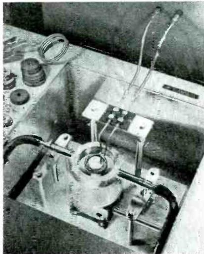
Lepel rotary induction gear heater and quenching unit automatically controls heat, improves quality
