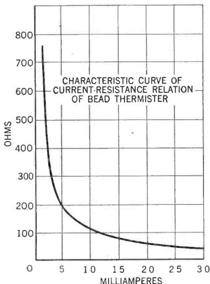
Fig. 2. Power dissipated in Thermistor heats it and unbalances bridge
