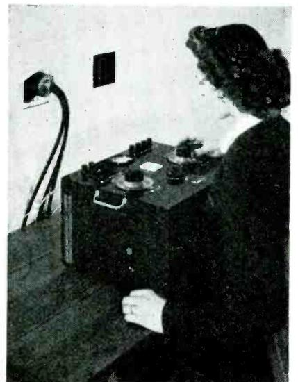
GE "reflection meter" in use by Institute of Paper Chemistry, Appleton, Wisc., for determining the whiteness of paper pulp
