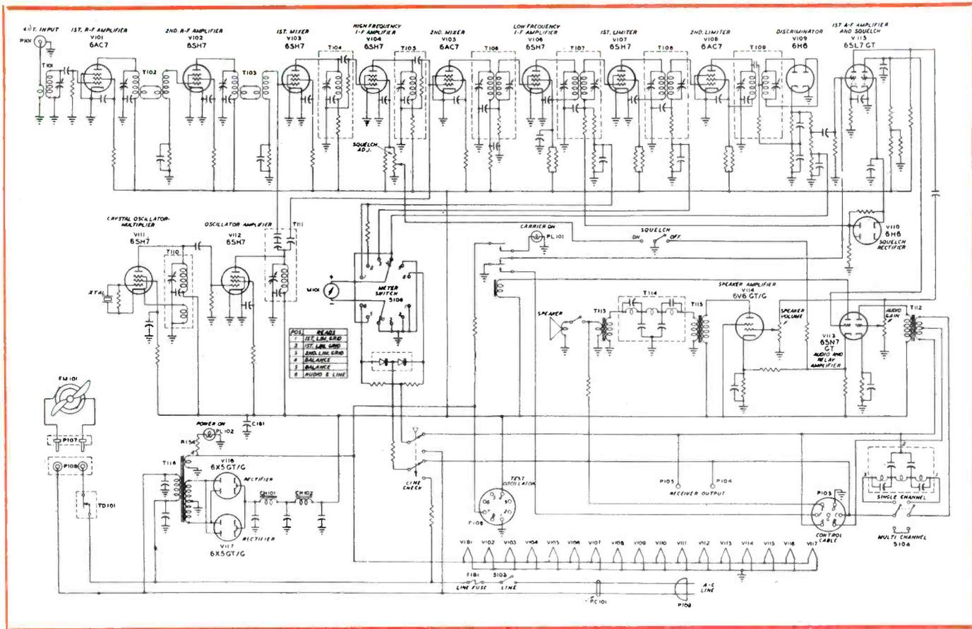
Complete circuit diagram of receiving set. Low pass filters, center (T114) and lower right, permit the use of channel 1, audio frequencies below 3,000 cycles, for monitoring and break-in service when set is used at relay point
