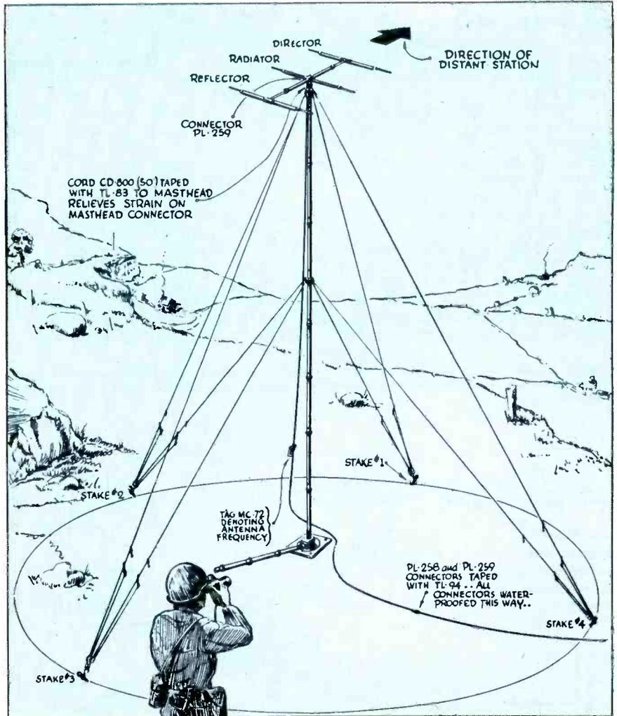
Antenna system completely installed in the field. The radiator, director and reflector element lengths and spacings must be adjusted for the operating frequency. Direction of transmission must be established by exact sighting
