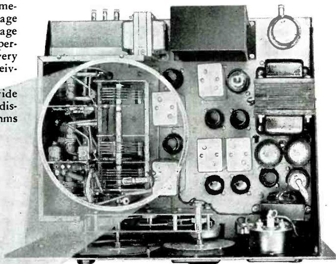
The RF section is built as a unit on a separate chassis which may easily be removed for servicing and incorporates a three position ceramic band switch. The positive action mechanical bandspread dial turns through more than 2200 divisions for each of the three ranges, 27.8 to 47, 46 to 82, and 82 to 143 megacycles.
