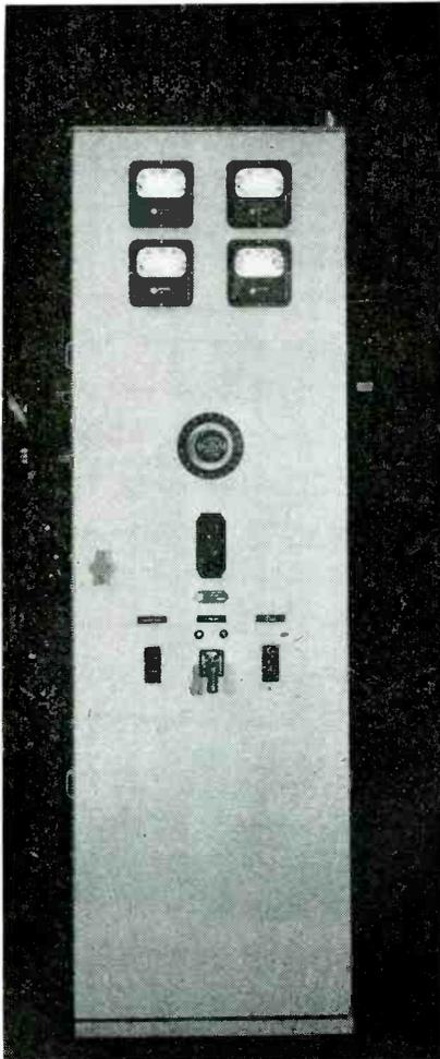
Fig. 5. Control cubicle necessary for operation of unit shown in Fig. 4 contains grid control, arc excitation, and vacuum measuring apparatus
