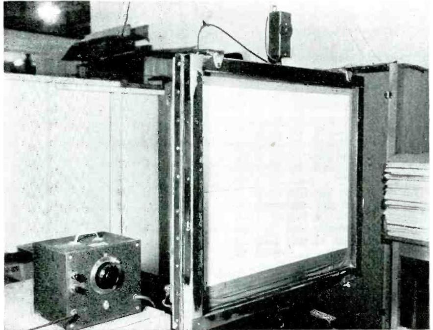
General Electric Totalux equipment in lithoprint plant of Edwards Bros., Ann Arbor, Mich., accurately determines photographic exposure time and compensates for fluctuations in light intensity
