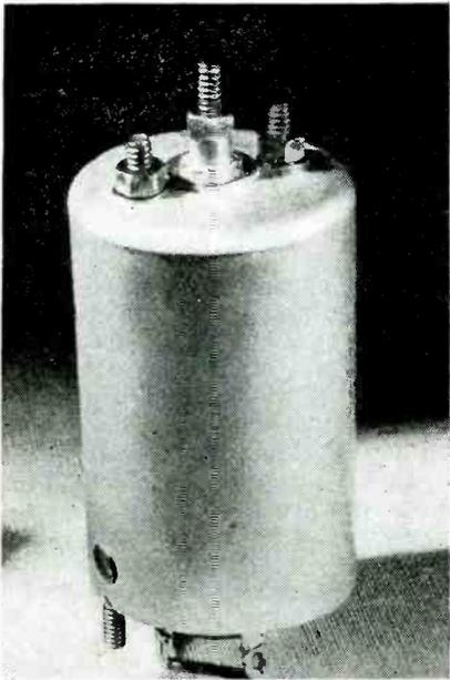
Efficient iron cored rf transformer in aluminum shield can with permeability adjustment of inductance
