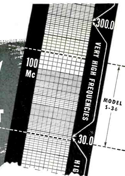
**T**HE Model S-36 is probably the most versatile VHF receiver ever designed. Covering a frequency range of 27.8 to 143 megacycles it performs equally well on AM, FM, or as a communications receiver for CW telegraphy. Equipment of this type was introduced by Hallicrafters more than five years ago and clearly anticipated the present trend toward improved service on the higher frequencies.
