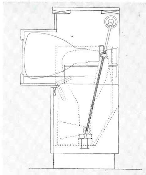
Fig. 3. At right is home cabinet design with tube in viewing position. Push-button operated motor moves tube when set is to be used
