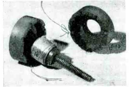
Small pot type assembly consisting of two cup cores and a center slug surrounding the compact coil. The center slug can be adjusted to vary the inductance
