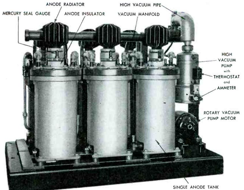
Fig. 4. Arrangement of six tanks and vacuum system. Note heat radiator fins on anodes
