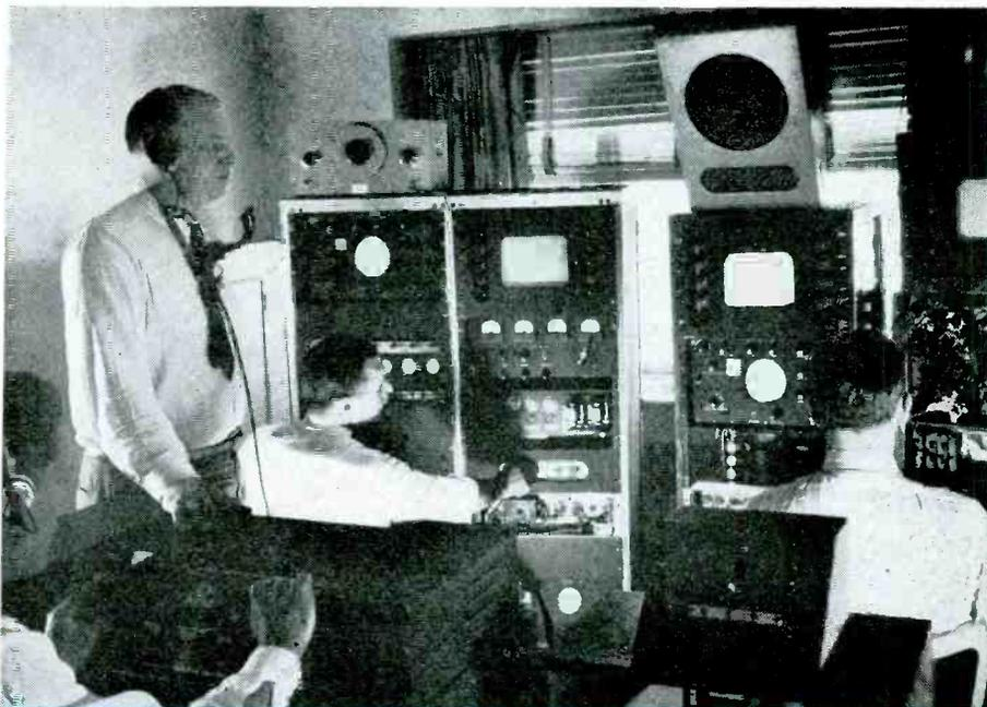
Fig. 3. Video monitoring equipment at Statler Hotel in Washington, reference marks are placed on the various monitor CR tubes for establishing synchronizing levels, etc.
