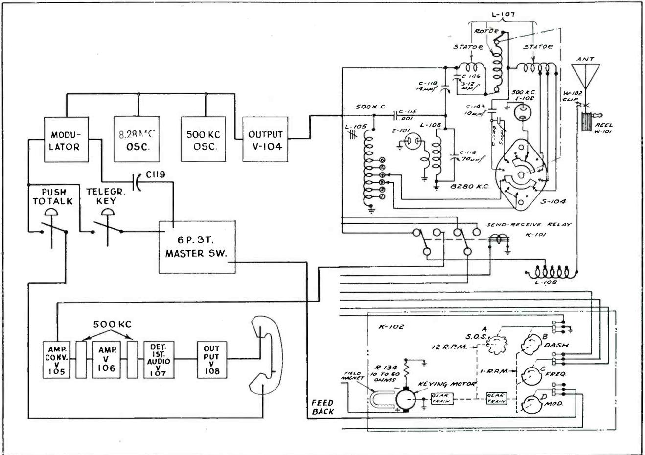
Fig. 3. Combination block and circuit diagram showing layout and noteworthy features of automatic keying mechanism and double output tanks. Rotation of L-107 for 500 kc tuning automatically changes taps on L-105 and L-107. A high impedance loop with C-145 blocks grounding of 8.28 mc output
