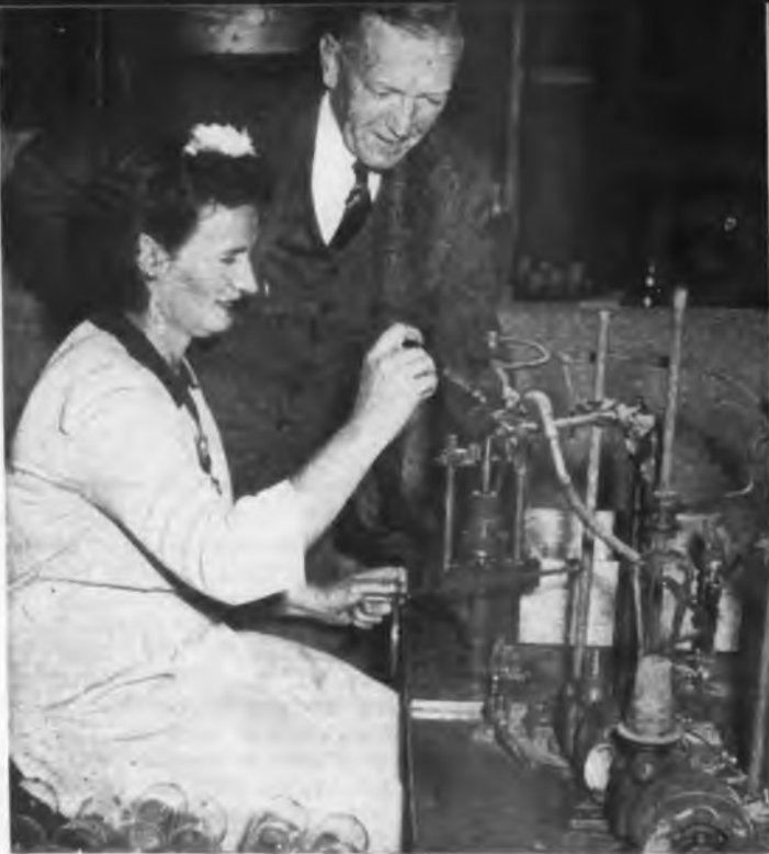
1 —Mass production isn't always best way. Top seal operator at United Electronics Co., Newark, N. J., upped production six times on 967 rectifier with jig to handle them individually, reducing breaking off of anodes, cracked seals, and other shrinkage
