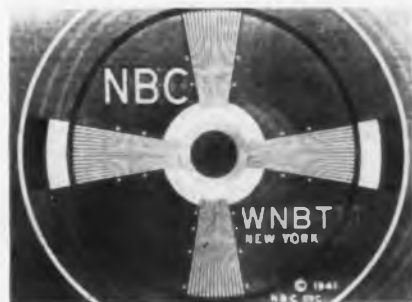
Multipath No. 1, 2480 feet and 7 per cent amplitude and No. 2, 4500 feet and 7 per cent
