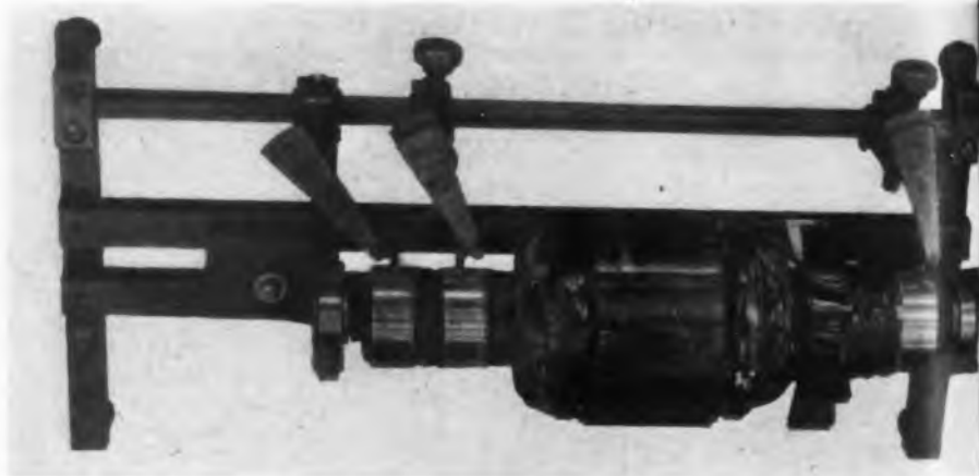
3 —Ingenious fixture devised by engineering staff of Carter Motor Co., Chicago, does three truing up jobs at once, which formerly involved separate operations. Bearings, shafts, and commutators of rotating power units must be concentric within close tolerances for proper operation. This new type gage gives a check accurate to .0001-in. within a few moments. Armature is simply set into jig in its own bearings and rotated. Indicating gages measure eccentricities for easy truing up
