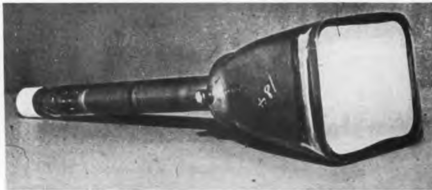
A cathode ray tube developed for CBS color television has flat viewing surface and screen same shape as image. Image is same size as conventional 7-in. round tube—5½ x 4¼ in. Magnifying lens is used.
