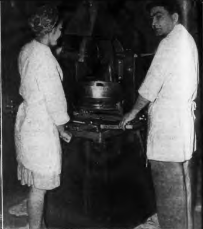
2 —Catch pan proved to be a war bond oil well to North American Phillips Co. worker, if you don't mind mixing metaphors. Oil is ammunition and many other things to this quartz wafer saw worker, who devised simple catch pan, to save and re-use the vital coolant
