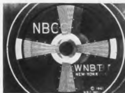
Multipath No. 1, 3940 feet, 30 per cent and No. 2, 11,100 feet at 2 per cent amplitude
