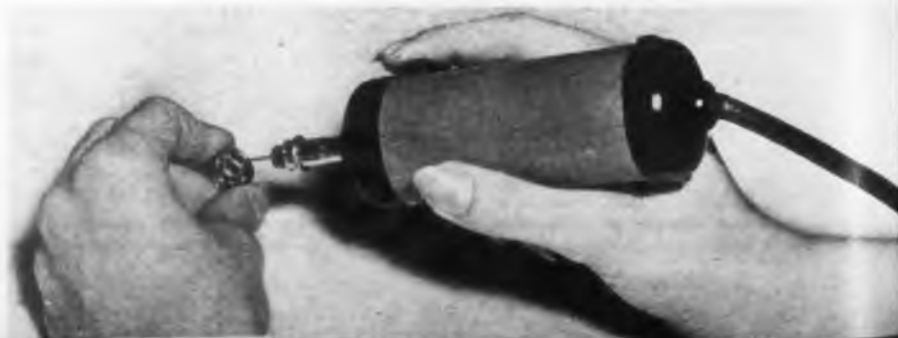
4 —Motor driven eraser drafted from the drafting room solved a tough problem by salvaging four thousand dollars worth of rusty miniature ball bearings at the plant of International Business Machines Corp., Endicott, N. Y. Used in delicate assemblies, the bearings can not be oiled because of the burden of the oil's viscosity. Only satisfactory way to remove rust before installation proved to be by "burnishing" the balls and races with rapidly vibrating soft steel wire held in chuck. Best "tool" for the purpose was paper-clip wire!
