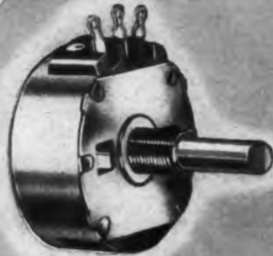
This is the new 1 1/2" diameter, wire wound variable resistor, 352 Series, with resistance value up to 20,000 ohms linear and with the same bakelite housing and grounded metal construction as the popular 1 1/4" 252 Series. (This resistor only, shown at actual size.)
