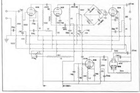
Fig. 5-Sonic flocculating unit capable of developing 2500 watts. Amplifiers at left
