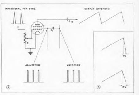
Fig. 2—Waveforms generated at screen and suppressor grids, and at output of circuit in Fig. 1. Synchronizing signal should be short duration pulse as shown. In B, the return trace time is 9 per cent up to approximately 180 kc and 15 per cent at 1 mc
