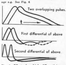
Fig. 8—Effect of multiple differentiator on overlapping pulses. Permits separation for control purposes
