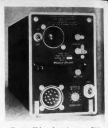
Fig. 10-Glide path receiver, type RUJ
