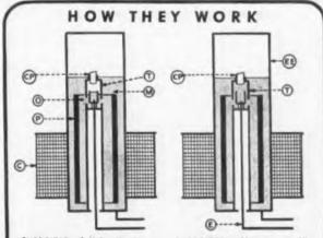
ENERGIZED-Coil C pulls plunger P down into mercury. Mercury thus displaced enters thimble T through orifice O. Inert ges in thimble gradually escapes through ceramic plug CP-thus producing time delay. ENERGIZED — Mercury now fills thimble T, is completely leveled off and mercury-to-mercury contact established between electrodes E and EE. Degree of porosity of ceramic plug CP determines length of time delay.
