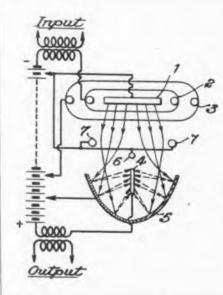
part of the anode 4, so that the secondary electrons go directly to the flat sides of the anode. The electron beams impinge on the inner surfaces of the secondary emission electrode 5 in such a way that substantially all secondary electrons pass directly to the anode without oscillating around or near it, and practically none of them return to the vicinity of the control grid 2. A. J. W. M. van Overbeek, Allen Property Custodian, (F) June 6, 1941, (I) Feb. 1, 1944, No. 2,340,631.
