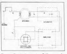
Fig. 6—Circuit for tracing B-H curves for magnetic samples using cathode ray oscillograph. Low frequency ac is used
