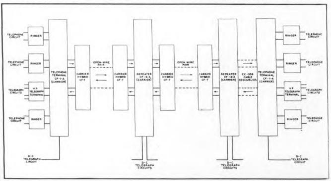
Block diagram of complete spiral-four carrier telephone and telegraph system showing equipment used to provide three telephone, four duplex telegraph, one alarm and one dc telegraph circuits on new four wire cable. Terminal repeater equipment housed in portable cases
