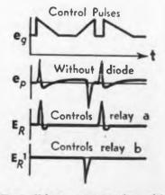
Fig. 6-Voltage waves at various points in circuit of Fig. 7
