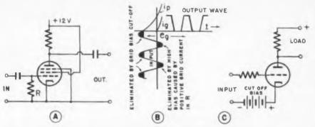
Fig. 3. Pentode limiter circuit at (A) uses low voltages and grid leak bias to limit response on positive and negative cycles as in (B). At (C) is clipper circuit to pass only part of positive half cycle of input voltage. Bias battery adjusts clipping level
