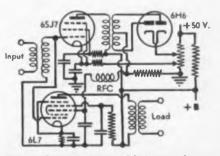
Fig. 4. Limiter circuit with increased control range uses separate amplifier tube (6SJ7) and rectifier (6H6) to control 6L7 arate the synchronizing signals from the video in television.
