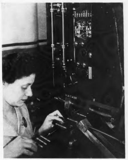
Close-up of delivery end of Matam Corporation's shell inspection machine. Note final measuring and ejecting positions
