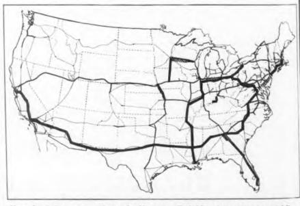
Heavy line indicates proposed coaxial cable routes. Shaded line shows existent coaxial lines ELECTRONIC INDUSTRIES • May, 1944
