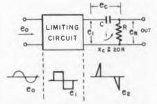
Fig. 5. Typical circuit for producing sharp pulses of short time duration. Sine wave input converted to square wave by limiter and differentiated by R-C to give pulse
