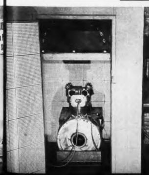
Constitution detector equipment on engine in soundproof chamber. Photo shows tests in progress on improved detonation detector equipment being developed by the research laboratories at Sperry Corp. Tests involved are similar to the actual operation of the equipment as used in work on aircraft engines
