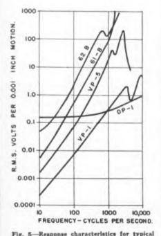
Fig. 5—Response characteristics for typical inertia type piezo pickup Shure and Brush (with rising characteristics) and stylus driven displacement unit, Brush DP-1
