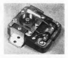
Fig. 6—Western Electric RA-355 vibration pickup with cover removed (above). Combines high-directional sensitivity and wide frequency range
