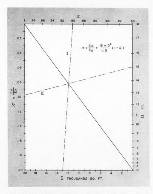
A formula for the ratio (r) of the energy density  $E_{\rm H}$  of reflected sound to  $E_{D*}$  that of the direct sound appears on the nomogram above.
