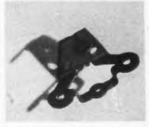
Instrument frame of beryllium-copper outperforms a die casting, costs less and requires no finish machining. Formed while soft and hardened in fixture to hold important dimensions
