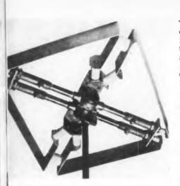
Fig. 3--One of localizer beam radiators for producing pattern shown in Figs. 2 and 4
