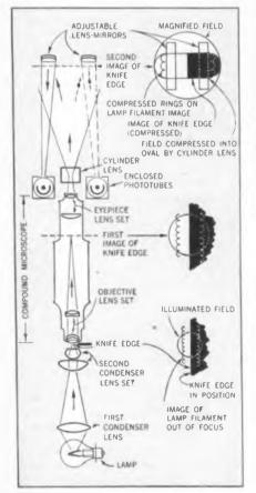
Fig. 1—Diagram of one of the 8 optical and photoelectric units. Knife edge takes a position determined by actual dimension being measured
