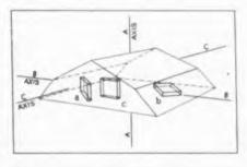
Fig. 2-Rochelle salt crystal exhibits greatest piezo-electric effect along axis 45 deg. from B and C perpendicular to A
