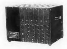
tubes are used for counting and indicating a scale of ten. The answers are indicated for each decade on four neon lamps desinated 1-2-4-8. Combinations of these lamp indicate 0 to 9. The instrument operate from a line voltage of  $100-125 \times 60$  cycle ac. The tube complement is 27 tubes. Plugin construction of the units is used throughout. The counter chronograph interval timer's dimensions are 15 in. x 10 in. x 10 in., and the weight is approximately 39 nounds.
