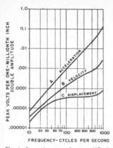
Fig. 4—Conversion curve for type 61B vibration unit (Shure). Curve A with 3 megohm load, B with a 3 megohm—.003 mf integrating stage, and C with two of these integrating stages in cascade
