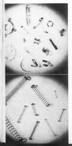
ty is twice that of bronze, and it will maintain spring properties under temperatures 100 deg. F. higher than bronze. In addition, it has less tendency to drift or take a set than any other spring material, an important property in many electronic applications.
