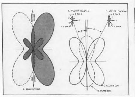
Fig. 2—Radiation pattern for localizer bean at left is composite of two patterns at right (Fig. 4). Course sharpness is 1.2 db per 1.5 deg. off-course. On-course signal approximately 2.75 db below maximum at 25 deg. off-course
