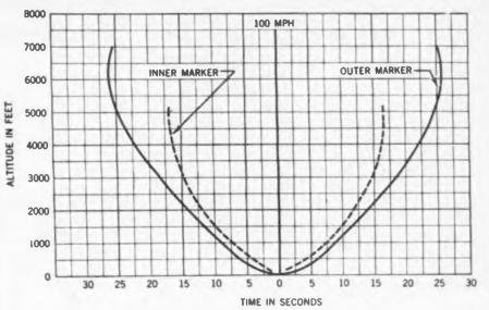
Fig. 9-Vertical pattern of outer and inner marker beams showing duration of indicator lamp glow at various elevations in feet for plane speed of 100 mph
