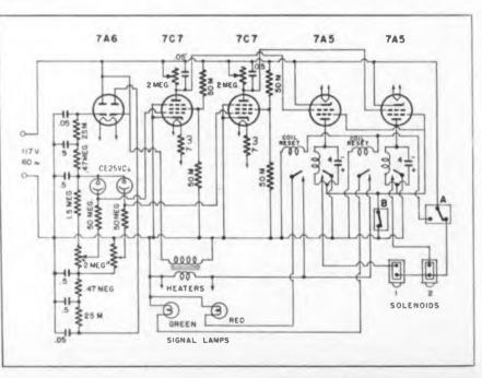
Circuit diagram of photoelectric dimension gager unit. Microswitches A and B operated by cam on conveyor mechanism. Phototube signals operate solenoids 1 and 2 to reject off-size shells operated at 4.5 volts instead of at 6.3 volts. This has been found to be helpful when phototubes deliver very little current, as in the present case.
