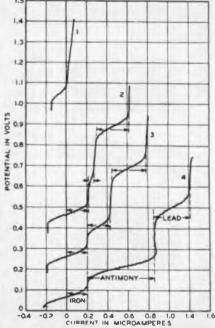
Fig. 3—Changes in current, as the potential applied to the electrodes increases, are recorded. To avoid superimposition of curves the vertical scale indicates voltage differences so that curves start at different points
