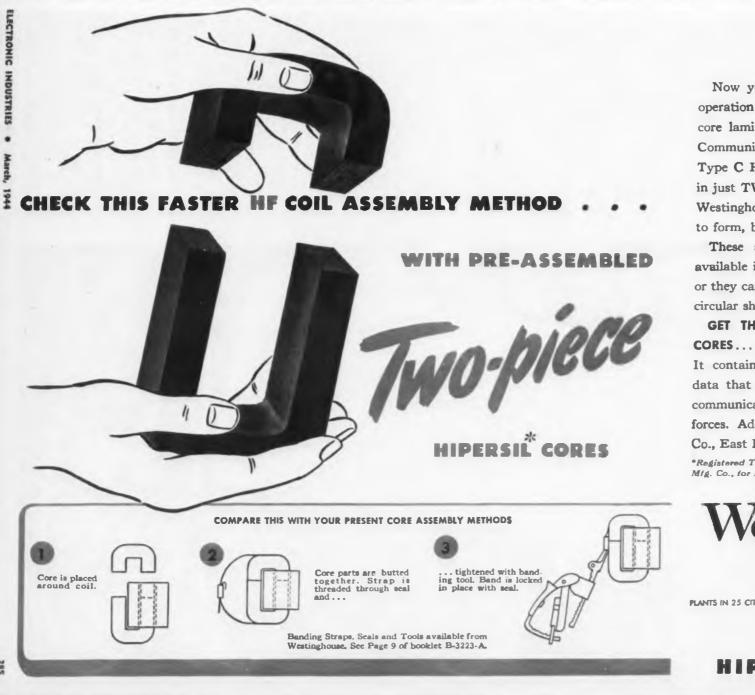
Now you can eliminate the time-consuming operation of stacking hundreds of tissue-thin core laminations by hand for High-Frequency Communications Equipment. Pre-assembled Type C HIPERSIL cores are delivered to you in just TWO ready-to-assemble pieces per loop. Westinghouse winds a thin strip of HIPERSIL to form, bonds it, then cuts it in two.
