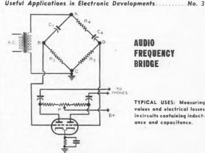
TYPICAL USES: Measuring values and electrical losses incircuits containing inductance and capacitance.
