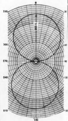
Fig. 4---Secondary voltage pattern of a Circutrol (782-02) for various powitions of the shaft
