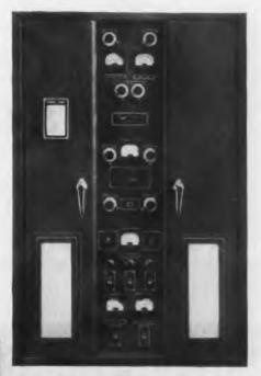
**Transmitter** for Airport Traffic Control. Output rating 50 watts, Frequency range 116 to 126.25 megacycles.
