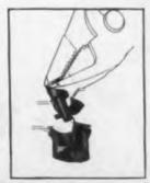
Stud Assembly is easily inserted or removed as a unit. Selection of correct size at final assembly allows for cumulated tolerances. Cross pin is permanent.
