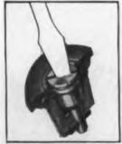
Camloc high speed fasteners operate with a quarter turn of the screwdriver. They secure doors and access panels in metal, plastic or plywood.
