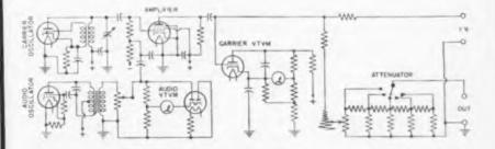
TYPICAL USES: Analyzing circuit performance of radio, sound, and other amplifiers at selected excitation frequencies.
