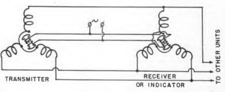
Fig. 1—In their commoner uses, rotors of all units in a group are excited from the same single phase source of ac
