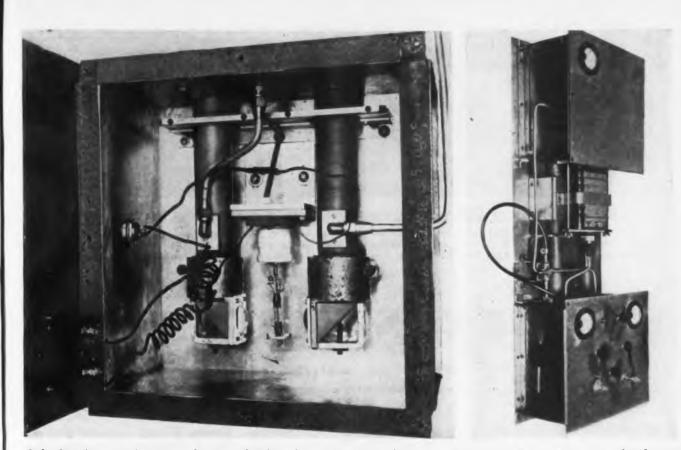
Left: Interior of light-source chamber, showing ultra-violet lamp with outer glass envelope removed; condensing lenses, and prisms. Right: Close-up of the analyzer. Chamber at top holds ultra-violet generator and quarts condensing lenses and prisms. Two large gas tubes connect to analyzing chamber, at bottom containing balanced phototubes and amplifier
