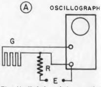
Fig. 11-Method used to connect strain gage to an oscillograph
