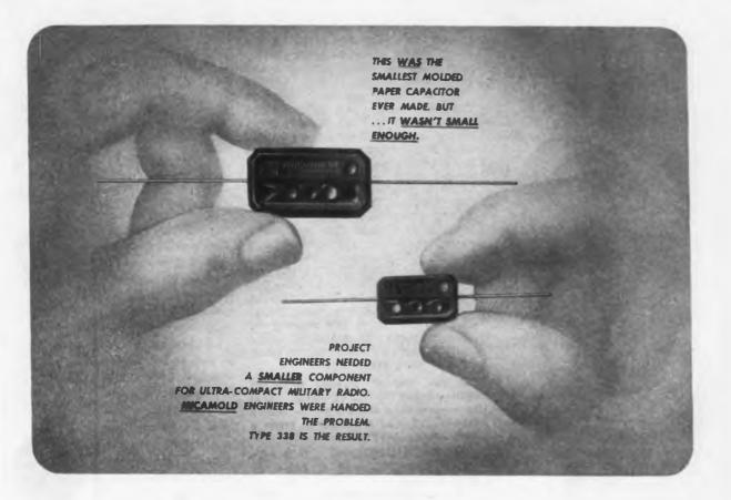
The Type 338 is a paper by-pass capacitor molded in bakelite. Specially designed manufacturing equipment was built to produce it. The Type 338 is very small, measuring only  $\frac{3}{4}$ " x  $\frac{7}{16}$ " x  $\frac{7}{32}$ ". And it weighs but 2.5 grams. These units are used in large quantities in their special application.
