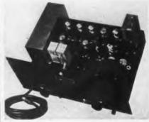
ordinary indoor temperatures. Output voltage available is at least 30 volts for any frequency. Output impedance is 500,000 ohms maximum. The wave shape at all frequencies is sinusoidal and symmetrical within approximately 10 per cent. The unit is manufactured by American Time Products, Inc., 580 Fifth Ave., N.Y.C.
