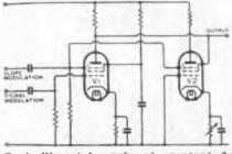
Controlling tube gain at constant de current
