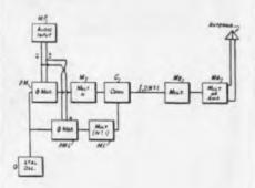
by the integer 1. The output of mixing tube C then contains the original carrier, i.e., the difference frequency of its inputs, having a phase deviation equal to the combined retarded and advanced phase deviations of modulators PM and PM1, i.e., equal to  $2N \pm 1$  times the original phase deviations. This output component is multiplied, amplified and transmitted by the antenna. H. E. Goldstine, RCA, (F) June 10, 1942, (I) Dec. 7, 1943, No. 2,-335,934.
