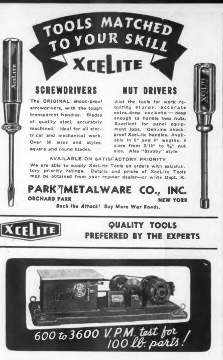
**E**LECTRONIC, aircraft and electrical parts and assemblies up to 100 lbs. in weight can be readily subjected to continuous or intermittent vibration fatigue test—the test that answers many questions about engineering, design and construction materials—on the **Model 100A All American Vibration Fatigue Testing Machine.**
