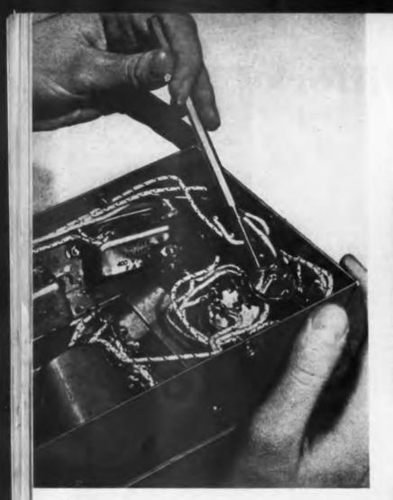
2 A DENTAL MIRROR enables solder-girls and inspectors to see both sides of every connection at Electronic Labs., speeding wiring and eliminating rejects.
