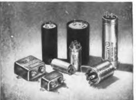
TYPICAL example of Mallory progress in building components is this BS 81 "Bathtub" Capacitor. Rated at 8 mfd. 500 volts, with a 700 volt surge, it is hermetically sealed in a steel case measuring only 2"x1¾"x1". Its -40° C impedance at 120 cycles runs as low as 220 ohms. The Capacitor itself has been thoroughly tested in war service from the arctic to the tropics.
