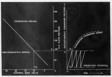
Fig. 2a (Left). How control characteristics of an SS4 affect oscillation voltage and frequency, Fig. 2b. How a thyratron generates oscillation
