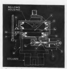
Cross section of double pressure bellows system with the hend in the up position of operating stroke
