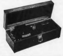
It operates with a barrier-lever photocell which is connected to a taut-wire suspension galvanometer. The instrument is built into a portable wooden case  $5 \ge 6 \ge 15$  in. and does not require any external power connection.
