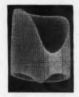
Another DuMont cyclogram, this time indicating high internal streams. The Cyclograph may be used to distinguish between two pieces of steel having the same hardness, one of which has low internal stresses and the other higher internal stresses and therefore more brittle.
