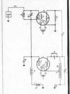
pedance to the harmonic frequency, but a high impedance to the fundamental frequency. It is stated that large amount of harmonic energy can be secured with relatively good plate efficiency and with out the use of extra filters or wavetram circuits. J. Markowitz, (F) March 31, 1942 (1) Sept. 7, 1943, No. 2.329,069.
