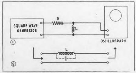
Test circuit for measuring inductance and stray capacity with square wave generator and oscillograph. Circuit 1 will measure capacity if R is replaced with C and L by R
