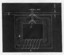
Sectional view of recording and reproducing head showing flux path
