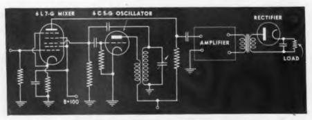
Fig. 1. General circuit for amplifying a steady potential by letting it modulate a fixed carrier
