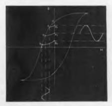
Relationship between Br and Hr when using h-f recording system
