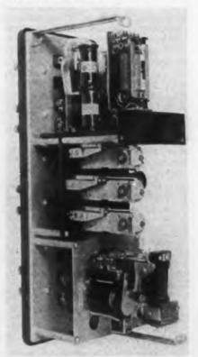
Fig. 12—Automatic synchroniser uses two low-power vacuum tubes
