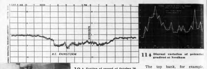
10 A Portion of record of October 28, 1943, showing point discharge between earth and sky during a rainstorm
