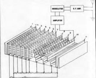
Fig. 1, Right—Basic elements in the Craig pickup tube for deriving a television signal without scanning Fig. 2—Closeup of a few of the holes of the signal generating electrodes of Fig. 1. Method of applying winding to an element shown in inset
