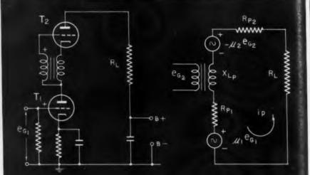
Fig. 5-Actual and equivalent circuit for transformer coupled series tubes. Equivalent circuit voltages 90° out of phase approximately b
