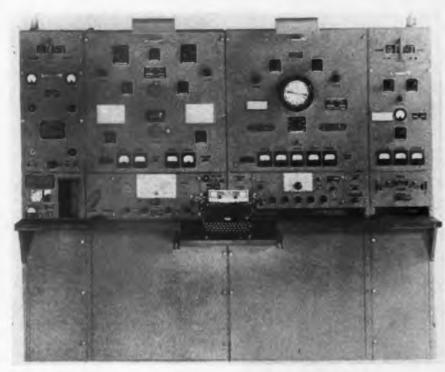
Left to right, panels in the unit hold the auto alarm, high frequency unit, low and intermediate frequency unit and the emergency equipment
