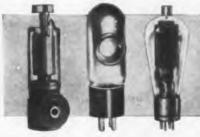
A G-E X-ray tube (1), a G-E stratetube (2), a G-E thyratron tube (3), and several G-E amplifier tubes are the "oyes and brains" of this increasing machine.
