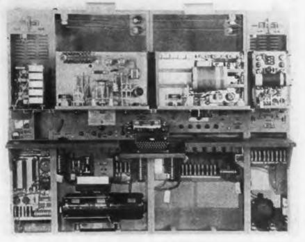
Front view of the console unit with all panels open showing arrangement of the various transmitters and receivers and their accessibility
