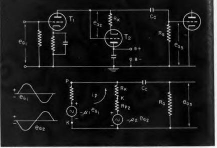
Fig. 1—Typical circuit with tube  $T_p$  acting as load impedance for input tube  $T_p$ . Voltage  $E_{gp}$  is developed across  $R_p$ . Equivalent circuit below shows relative polarity of equivalent generators
