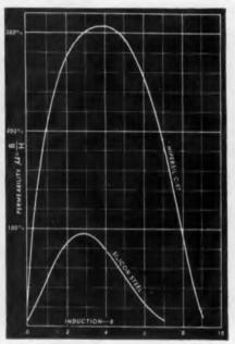
Fig. 2 — Permeability of Hipersil and ailicon steel
