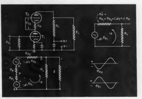
Fig. 3-Actual and equivalent circuits for series tubes working into resistance load. Voltage Egt is developed across resistor R, 180° out of phase with Egt
