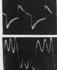
Upper pattern is voltage across inductance for circuit I at right. End point of decay is 4 per cent of initial voltage. Lower pattern is 2.5 cycles of damped oscillation for circuit 2
