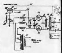
amplifier tubes 32 or 33 predominates, in case of class A operation, or which of them conducts, in case of class B operation. E. S. Winlund, RCA, (F) Oct. 31, 1941, (I) Oct. 12, 1943, No. 2,331,821.
