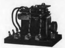
amps. Contacts are rated 5 amps. at 115 volts, 60-cycles and may be had up to 3-pole double-throw. The coil may be wound to operate on any wattage between 32 and 4.5; resistance is 8 ohms. Vibration resistance, energized or de-energized, is eight times gravity. Insu ground, tested at 900 volts ac. Insulation to
