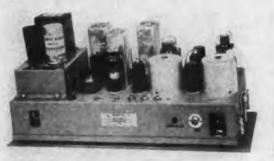
Type PRS-9X, 30-40 MC Mobile Receiver with Dust Cover Removed.
