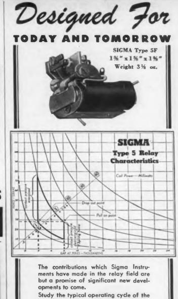
Study the typical operating cycle of the new Sigma Series 5 Relay shown above —notice that it is operating at 5 Milliwatts with 4 mil air gap between contacts, and 4 mil air gap at poles. Notice further, that contact pressure of over 40 grams is provided in the energized state and 28 in the deënergized state.
