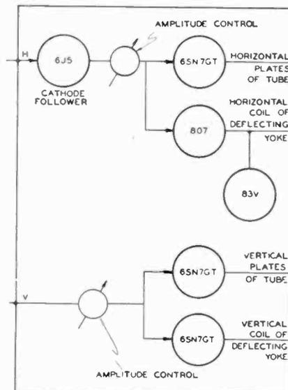
Fig. 10—Deflection amplifier and control diagram, 24-position rack
