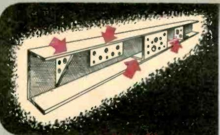
SWITCHBOARD CHANNEL FRAMES HAVE BRACKETS ATTACHED BY WELDING.
