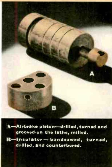
**A**—Airbrake piston—drilled, turned and grooved on the lathe, milled.
