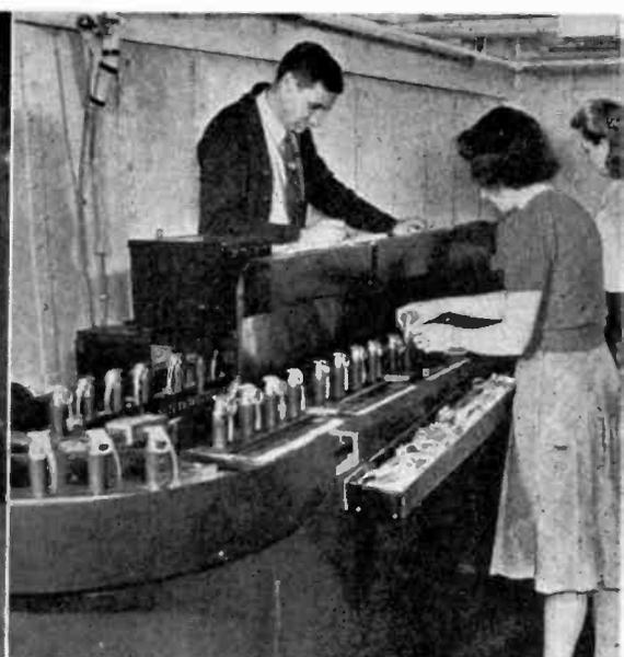
Automatic check on grenade fuses. Phototube behind fluoroscope screen sounds alarm if powder charge is incorrect, in this G-E set-up
