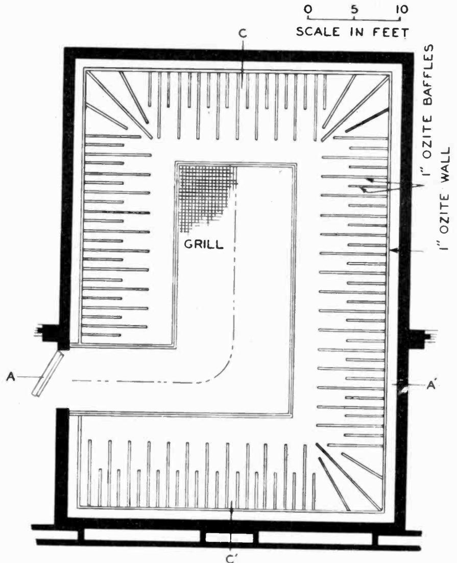
Plan of the free field sound room laboratory showing method of applying sound absorption material and location of platform grill
