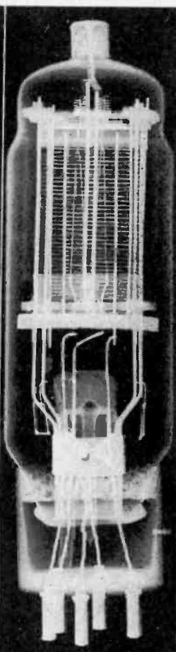
Tubes are X-rayed on film or paper to check elements
