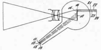
and the mica plate. The lines of four-line plate 18 are correlated with the lines of the mosaic color line screen and are fed to separate amplifiers through leads 21, 22, 23, 24. A similar arrangement is used for the receiver. B. T. Hewson, (F) Aug. 20, 1941, (I) Aug. 31, 1943, No. 2,328,145.
