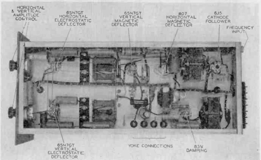
Fig. 4—Deflector chassis of sixteen-position rack
