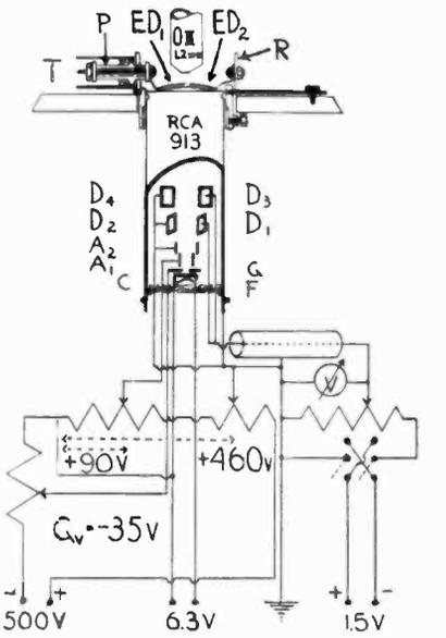
Cathode ray tube voltmeter
