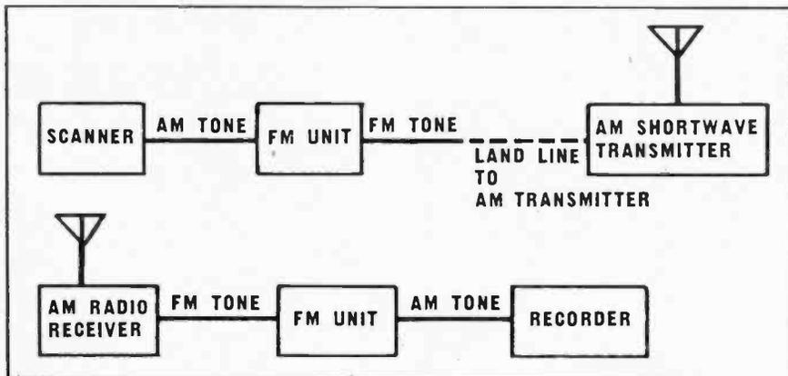
Although the principle of sub-carrier frequency modulation is neither brand new nor novel, having been introduced to commercial use by RCA in 1939 with the opening of a circuit between London and New York, there is considerable element of newness in the light-weight compact equipment developed by OWI engineers and in the method of using it.
