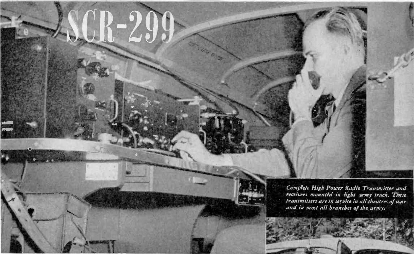
Complete High Power Radio Transmitter and receivers mounted in light army truck. These transmitters are in service in all theatres of war and in most all branches of the army.
