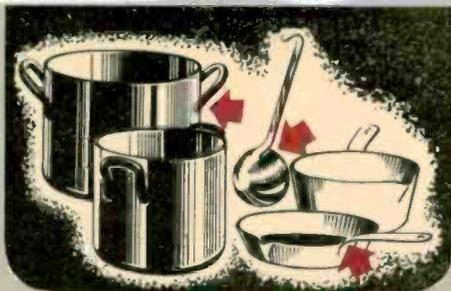
STAINLESS STEEL, ALUMINUM OR STEEL KITCHEN UTENSILS HANDLES PROJECTION WELDED.
