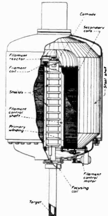
Tube in "Million Volt" unit is mounted inside high-voltage transformer
