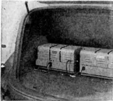
Complete 22 Watt High Frequency Mobile Installation
