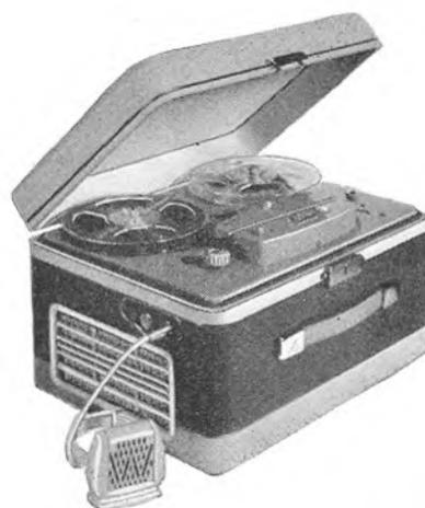
Those who possess a high fidelity amplifier and speaker system could undoubtedly use the recorder to good effect, as the frequency characteristic at the external amplifier output socket is substantially flat and not affected by the tone control.
