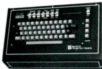
The slightly modified typewriter keyboard contains sixty-four characters including letters, numbers, and punctuations. Sixteen lines of copy, with thirty-two characters per line, can be typed and displayed on a television screen against a black background, or overlaid on another picture.
