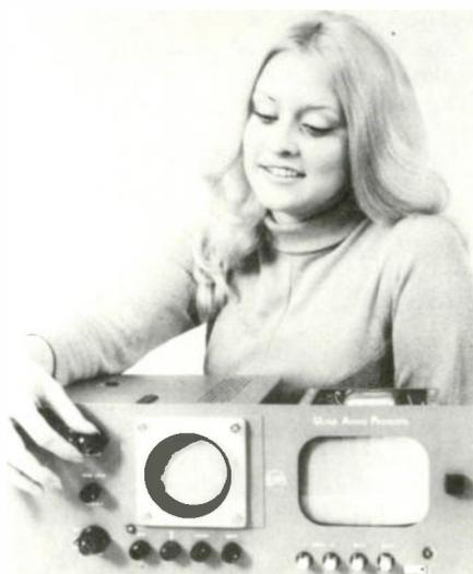
tion with a high-resolution 5" picture monitor. The assembly, WV-063, requires 7" of rack space and is designed primarily for placement of one such array on the output of each camera in a studio system, although it may be connected anywhere in the video circuit.
