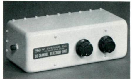
The unit, measuring 9" x 3" x 3 5/8", decreases co-channel interference by 20-30 dB. The single channel unit is priced at \$750.
