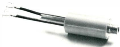
low-loss, completely shielded matching transformer which is used for connecting a 75-ohm coaxial tap line to the 300 ohm TV set input terminals. Mounts behind the TV set and comes supplied with male F-Type connector.
