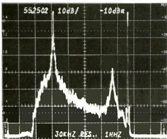
Figure 3: CATV head-end output.
