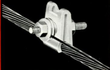
Permanent termination for lashing wire at the pole. Aluminum alloy plates fit and hold 1/4" strand. Hot dipped galvanized washers and nut hold lashing wire.
