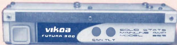
Model 265 Mainline Amplifier Module contains a four stage, push-pull broadband VHF amplifier circuit utilizing solid state active devices. Front panel controls include continuously variable Gain and Tilt potentiometers. A receptacle is provided for Vikoa's Expanded Range plug-in equalizer pads available in various db values.
