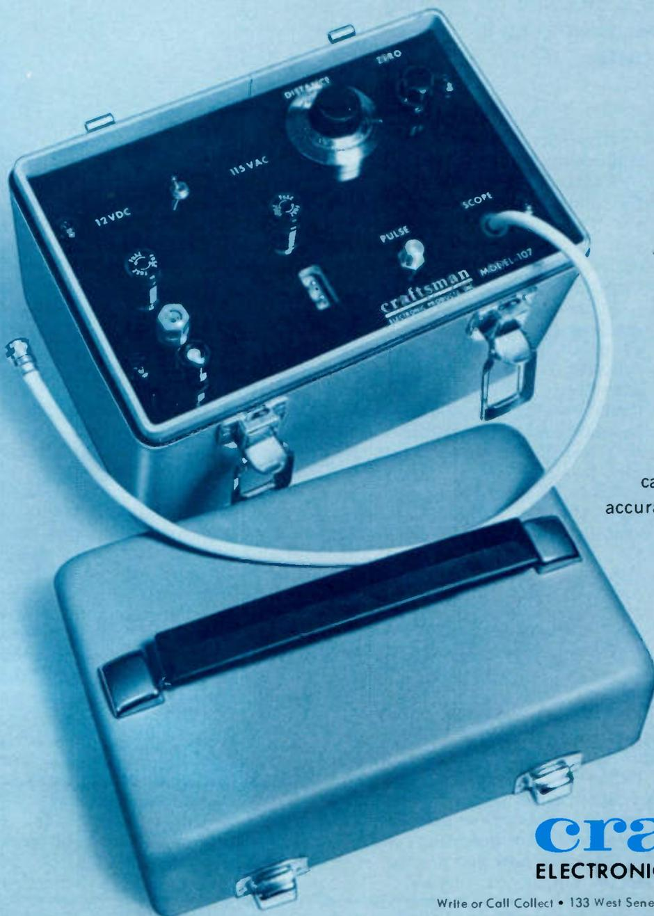
... with our new 107 Coaxial Cable Fault Finder - which fills one of CATV'S major needs: it's an accurate, portable and economical TDR (Time Domain Reflectometer). Sending a fast rise time pulse down the cable under test (up to 2500 ft. of .412) the return pulse pinpoints shorts, opens and both inductive or capacitive mismatch, all within  $\pm 2\%$  accuracy. You owe it to yourself and your system to talk with your Craftsman representative about it soon.
