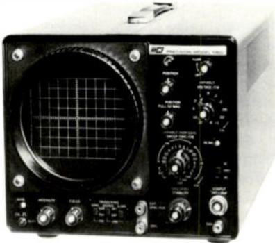
Patterns on the flat-face, high-sensitivity 5" screen are exceptionally bright. There's no "dot blooming" with the 1460; 1650 volts on the accelerating anode insure sharp patterns at fast writing speeds of up to 0.1 micro-second/cm (with x5 magnification). The only tube in the 1460 is the CRT, all
