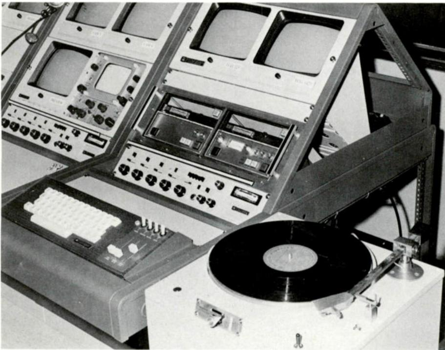
The audio portion of this CATV studio includes a professional turntable, two TAM-105 audio control units (just above the arm-rest portion of the console) and two audio cartridge tape units. (Photo courtesy TeleMation.)
