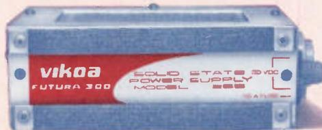
Model 266 DC Power Supply Module contains solid state switching regulator circuitry for maximum efficiency. Current-Guard design reduces dissipated power and heat. Output nominal 30 volts DC at up to 1.25 amperes. Test points and protective fuse are mounted externally for accessibility.
