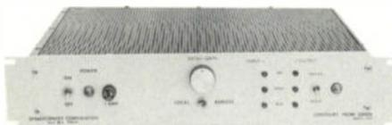
The scanning beam in a pickup tube has a finite size which tends to overlap adjacent picture elements. This results in the waveform having rounded rather than square corners. The Dynasciences enhancers are designed to correct for this, and thereby improve picture quality. All five enhancers are available in NTSC (525 lines) standards or PAL (625 lines) standards.
