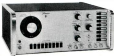
1 volt rms into 50 ohms. The VS-30 includes provisions for eight plug-in crystal controlled markers, a variable marker option and sweep rate controls from 60 Hz to 5 Hz plus manual sweep. The price of the unit is \$895.
