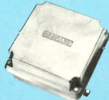
Weatherproof power supply housing of cast aluminum alloy for pole, cross-arm or underground installation. Clamshell design and silicon rubber sealing gasket provide complete sealing and radiation protection. Includes primary switch/breaker and AC convenience outlet. 12 x 12 x 7 $\frac{3}{4}$  inches. 17.5 lbs.
