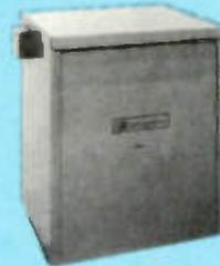
Weatherproof power supply housing of welded sheet aluminum. Supplied complete with externally-operated primary switch/circuit breaker, internal duplex receptacle and crossarm mounting bracket. 14 $\frac{1}{2}$  x 13 $\frac{1}{4}$  x 11 $\frac{1}{4}$  ins. 11 lbs.
