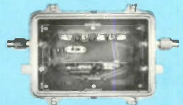
Cable-powered line extender in compact cast aluminum housing. Separate RF and power supply modules allow instant replacement. Features high output, low noise figure and wide control ranges. Bandwidth 50-220 MHz, ±.5db. Suggested operating levels are +40db mv out @ Channel 13.
