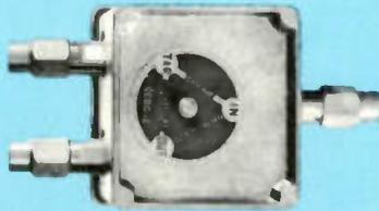
For insertion in trunk and feeder lines where an unequal split is needed, two models, CEDC-1/8 and CEDC-1/12 provide tap values of 8 and 12db,  $\pm 1$ db. Through-line insertion loss is 1.5 and 1db, respectively. Input, output and tap return loss is 20db over the 5-240 MHz bandwidth, and tap-to-tap isolation is a minimum of 18db. Circuit board may be positioned to use any of the three connectors as input, the other two becoming output and tap connections.
