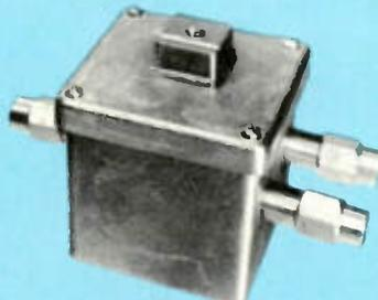
CELS is a passive line splitter, providing equal output to two trunk or feeder lines. Unique construction allows circuit board to be positioned to use any of the three connectors as input, and other two as outputs. Input and output return loss is 18db over 5-240 MHz range, and tap-to-tap isolation is 18db. Splitter loss is 3db at Ch. 2, and 3.5db at Ch. 13.
