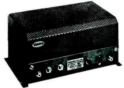
**All-band distribution amplifier, Model 940.** Separate low and high band gain controls. Low and high band tilt controls. Gain: 40 db (minimum). Covers all VHF channels plus FM. Output: 64 dbm (1.7v) total per band for less than 1% cross-modulation. Available with either F or UHF fittings at no extra cost. Add \$10.00 to price for 10,000 hour tubes. Price: \$65.00.
