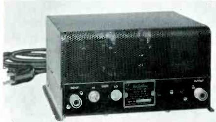
**Line amplifier, Model MLA-C.** Provides at least 40 db gain on all VHF channels. Separate gain controls for channels 7-13 and 2-6. Separate tilt controls. Maximum output (across 75 ohms) 2.0 volts per band for less than 1% cross-modulation. 3.5 volts per band for less than 3% cross-modulation. Net: \$94.85.
