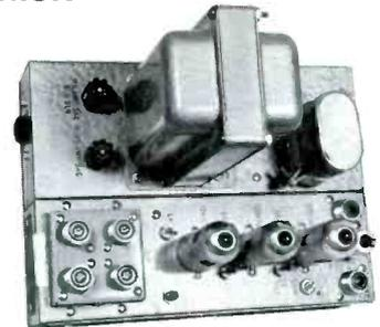
**Low band bridging amplifiers, Model BA-254 series.** Two inputs, four outputs, 50-88 mc. Gain: 20 db. Output, plus 42 db noncascaded; plus 37 db cascaded. 2 - 4 db noise figure. Gain control range 3 db variable. Attenuator plugs in 3 db steps. Built-in power supply. Available with or without regulated power supply. 75 ohm. Mounts any position. Price: \$99.50.
