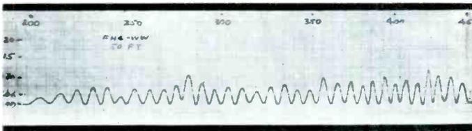
Fig. 4 VSWR measurements on length of 1/2" foam Heliac.
