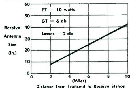
Since it would not be economical to provide all ranges of antenna sizes to logical selection would be to pick two sizes that represent a reasonable safety margin—for example: 4 feet and 2 feet.
