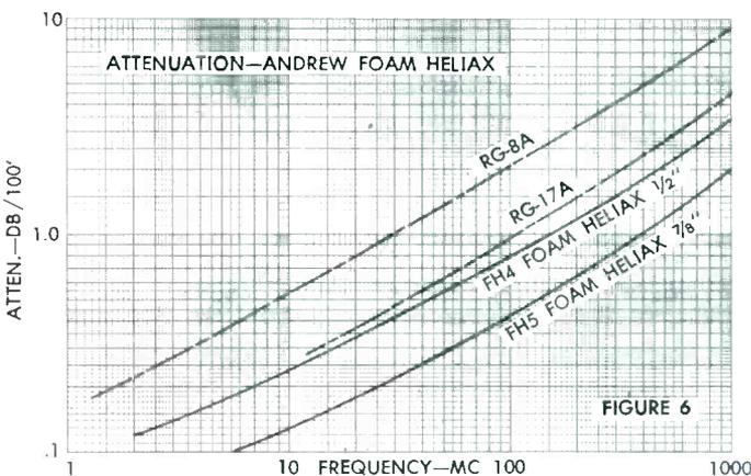
Fig. 6 Comparative attenuation curves for 1/2" and 7/8" foam Heliac.
