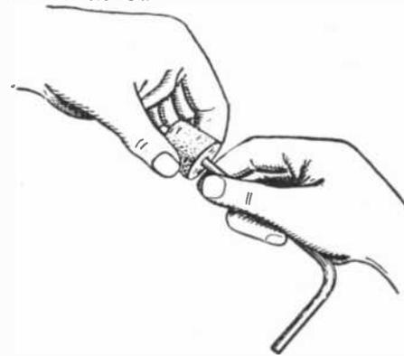
Inserting a bent tube in a cork; the same care is taken as in the preceding case, so that if the tube breaks it will not mutilate the hand. It is an excellent plan to wrap a towel around the tube while inserting it.
