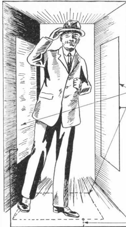
A very unusual entrance alarm may be constructed by the arrangement shown here. Large sheets of tin foil mounted on the walls of the entrance hall and connected to a grid circuit of an oscillating tube will leave the circuit unaffected, until some one alters the capacities between these sheets by stepping between them.
