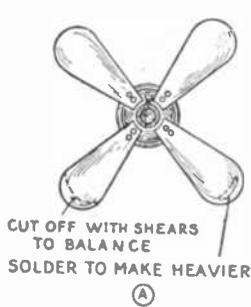
Electric fans frequently become noisy due to the fan blades being out of balance mechanically. In the present article details are given for balancing fan blades, as well as armatures, and the picture at the left shows how to lighten a blade by cutting off a circular strip on the outer edge; or to increase the weight of the blade with solder.
