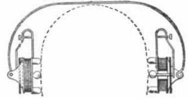
This is a head-set with very flexible diaphragms. Projections on the diaphragms press lightly against the temples. When a message comes over the telephone the pressure is varied, so that by the variations in pressure and by the duration of the periods of pressure, code can be received. Patent No. 1,531,543 issued to James J. Cooper, Atlanta, Ga.
