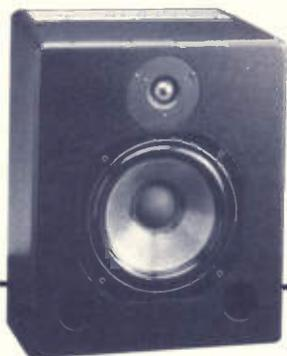
Q108 - 2 way active system with twin integral 100W power amplifiers and high quality BSS crossover network. 8" bass driver/1" soft dome ferrofluid cooled tweeter.
